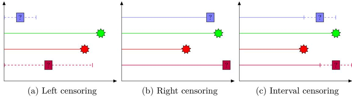
Fig. 2.1 Three types of censoring, left, right and interval. Stars represent an *observed* failure time. Intervals containing a question mark represent a period in which the failure is known to have occurred, but the exact time is *unknown* (censoring has occurred). In the case of right censoring, the event is known to occur beyond the question mark time. Colours represent different patients.
