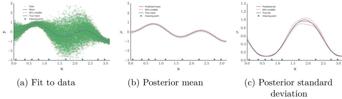
Fig. 4.7 Under a similar setting to Figure 4.6 the chained Gaussian process credible intervals collapse around the true values as the model becomes more certain in the presence of more data, particularly about the conditional standard deviation function
