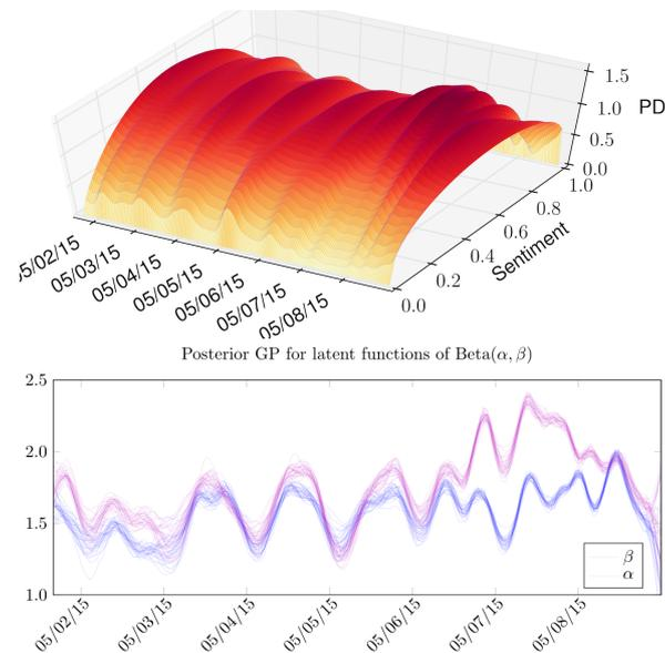
The latent functions  $\alpha$  and  $\beta$  that can be obtained from the model in Section 4.4.3 can be plotted themselves. If both latent functions went below 1.0 then the distribution at that time would turn into a bathtub shape. If both are larger than one but one is larger than the other, we have a skewed distribution. If one is below zero and the other above, it appears exponential or negative exponential.
