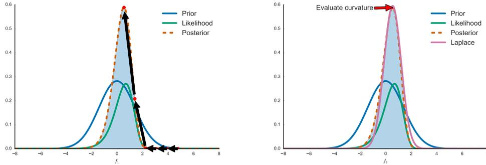
(a) Mode finding via Newton optimisation (b) Evaluate curvature at mode, use mode and curvature to approximate the posterior
