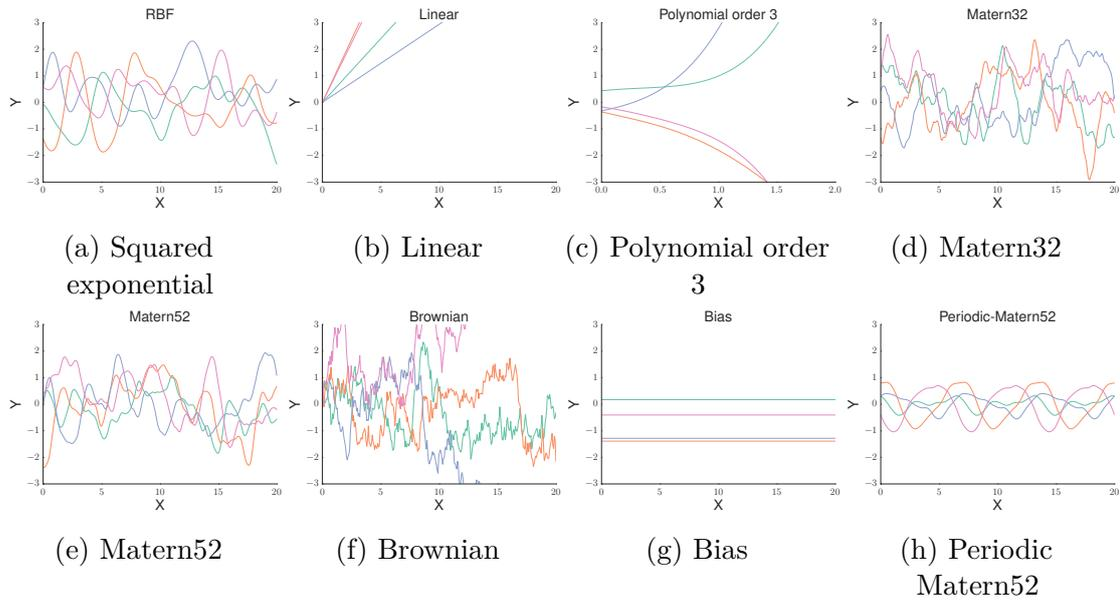
Fig. 3.3 Draws from zero mean GPs with a range of different kernel functions showing different assumptions about similarity between  $X$  locations. Equations for each kernel can be found in Appendix B or Section 3.1.1
