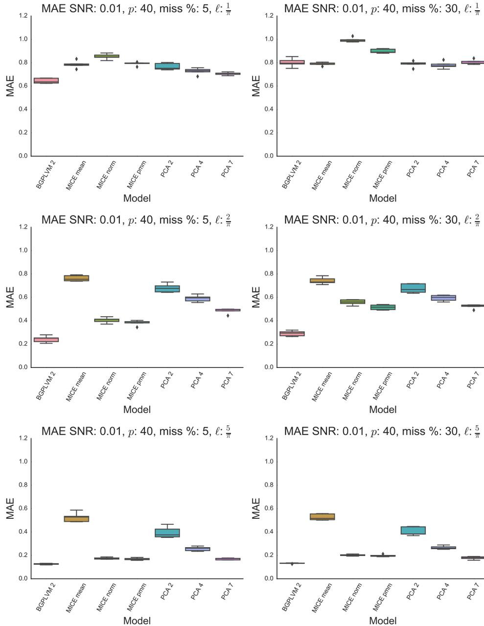
Fig. 5.3 Simulation study results for BGPLVM imputation model, with normally distributed observations.  $\ell = \frac{1}{\pi}$  indicates a very non-linear function,  $\ell = \frac{2}{\pi}$  indicates a relatively non-linear function, and  $\ell = \frac{5}{\pi}$  indicates an almost linear function. Missingness levels are varied between 5% and 30%.
