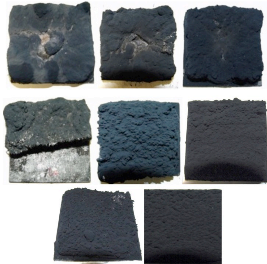
Figure 4.7. (Top left L-R) surface texture of char highlighting variation in pustule size and density for NTP separations of H/D = 20, 30, 40, 60, 80, 90, 100, 110 - CPF 1
