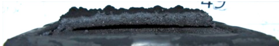
Figure 4.31(c). Cross sectional illustration of the char structure at the end of an experiment at NTP separation of H/D110 char pattern – HPF 2
