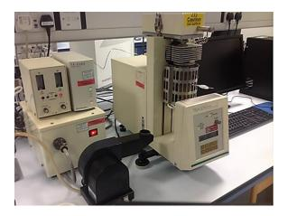
Figure 3-7 Thermo-gravimetric analyser (TGA) used for thermal and oxidative decomposition of oils
