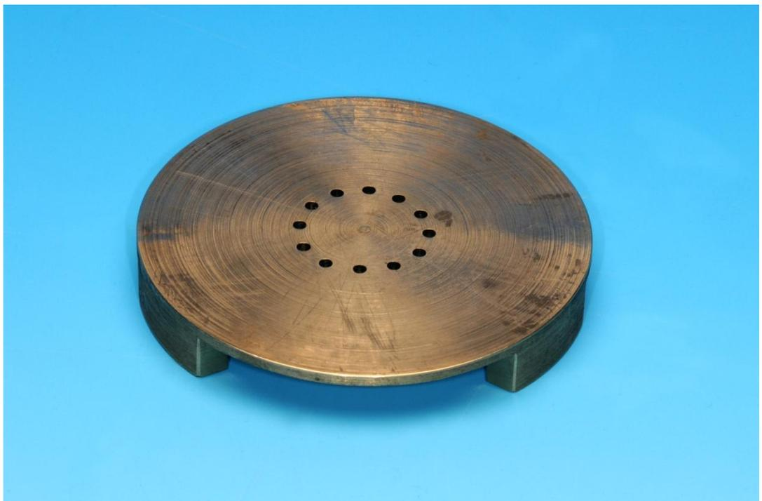
Figure 45 'impression tray' for the number of holes experiment
