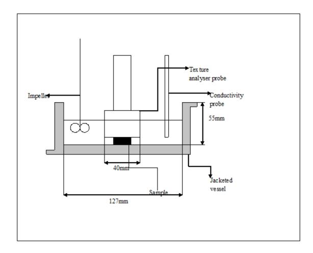
Figure 3.1 Vessel diagram for the experimental setup used in this study.
