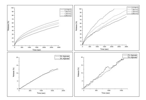
NaCl release over time into 200 ml of phosphate buffer from compressed 3 g cylinders of gels at room temperature (A), at 37  $^{\circ}$  C (B) (non-compressed) and room temperature (C), at 37  $^{\circ}$  C (D) (compressed). Gel compressed at constant rate of 2mm/s
