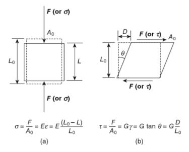
**Figure 2.7** Uniaxial compression (a) and shearing b) of a sample or product. Uniaxial compression of a sample with and original length  $L_0$  and area  $A_0$  and the Young's modulus *E*. (b) Shear stress  $\tau$  acting on opposite planes causing the distortion of the specimen with the shear modulus *G* and the area of  $A_0$ . Adapted from (Lu 2013).
