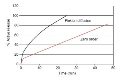
Figure 2.15 Schematic profile for zero order and Fickian diffusion model (Vasisht, 2014)
