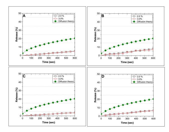
**Figure 5.3** Experimental release (%) over time (sec) for alginate gels for sodium chloride room temperature (A) and 37 °C (B) and compressed at room temperature (C) and 37 °C (D) plus theoretical release rates based on literature diffusion coefficients and viscosity.
