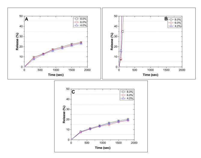
**Figure 4.14** Glucose release over time into 200 ml of phosphate buffer from compressed cylinders of gelatin gels at room temperature (A), at 37 °C (B) (non-compressed) and room temperature (C) compressed by constant amount (2mm).
