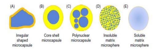
**Figure 2.19** Microcapsule (A, B and C) versus microsphere (D and E) morphology. (Vasisht, 2014)
