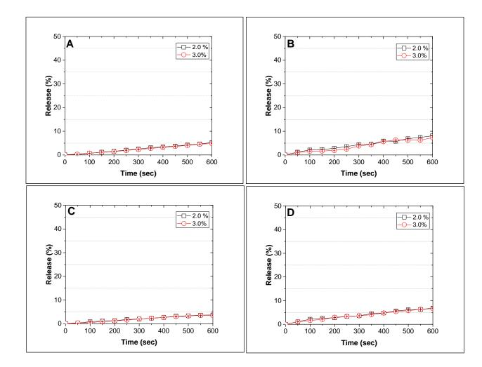
**Figure 4.10** NaCl release over time into 200 ml of phosphate buffer from compressed cylinders of alginate gels at room temperature (A), at 37 °C (B) (non-compressed) and room temperature (C), at 37 °C (D) compressed by constant amount (2mm).
