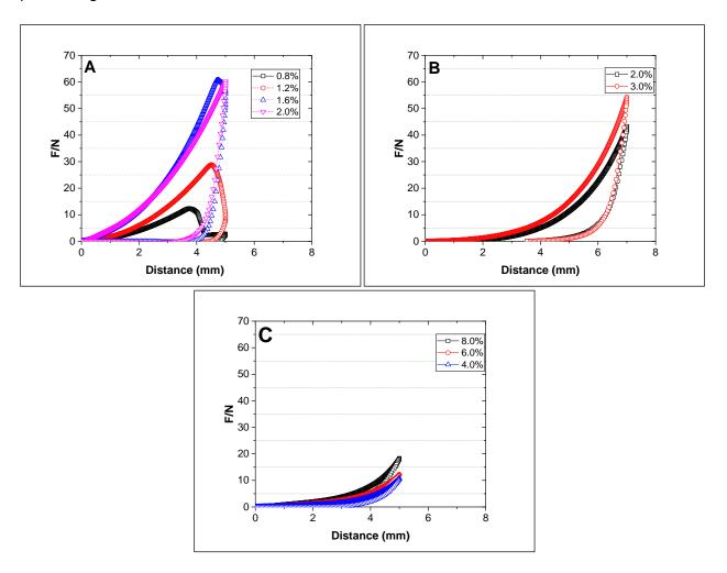
**Figure 4.1** Force (N) against distance (mm) curve for compression of cylinder with the addition for NaCl of  $\kappa$ -c (A), alginate (B) and gelatin (C) gels at different concentration. Tests were performed at a constant rate of 2mm/s to 5 mm distance compression. Alginate compressed at constant rate of 2mm/s to 7 mm distance.
