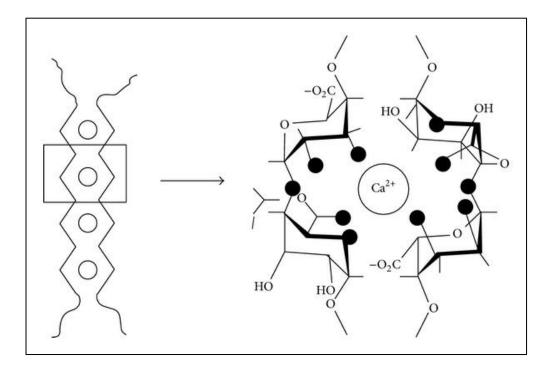
**Figure 2.3** Schematic drawing and calcium coordination of the "egg-box" model, as described for the pair of guluronate chains in calcium ALG junction ones. Dark circles represent the oxygen atoms involved in the coordination of the calcium ion. Reproduced from with the permission of the American Chemical Society (Sosnik, 2014).
