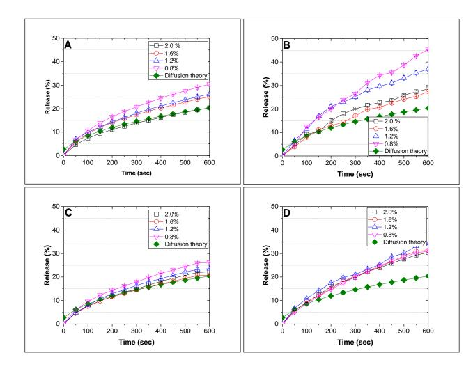
**Figure 5.2** Experimental release (%) over time (sec) for  $\kappa$ -carrageenan gels for sodium chloride room temperature (A) and 37 °C (B) and compressed at room temperature (C) and 37 °C (D) plus theoretical release rates based on literature diffusion coefficients and viscosity.
