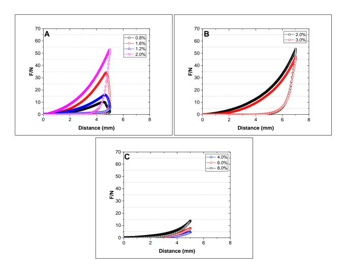
**Figure 4.2** Compression fracture force (N) against distance (mm) curve for compression of cylinder with the addition for glucose of  $\kappa$ -C (A), alginate (B) and gelatin (C) gels at different concentration. Tests were performed at a constant rate of 2mm/s to 5 mm distance compression. Alginate compressed at constant rate of 2mm/s to 7 mm distance.
