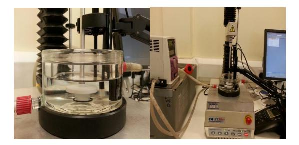
Figure 3.2 The actual experimental setups attached to the texture analyser.
