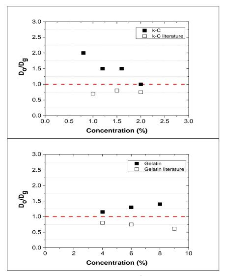
**Figure 5.8** Graphs showing comparisons of  $\frac{Do}{Dg}$ , Where ( $\Box$ ) obtained from study by Hendrickx et al., 1987) (**■**) is from the experimental data for glucose release.
