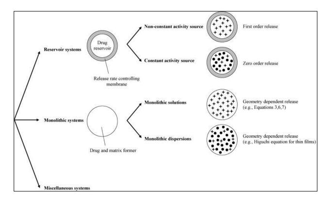
**Figure 2.20** Classification system for primary diffusion controlled drug delivery system. Stars represent individual drug molecules, black circles drug crystals and/or amorphous aggregates. Only spherical dosage forms are illustrated, but the classification system is applicable to any types of geometry taken from Siepmann and Siepmann 2008
