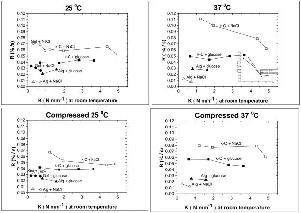
**Figure 4.16** R (%/s) over K (N mm<sup>-1</sup>) for all gels with the addition of sodium chloride and glucose room temperature.
