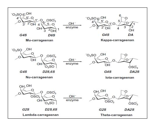
**Figure 2.1** Schematic representation of different structure of dimeric units of commercial carrageenan and related structure (Gulrez et al., 2003)
