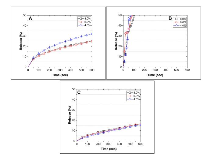
**Figure 4.11** NaCl release over time into 200 ml of phosphate buffer from compressed cylinders of gelatin gels at room temperature (A), at 37 °C (B) (non-compressed) and room temperature (C), at 37 °C (D) compressed by constant amount (2 mm).
