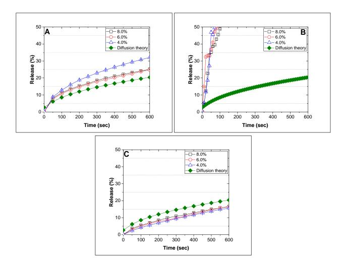
**Figure 5.4** Experimental release (%) over time (sec) for gelatin gels for sodium chloride room temperature (A) and 37 °C (B) and compressed at room temperature (C) and 37 °C (D) plus theoretical release rates based on literature diffusion coefficients and viscosity.
