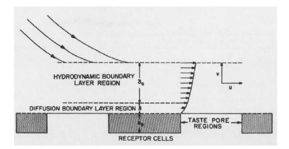
**Figure 2.18** Theoretical model of taste stimulus transport from a flowing source to the receptor cells within the taste pore. The diffusion boundary layer thickness varies with stimulus flow rate. The hydrodynamic boundary layer, the fluid velocity changes rapidly and is zero at the surface (Matsuo 2000)
