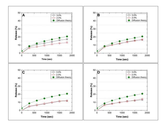
**Figure 5.6** Experimental release (%) over time (sec) for alginate gels for sodium chloride room temperature (A) and 37 °C (B) and compressed at room temperature (C) and 37 °C (D) plus theoretical release rates based on literature diffusion coefficients and viscosity.
