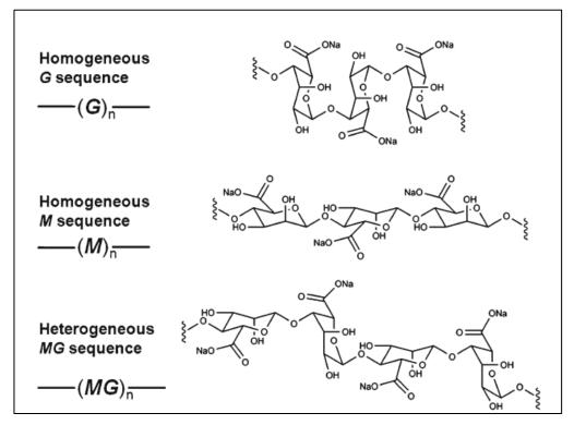
**Figure 2.2** Sodium alginate sequences (from top to bottom): homogeneous G sequence, homogeneous M sequence, and heterogeneous MG sequence. M mannuronic acid, G guluronic acid. (Fu et al., 2011)
