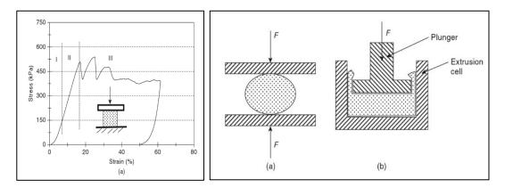
**Figure 2.8.** Example of Stress-strain (or *F-D*) curves of cylindrical apples tissue specimen under uniaxial compression. The stress-strain curves are approximately categorize into three phases of deformation: elastic, yielding and post yielding. Two types of compression test: (a) the uniaxial compression test between plates and (b) the simple compression-back extrusion test. Adapted from (Lu 2013)
