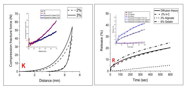
**Figure 4.15** Calculation gradient initial gradient for both release and compression fracture curves. Initial gradient for mechanical strength at distance 0.1-1 mm and the initial gradient for taste compound release from 0-100 seconds.
