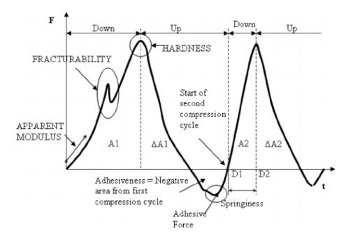
Figure 2.6 Force- time curve obtained from texture profile analysis (TPA) (Szczesniak 2002)
