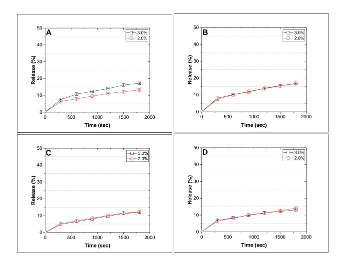
**Figure 4.13** Glucose release over time into 200 ml of phosphate buffer from compressed cylinders of alginate gels at room temperature (A), at 37 °C (B) (non-compressed) and room temperature (C), at 37 °C (D) compressed by constant amount (2mm).
