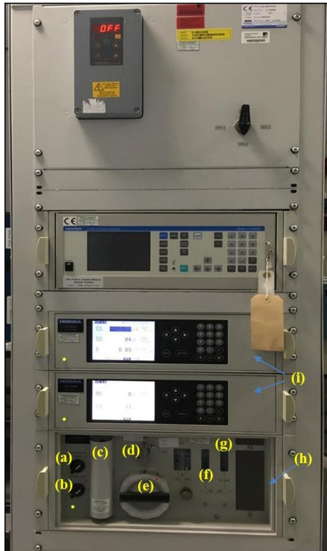
Figure 3.1-16. Horiba VS3000/VA3000 multi gas analyser; (a) Analyser pump,(b) Sample pump, (c) Mist catcher, (d) Selector valve, (e) Filter, (f) Sample flowmeter, (g) Calibration gas flow meter, (h) VS-3000 Gas sampling unit, (i) VA-3000 Multi – gas analyser unit.
