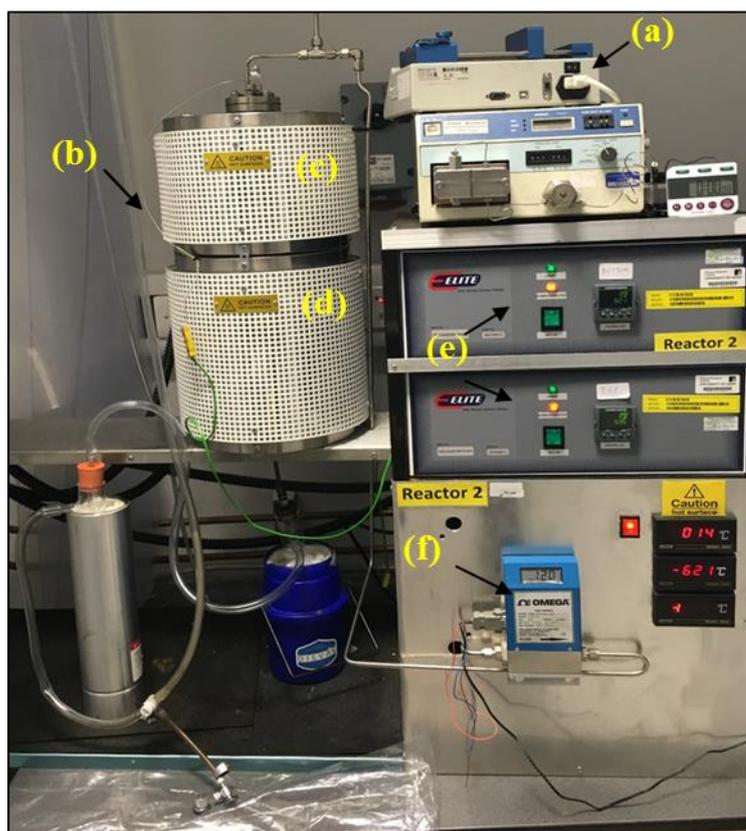
Figure 3.2-2. Assembled and main parts of the pyrolysis-gasification reactor; (a) Syringe pump, (b) Thermocouple, (c) 1<sup>st</sup> stage pyrolysis reactor, (d) 2<sup>nd</sup> stage catalytic reactor, (e) Furnace controller, and (f) Mass flow controller.
