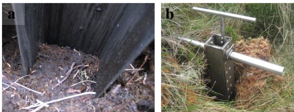
**Figure 5.3** a) Insertion of corer with three fixed sides into peat, surface was cleared of vegetation and compression was minimal. b) Corer with fourth side in place prior to core extraction.
