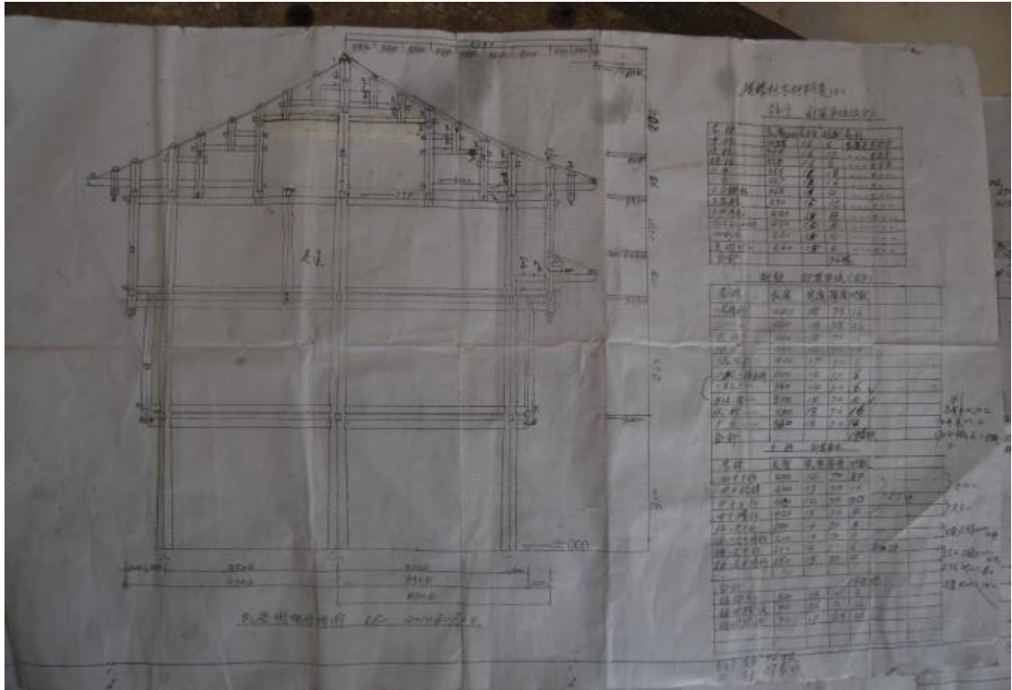
Figure 4. Drawing of hand-ink master Wenli Lu's new house with list of components at side, 2010. Drawing by Wenli Lu, photograph by Derong Kong.
