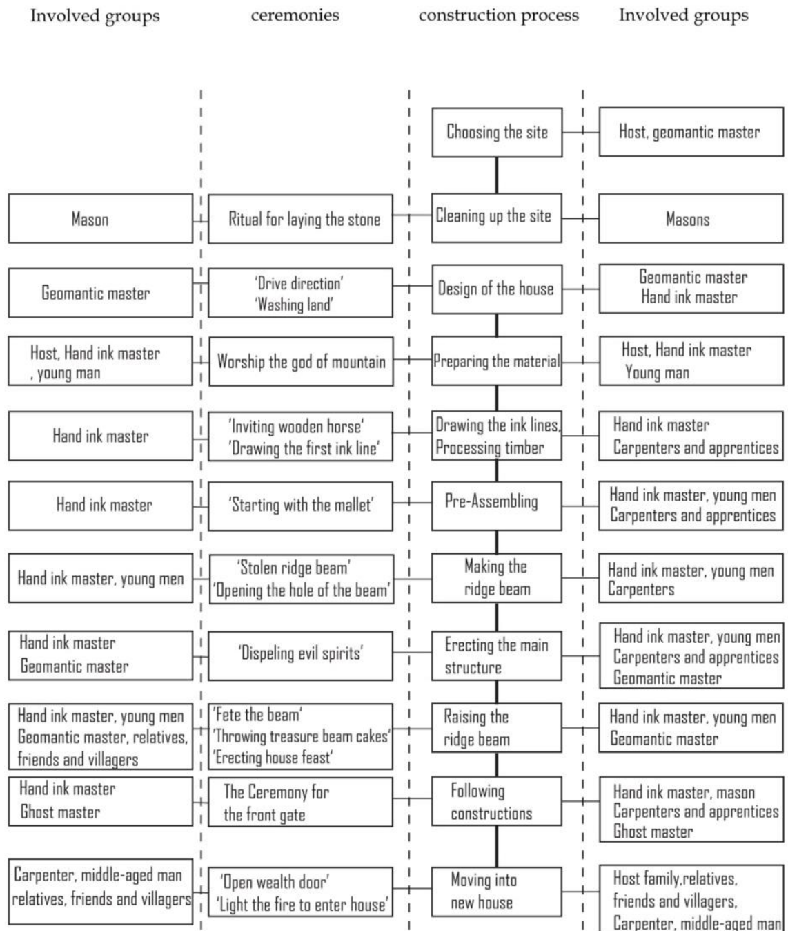
Figure 2. The construction process of the Dong house. Drawing by Derong Kong.
