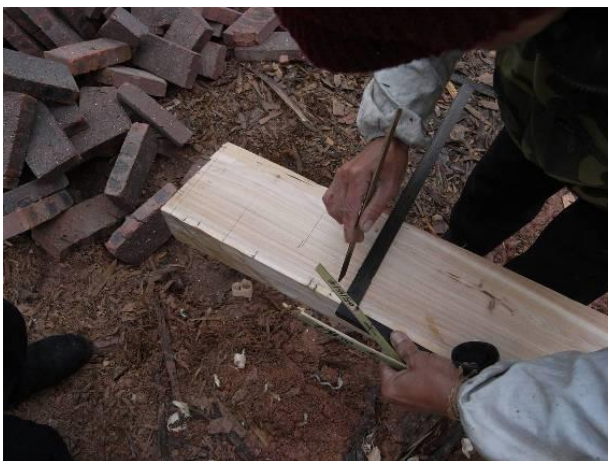
Figure 14. The hand-ink master Wenli Lu draws ink lines on draft wooden components. Photograph by Derong Kong.
