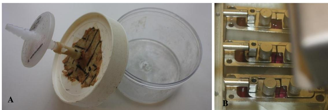
**Figure 5.15 Static incubation in the TenCell culture wells.** Samples incubated for 24 h at 37<sup>0</sup>C, 5 % (v/v) CO<sub>2</sub> in air, transferred to: (A) a culture tub (Nalgene) and placed in a standard incubator, (B) TenCell culture wells and placed in the TenCell-1 bioreactor.
