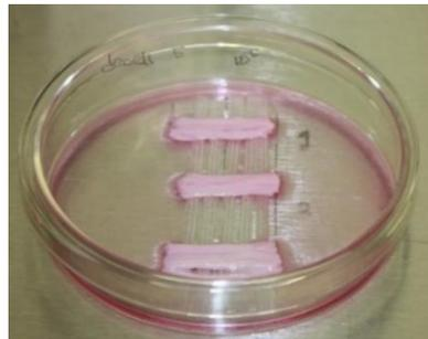
**Figure 5.18** Preparation of decellularised PPT scaffolds at the appropriate size ( $20 \times 10 \times 0.6 - 0.8 \text{ mm}^3$ ) in the preconditioning plate.
