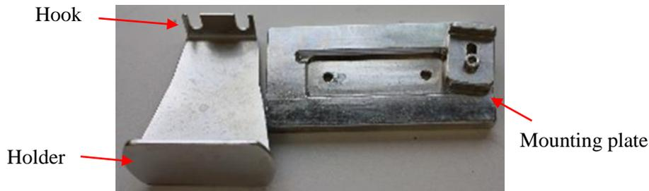
**Figure 5.4 A hook to move the inserts and a mounting plate to place the inserts.**
