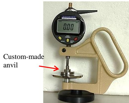
**Figure 5.7** The thickness gauge (J-40-V Schmidt)
