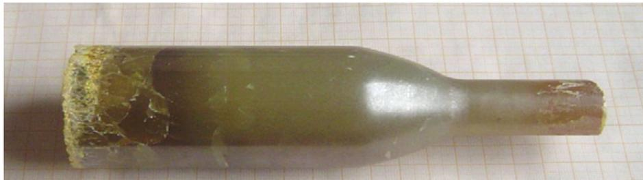
FIGURE 3.9: 25PIN-44PMN-31PT single crystal, 55 mm diameter and 100 mm length grown from a (110) oriented seed. From [65].
