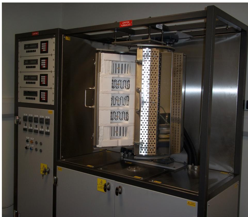
FIGURE 5.1: Crystal growth furnace at The University of Leeds. The five zone tube furnace is located on the right hand side, whilst the controls for translation/rotation movement together with temperature controls for each of the five zones of the furnace are located on the left hand side.
