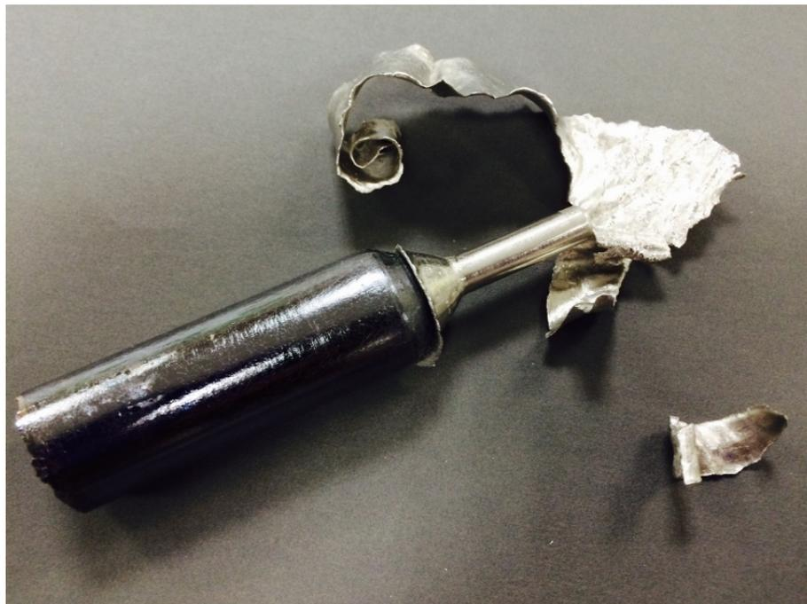
FIGURE 5.29: Single crystal grown during the fourth experimental run, B4 during removal from the platinum crucible
