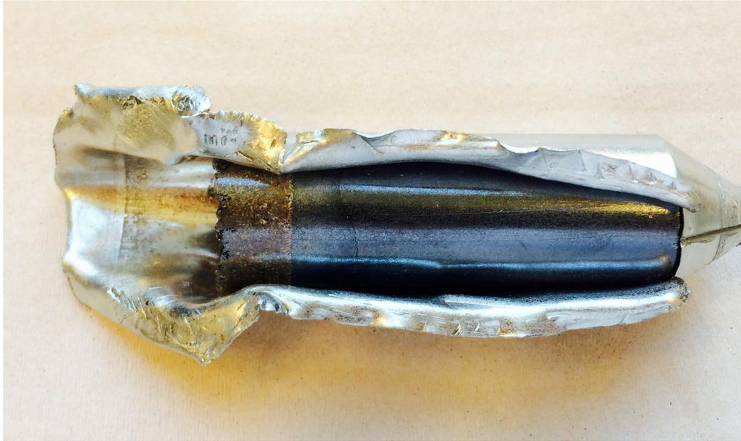
FIGURE 5.26: Single crystal boule grown during the third run, B3, as it is being removed from the platinum crucible
