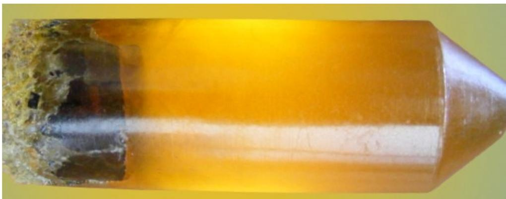
FIGURE 5.11: Crystal grown during the first run, i.e. unseeded growth as seen under a flashlight
