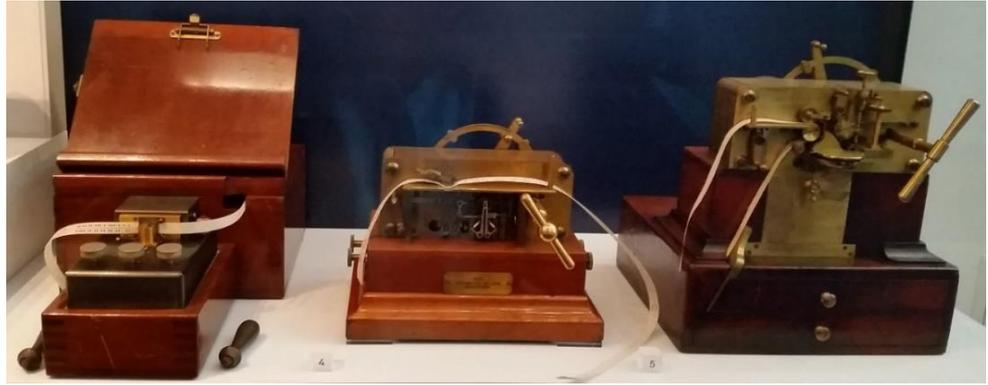
**Figure 5.3. Picture of a Wheatstone Automatic Instrument. It consisted of three distinct devices: the perforator with the dispenser of paper behind it (left), the transmitter (centre) and the receiver (right). Photograph taken at the Porthcurno Telegraph Museum in Cornwall and reproduced here with their kind permission.**
