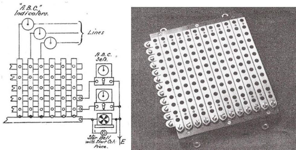
Figure 6.4. The universal switching capability of the Umschalter can be seen here (left) under one possible configuration of the switch (Source: diagram extracted from T.F. Purves, Figure 3). The picture on the right is an actual twelve-line Umschalter dating from 1880 (Source: BT Archives)
