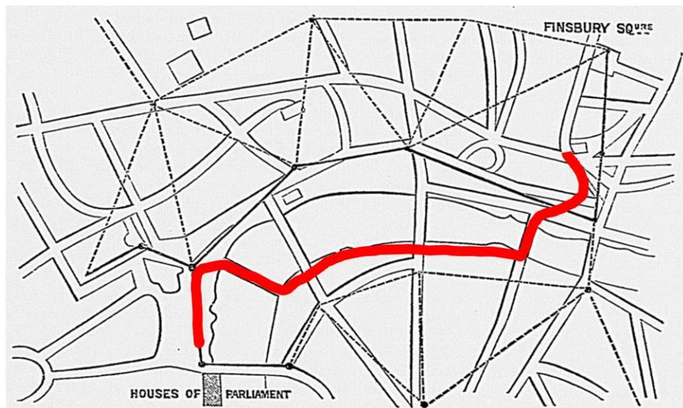
Figure 4.2. Waterlow's private network (1857) from London Wall to Parliament Street, via the Southwark and Hungerford bridges: an approximate path (thick red line) has been overlaid on a map of London published in an article titled 'The nervous system of the metropolis' on 2 March 1861 in the magazine *Once A Week*. The other plain and dotted lines represent the intended route of the future UPTC network (see Figure 4.5.).
