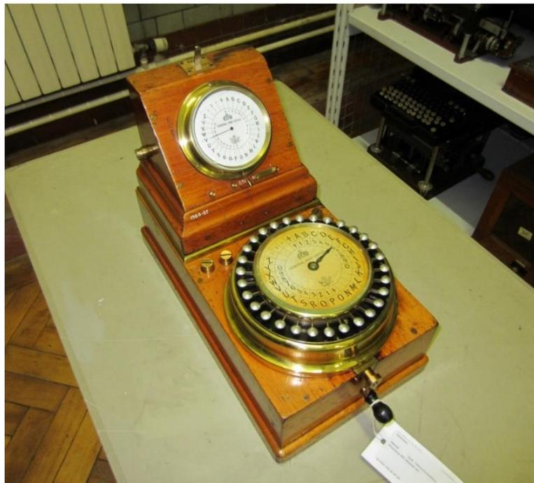
**Figure A 4.4. ABC instrument, 1860 specification. This instrument is stamped GPO but is likely to be one designed according to the 1860 specification. Photographed at Blythe House in September 2013, and reproduced with the kind permission of the Science Museum.**
