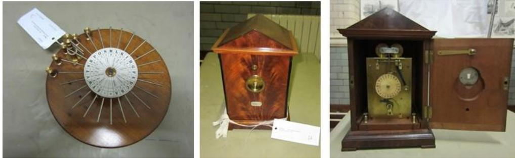
Figure 4.1. Charles Wheatstone's original 1840 dial instrument (Patent No. 8345), based on the step-by-step technology: the 'Communicator' on the left, and the 'Indicator' on the right (battery not shown). See Appendix 4 for a full history of the step-by-step technology and the ABC instrument. Photographed at Blythe House in September 2013, and reproduced with the kind permission of the Science Museum London.
