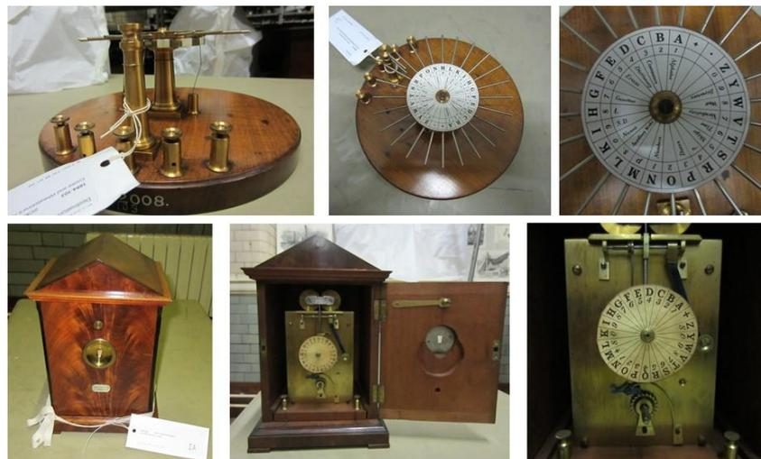
**Figure A 4.2. ABC instrument, 1840 specification. The device in the top row is the communicator (battery-operated). The bottom row shows a receiver that uses the alternative circular dial presenting the symbols in a small aperture. Photographed at Blythe House in September 2013, and reproduced with the kind permission of the Science Museum.**
