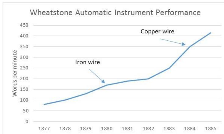
**Figure 5.4. The use of copper wires on aerial lines significantly improved the speed of telegraphic transmission.<sup>426</sup>**
