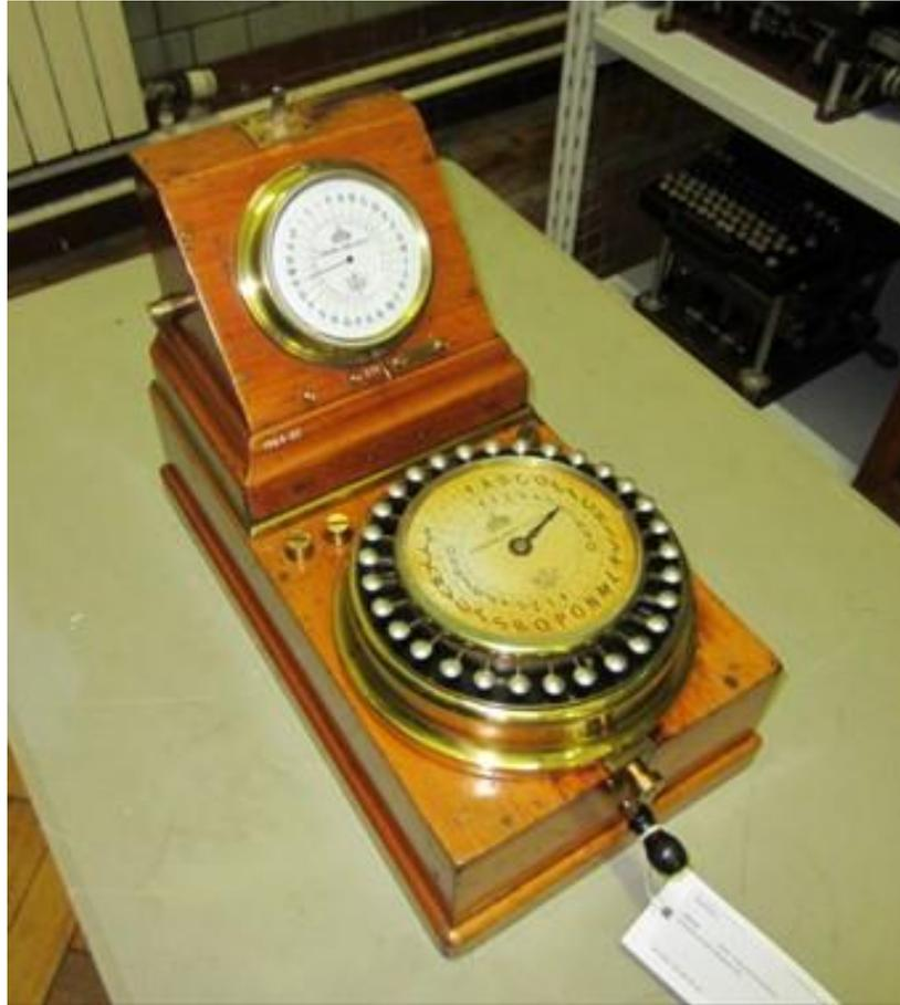
**Figure 4.4. Charles Wheatstone's ABC instrument, based on the 1860 specification (Patent No. 2462) and further improved (c. 1865) by combining the Communicator and Indicator into a single instrument, together with a magneto-electric generator to avoid battery operation. This instrument is stamped GPO. Photographed at Blythe House in September 2013, and reproduced with the kind permission of the Science Museum.<sup>319</sup>**
