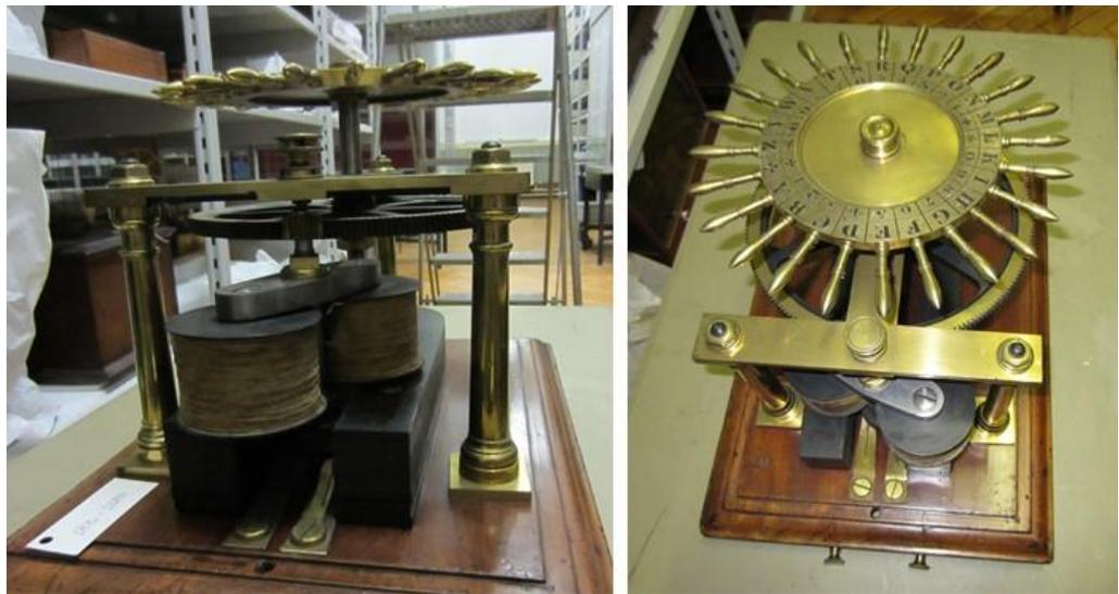
**Figure A 4.3. Magneto-Electric ABC Instrument, 1840 specification. Photographed at Blythe House in September 2013, and reproduced with the kind permission of the Science Museum.**
