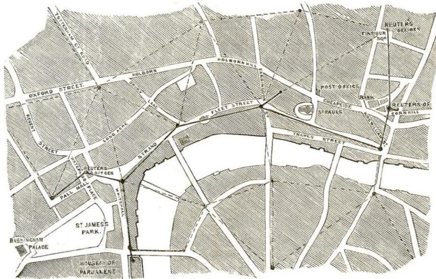
**Figure 4.5. UPTC metropolitan network in 1861. The dashed lines are presumably the planned routes. The triangulation technique described in the 1860 specification can clearly be seen in this representation, but at this early stage of development the trunk line infrastructure was mostly linear.<sup>331</sup>**
