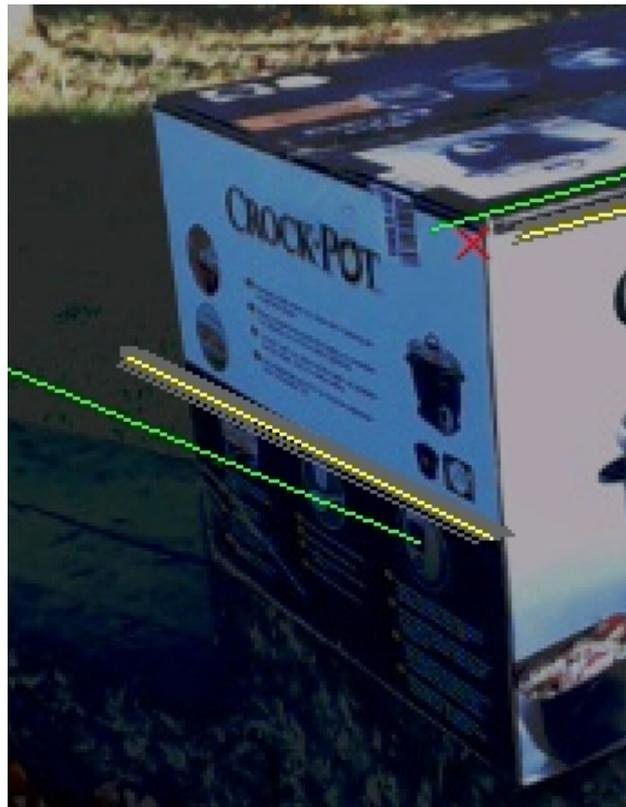
**Figure 5.16:** Scattered particles. One of the properties of particle filtering is that when no hypothesis has more votes than another, the newly resampled particles present scattering (Grey lines covered by the yellow line). This allows more resilience to erratic motion, since the scattered particles cover a wider area allowing to retrieve the object's edge gradient observation. Once a hypothesis with high weight is found, the particles quickly pile up towards the most weighted one.
