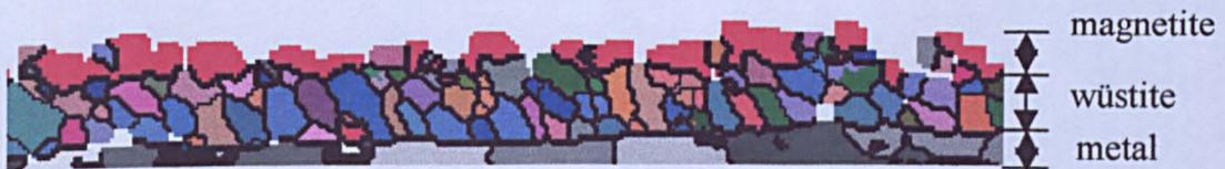
( c ) EBSD map of the scale on K08 rod surface (LT890°C), sample was supplied by Scunthorpe Rod Mill (scale thickness is 13µm)
