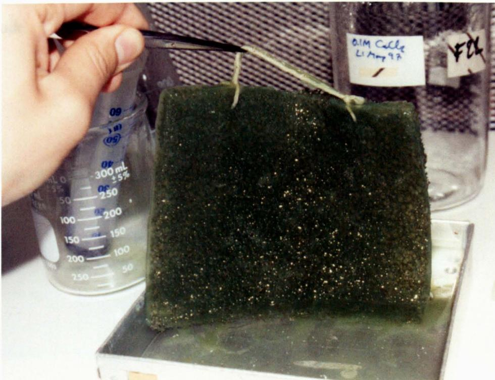
**Figure 2.3:** Immobilised algae in calcium alginate with spongy sheet supporter (algal sheet). Top picture shows pouring algal and alginate mixture on spongy sheet and picture below shows “algal sheet” after it has solidified.
