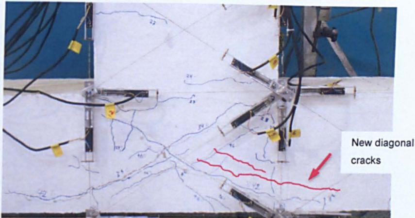
**Figure 4.33: Specimen JC-1 after three cycles at 1.5% drift**
