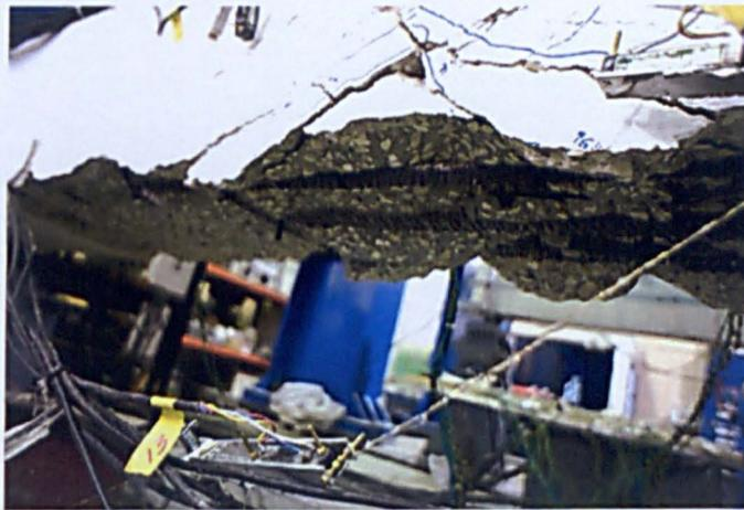
**Figure 4.38: Exposed rebar in specimen JC-1 after 4.0% drift cycles**
