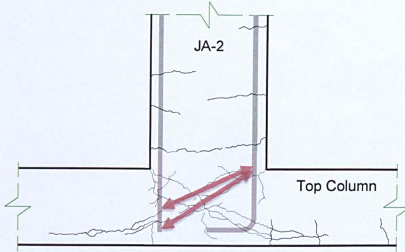
Figure 5.8: Crack pattern of JA-2 showing an extended compression strut
