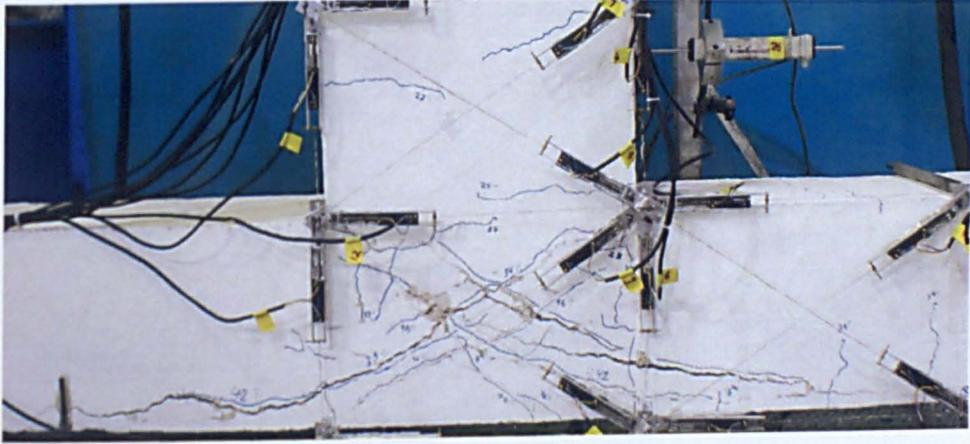
**Figure 4.35: Specimen JC-1 after three cycles at 3.0% drift**
