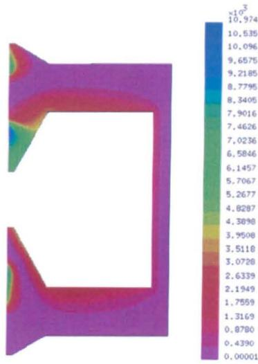
Fig. 5.31 Eddy current density distribution in SMC stator at 50 Hz with armature position at 5.0 mm
