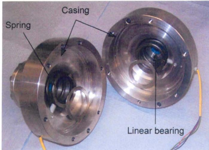
Fig. 6.2 Motor casing
