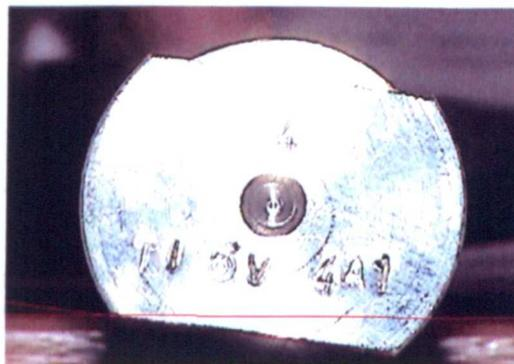
*Figure 5.26 Sample after failed forward-reverse torsion showing  $\sim 8^\circ$  permanent twist (table top used as datum reference)*
