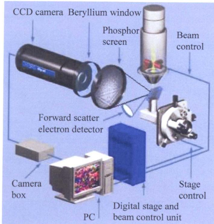
Figure 2.24 EBSD detection equipment arrangement [62]
