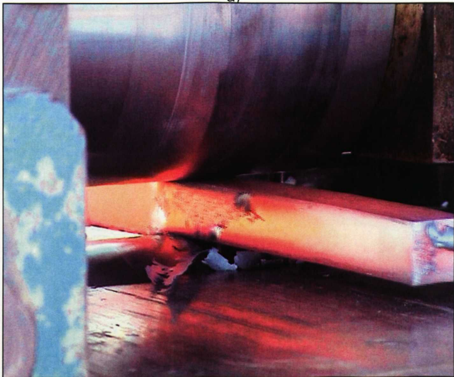
Figure 6.23 – Effect of the different rolling passes on the scale layer removal for sample 03-11b; where a) is looking at the roll bite entry for the descale pass (10% reduction), and b) is the looking at the roll bite exit for the principal rolling pass (20% reduction).
