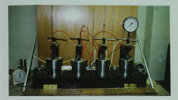
Figure 6-2 A general view of "The Leeds Permeability Cells"
