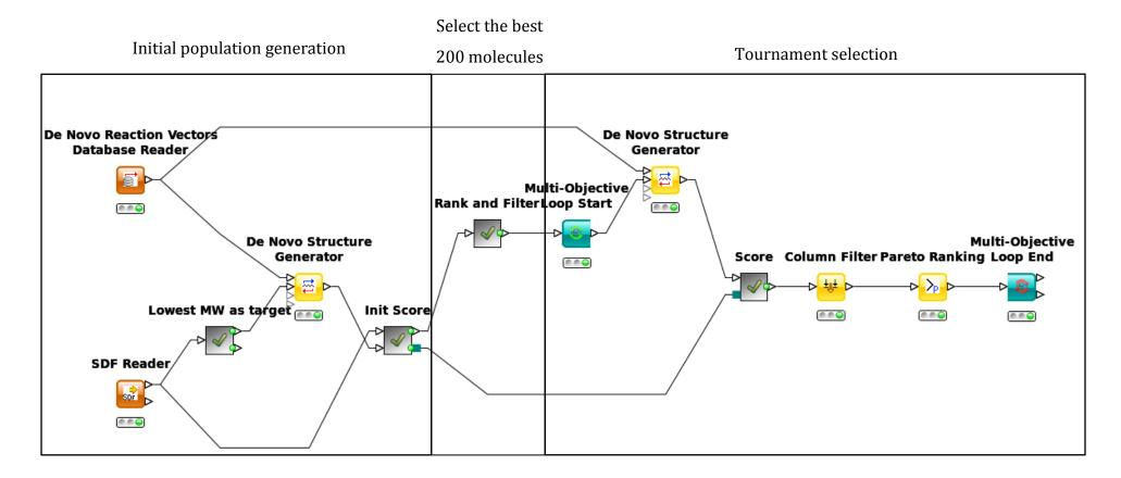
Figure 8.12: KNIME workflow for the tournament selection process.
