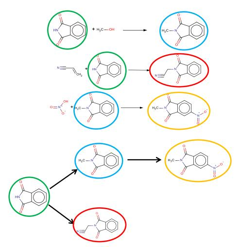
Figure 5.6: Example of network construction for three reactions from the database. Only one reactant and one product are considered for each reaction (circled, top) to be collated into the network based on their relative roles (bottom). (Wallace, 2015)
