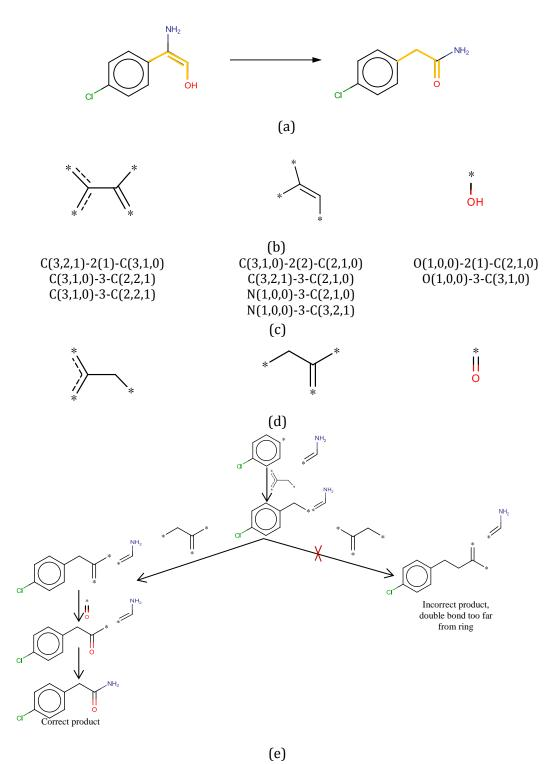
Figure 4.2: The structure generation procedure using the reaction vector method. (a) The reaction in question (affected bonds in orange). (b) The bonds to be removed from the reactant to form the fragment (\* indicates attachment point). (c) The negative AP2 and AP3 descriptors (the 'negative' pairs from Figure 4.1). (d) An unordered set of bonds to be added to the fragment to form the product. (e) The structure generation procedure – fragments are assembled bond-by-bond. (Wallace, 2015)
