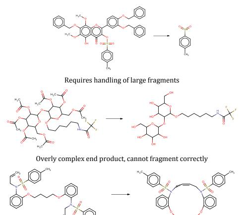
Figure 6.9: Examples of reactions that fail using the *de novo* algorithm, with the reasons for failure. (Wallace, 2015)
