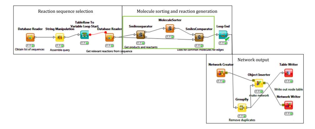
Figure 5.5: KNIME workflow showing the generation of the reaction network.
