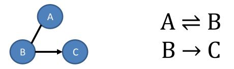
Figure 2.12: Example of a reaction graph (left) for a simple reaction sequence (right).
