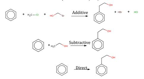
Figure 6.3: Examples of the different methods of generating reaction sequence vectors from a typical two step reaction sequence. (Wallace, 2015)
