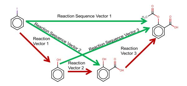
Figure 6.2: Comparison of the reaction vector (RV) and reaction sequence vector (RSV) based approaches to structure generation. The RSV method aims to enable direct transformation from start to end point of the sequence, without having to generate each individual reaction in turn. (Wallace, 2015)
