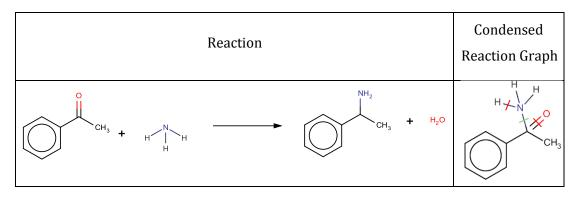
Figure 2.7: Illustration of the condensed reaction graph approach for the Mignonac amination reaction. (Wang, 2010, Wallace, 2015)
