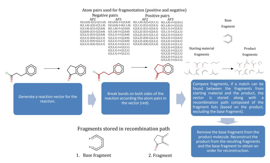
Figure 4.3: Flowchart showing the reverse fragmentation process. Note that all the acyclic atoms are 'lost' as they become part of a ring in the product. On recombination, the ring fragment (labelled 2 above) is stored as the recombination path (Wallace, 2015)
