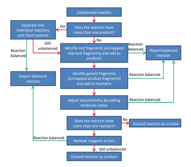
Figure 4.8: Summary of the reaction cleaning algorithm. At each step, the carbon count is rechecked, with the algorithm stopped if the reaction is balanced (green route). If not, the algorithm continues (red route).
