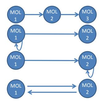
Figure 2.13: The reaction graphs for a two step reaction sequence, including loops where a loop represents a rearrangement. The four graphs represent: a simple two step progression; a rearrangement of molecule 1 followed by a reaction to molecule 2; a reaction to molecule 2 followed by a rearrangement; and a dynamic equilibrium. With comparison to the observed behaviour of the reaction system, logical conclusions can be drawn as to which of these mechanisms are valid, facilitating assignment.
