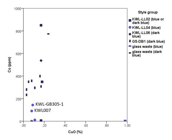
Figure 9.10: The CuO-Co bi-plot of blue and dark blue v-Na-Ca glass.
