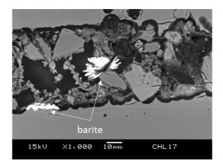
Figure 8.22: The inclusions of barite in JXL17.
