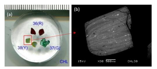
Figure 9.16: (a) The yellowish outer area and greenish inner area in JXL38; (b) the BSE image shows compositional differences in the two areas.
