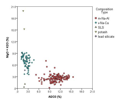
Figure 8.1:  $Al_2O_3$ -( $MgO+K_2O$ ) bi-plot showing the chemical groups of beads from Kiwulan, Shisanhang, Jiuxianglan, Guishan, Wujiancuo, Daoye and Xiliao (base compositions).
