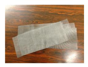
**Figure 3. 20** The photograph of rectangular cuts of the stainless steel screen of the regenerator
