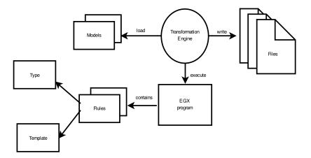
FIGURE 2.10: Overview of transformation execution using EGX.
