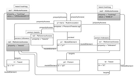
FIGURE 5.3: Expansion of the property access trace for the *p1-trans* rule invocation.
