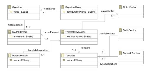
FIGURE 4.2: Extended Module invocation in EGL.
