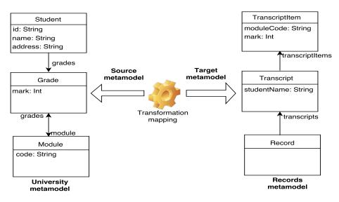
FIGURE 2.5: Example of a Model-to-Model Transformation
