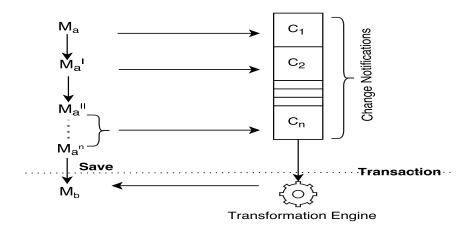
FIGURE 5.5: Overview of user-driven transaction boundary in online transformation mode.
