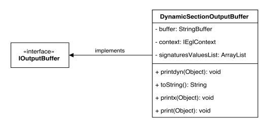
FIGURE 4.3: Extended OutputBuffer for Automatic Signatures.
