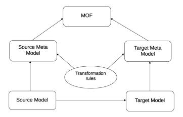
FIGURE 2.6: Overview of Model Transformation Process taken from [3]
