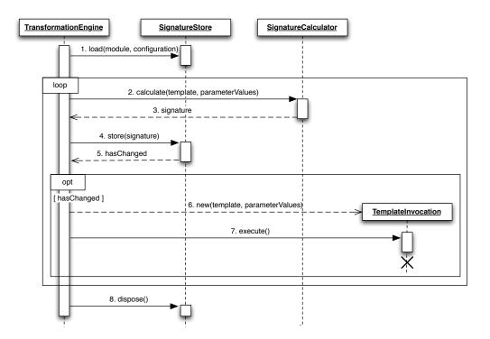
FIGURE 4.1: UML sequence diagram describing how Signatures are used to determine whether or not a TemplateInvocation should be executed.
