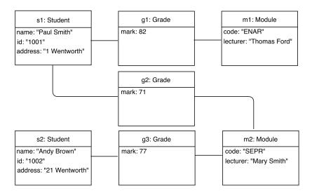
FIGURE 2.11: Example of University model that conforms to metamodel in Figure 2.1
