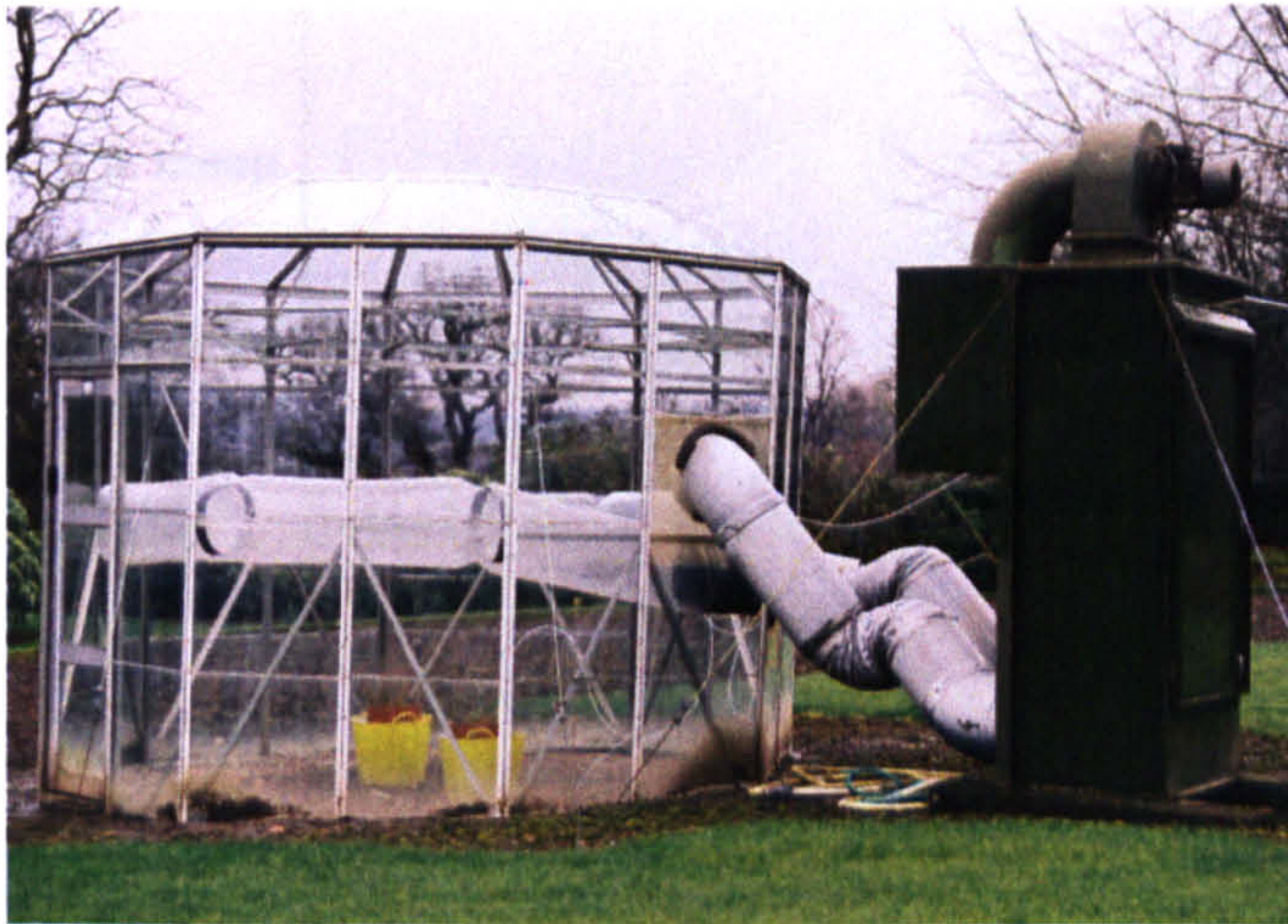
Figure 75: Lowland mire mesocosms placed in open top chambers at the field station Close House, New Castle (Source: Dr. Toet).
