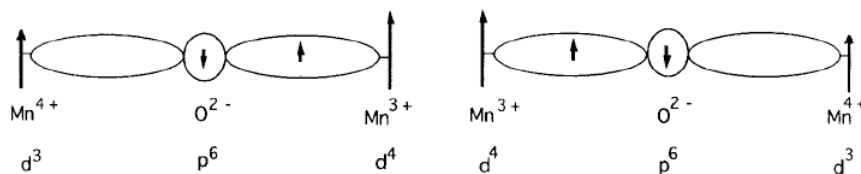
Figure 2.6: Schematic diagram of the double-exchange mechanism. The two states \text{Mn}^{3+} - \text{Mn}^{4+} and \text{Mn}^{4+} - \text{Mn}^{3+} are degenerate if the manganese spins are parallel. From (1).
