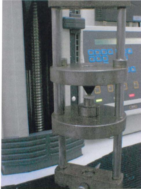
Figure 8.6: Ball on ring arrangement in a Lloyds LRX tensometer used for biaxial flexural strength test.
