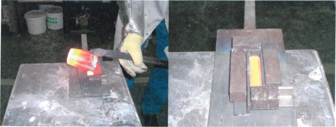
Figure 8.8: Re-melting of the glass pieces and the mould it was cast in.
