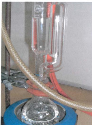
Figure 8.1: S57 glass discs within the extraction apparatus.
