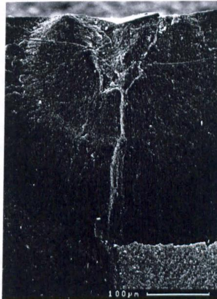
Figure 3.13 Radial/median crack formed during Vickers indentation
