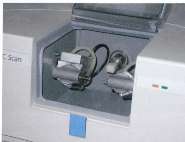
Figure 8.10: The CEREC-Scan hardware with an S80 block inserted.
