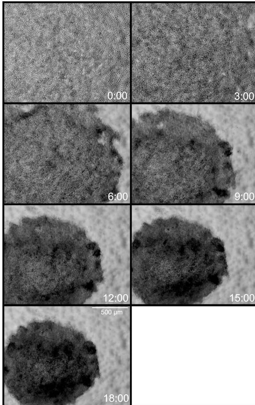
**Figure 4.4.6 – Time-lapse of MSC-EC spheroid formation using a light microscope**
