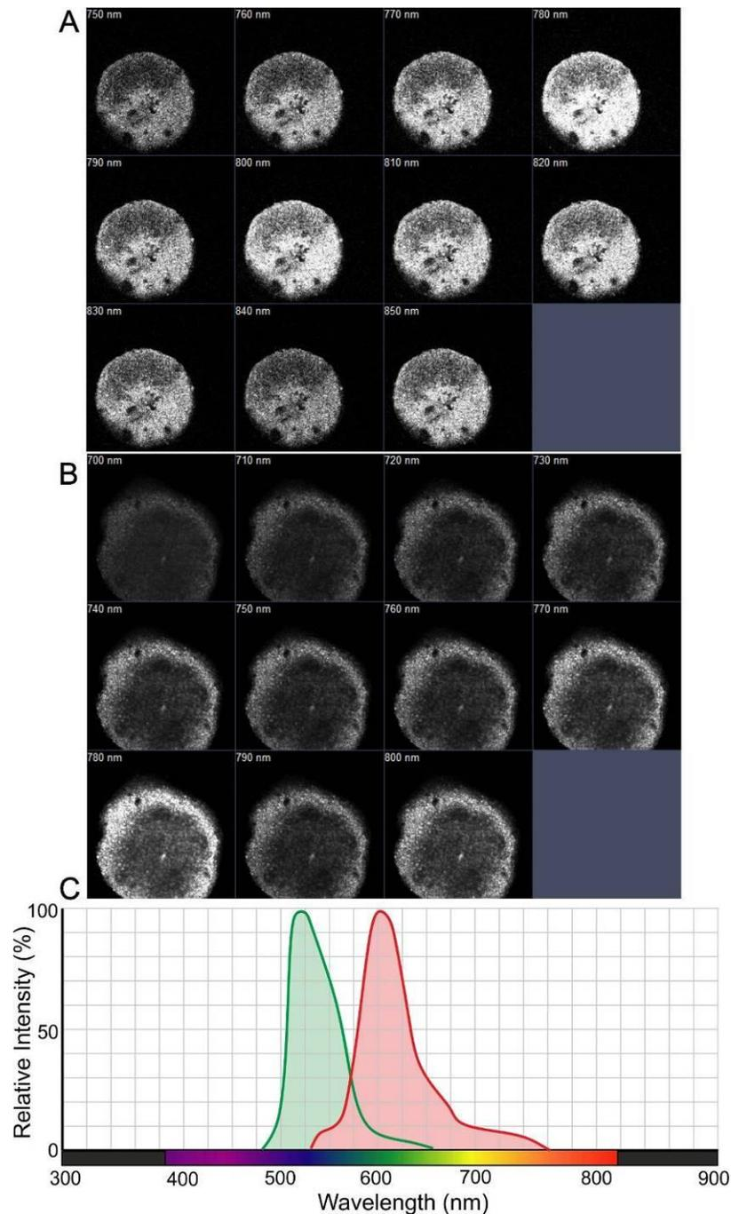
**Figure 4.4.1 – Laser optimisation and spectral analysis using CellTracker™ Green and Red**
