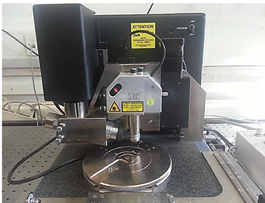
Figure 4.20: Veeco-Dimension 3100 AFM device at the University of Sheffield
