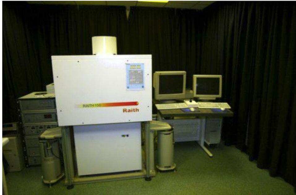
Figure 4.2: EBL system at the Centre for Nanoscience and Technology University of Sheffield
