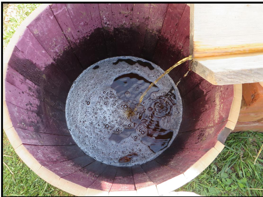
Figure 6: lixivium of four settling tubs draining via the trough
