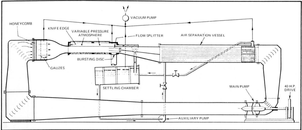
Figure 5.1a – Schematic Diagram of the Variable Pressure Recirculating Water Channel. From Hunter et al.<sup>5.5</sup>
