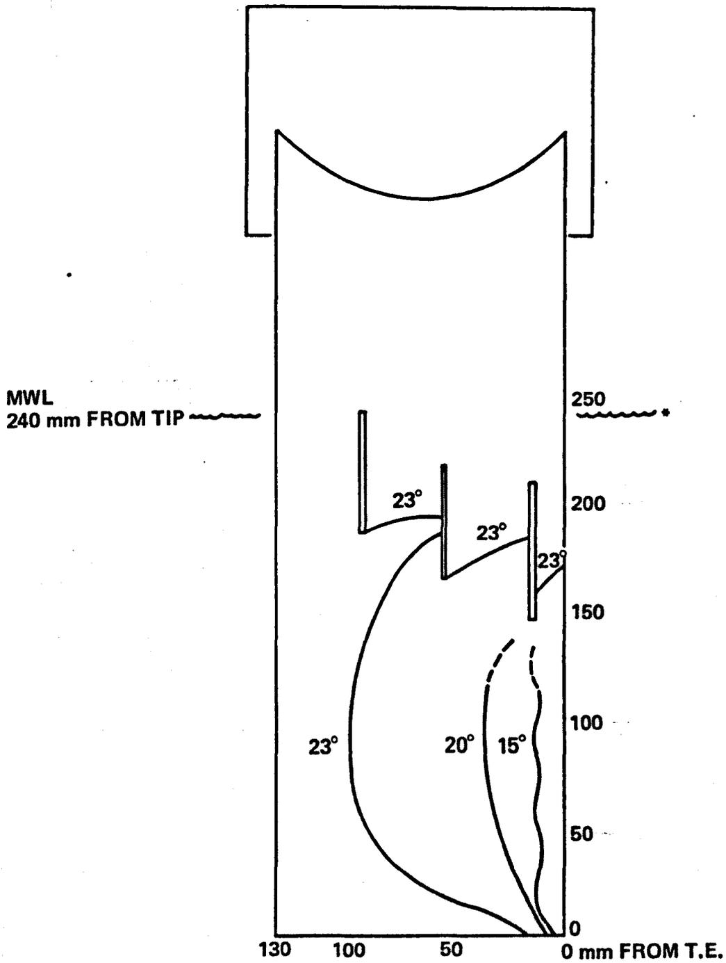
Figure 9.18 – Development of Separation on NACA 16 021 Strut, Configuration P7\*,
