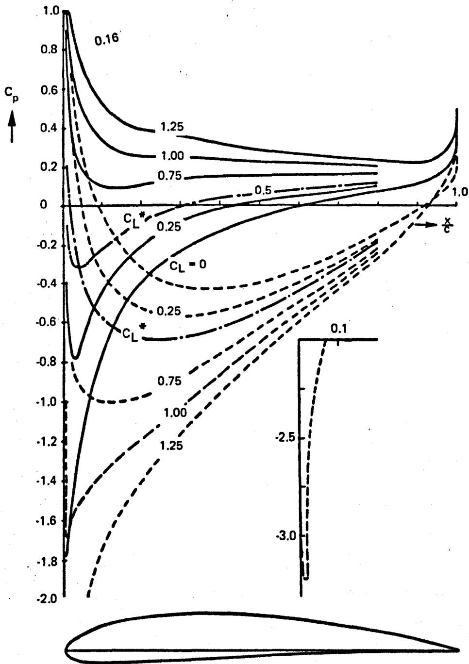
Figure 7.4 – Change of Pressure Distribution with Angle of Attack (Change in Lift Coefficient). From Riegels<sup>7.4</sup>.
