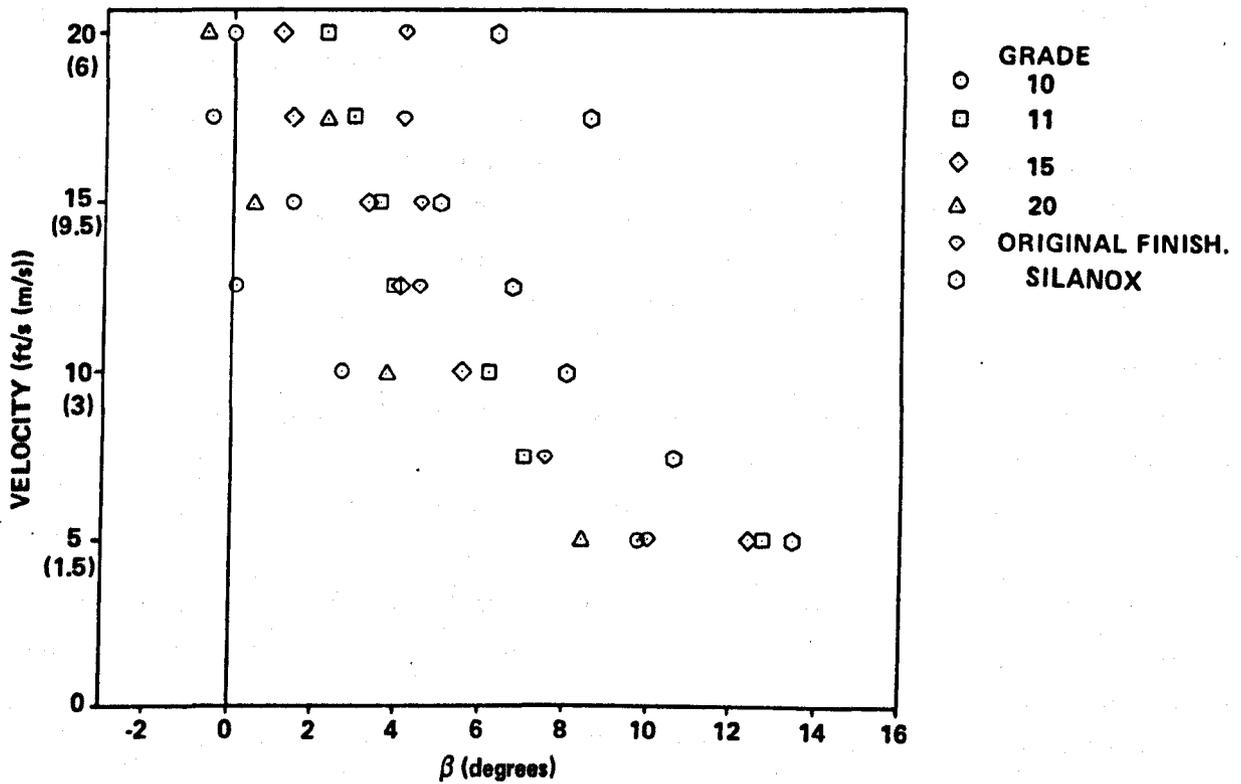
Figure 5.16 – Washout Angle vs Speed for NACA 0012 Mk II with Roughness, Silanox Coating and Plain.
