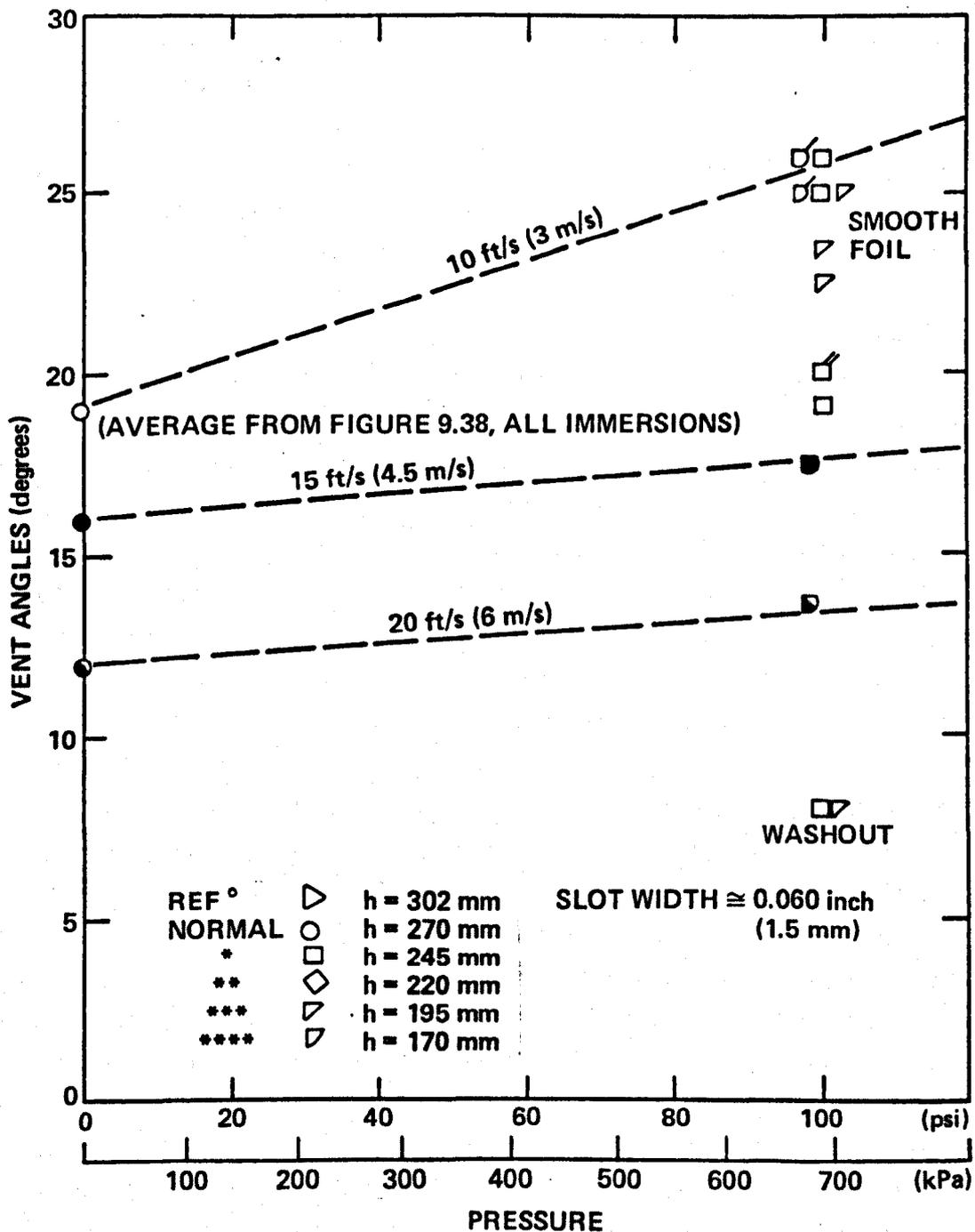
Figure 9.39 – Ventilation Angle Versus Blowing Reservoir Pressure, NACA 16 021 Foil With Shortened, Wide Slots, With Roughness.
