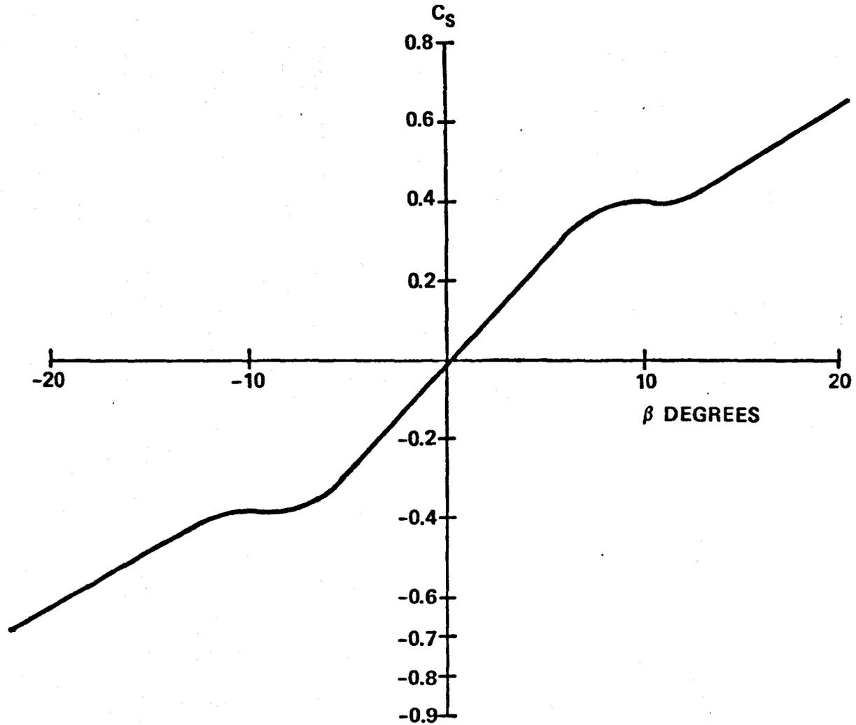
Figure 9.2 – Sideforce Coefficient Versus Sideslip Angle,  $\beta$ , For a NACA 16 021, 100mm Chord Strut, Immersed to 1.9c, 3m/s. From Wright, Et AL<sup>9.26</sup>
