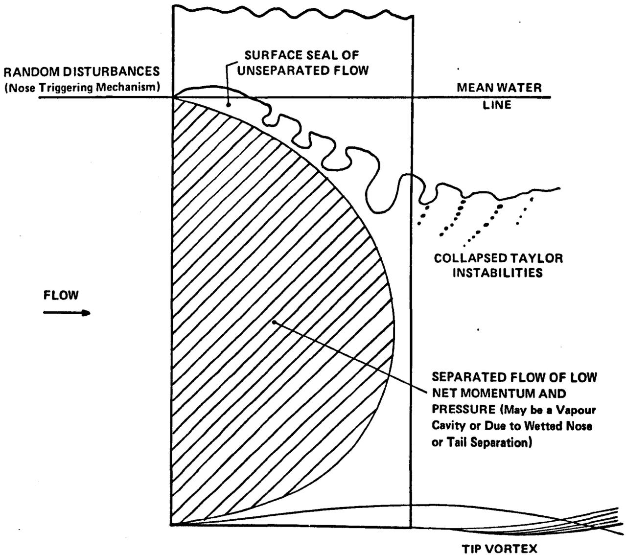
**Figure 2.4 – Principal Features of Flow Immediately Before Ventilation Inception.**
