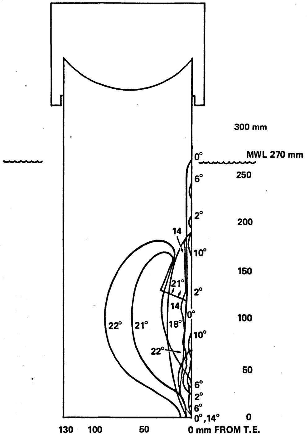
Figure 9.12 – Development of Separation on NACA 16 021 Strut, 10 ft/s (3m/s), 270mm Immersion.
