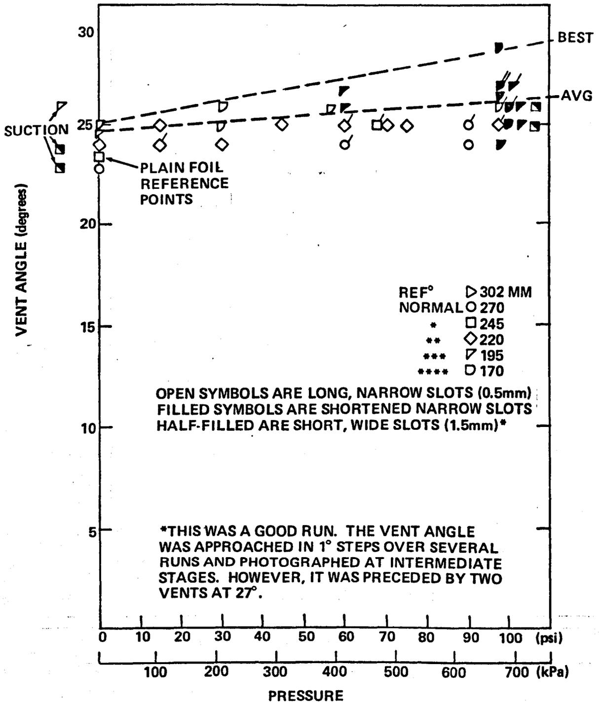
**Figure 9.30 – Ventilation Angle Versus Reservoir Pressure, NACA 16 021 Foil With Long, Narrow, Vertical Slots, Shortened Slots, and Widened Slots. 10 ft/s (3m/s).**
