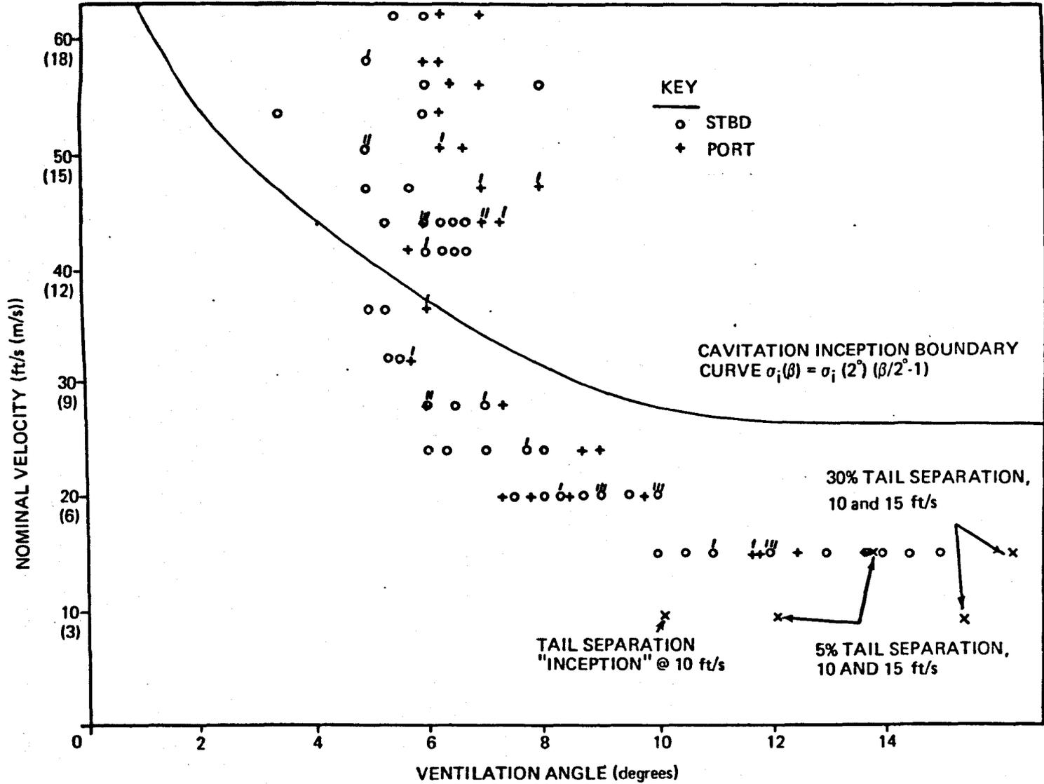
**Figure 6.6 – Ventilation Angles vs Velocity, NACA 0012 Model with No. 10 Roughness. Percent Figures Indicate Extent of Tail Separation in Smooth Case for Like Velocities and Incidence Angles.**
