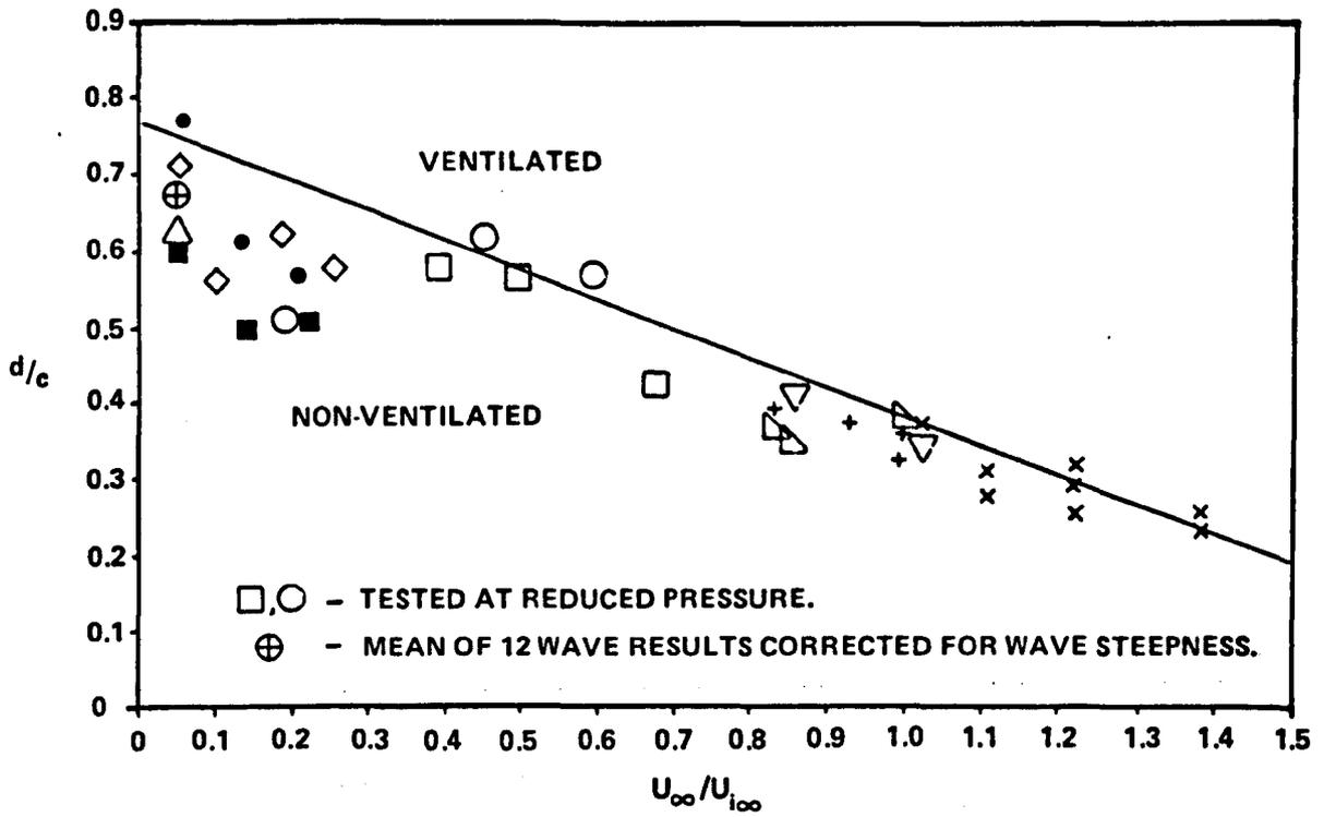
Figure 4.7 – A Criterion for Tail Ventilation
