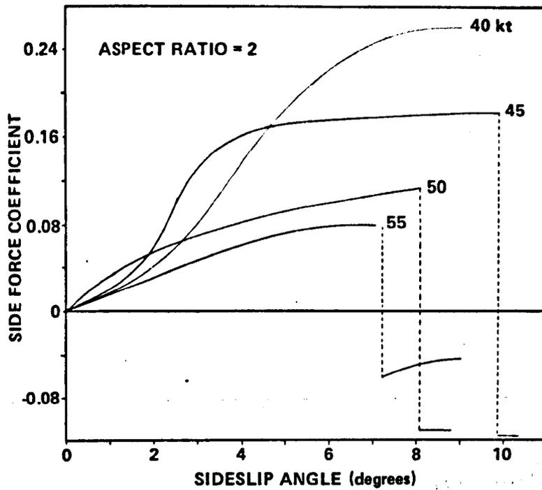
Figure 4.1 – Falloff of Sideforce Coefficient Prior to Ventilation, from Rothblum and Mayer<sup>4,7</sup>.
