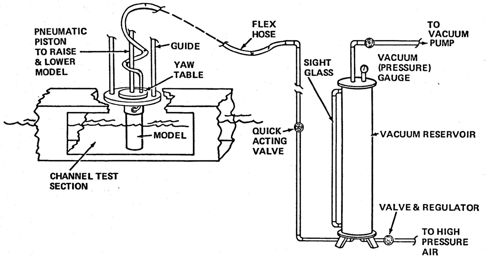
Figure 8.11 – Suction System and General Arrangement of Yawing and Immersion Apparatus
