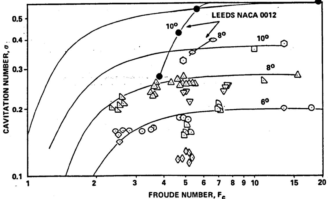
Figure 4.6 – Ventilation Boundary Correlation for Geometrically Similar Versions of NSRDC Strut Model 2 (similar to NACA 16-021). Also Shown are Boundary Points for NACA 0012. Data Taken from Present Tests and Rothblum et al.,<sup>4,7</sup> Waid,<sup>2,11</sup> and Wright et al.<sup>4,10</sup>
