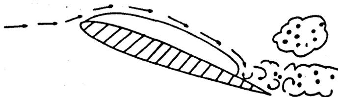
AS THE ELASTIC LIMIT OF THE CAVITY IS REACHED, THE FLOW BEHIND THE CAVITY SLOWS AND THEN REVERSES.
