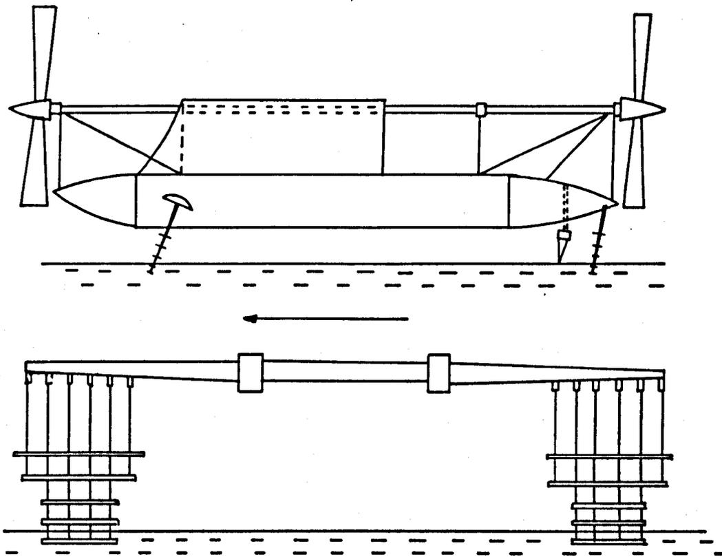
Figure 1.3 – Forlanni Ladder Foil, from Hayward<sup>1,1</sup>, Probably Based on Patent Sketch (1905).
