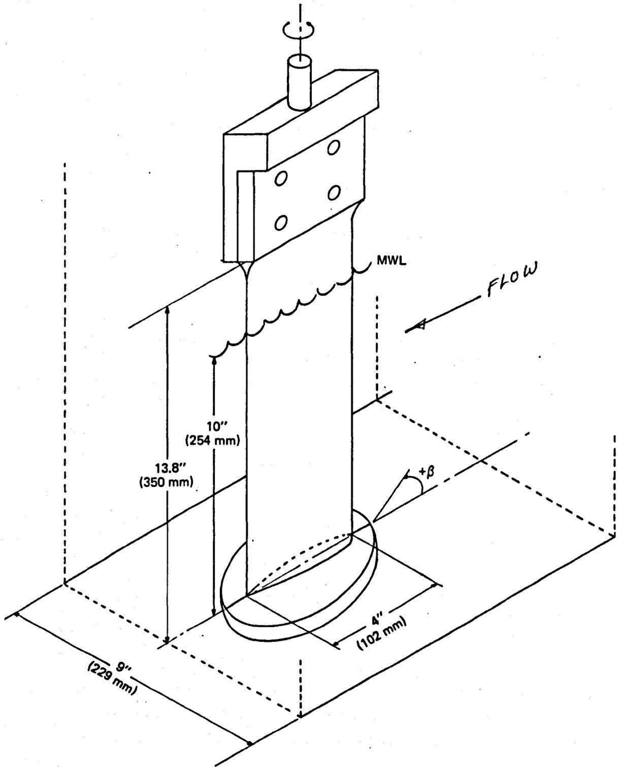
Figure 6.4 – Sketch of Method of Mounting NACA 0012 Mk II Strut Showing Principal Dimensions.
