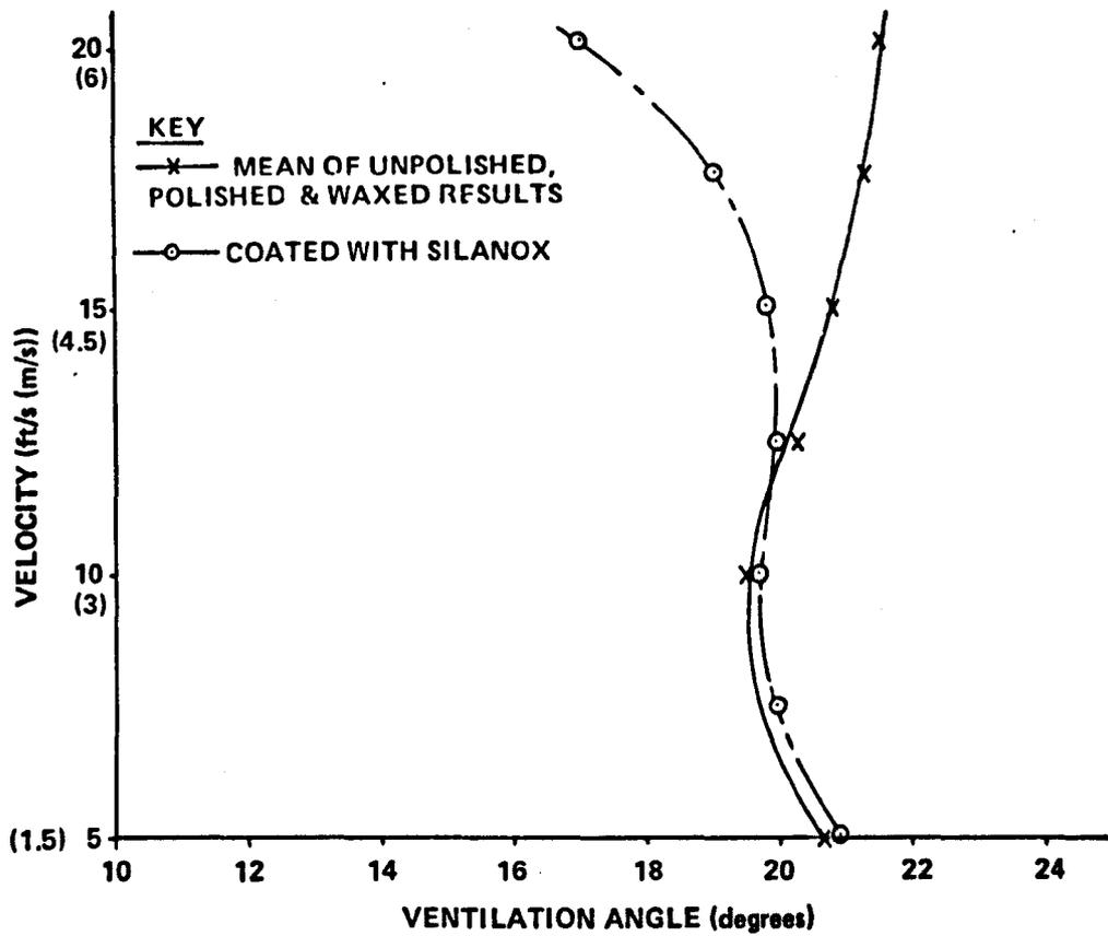
Figure 5.13 – Effect of Surface Contact Angle.
