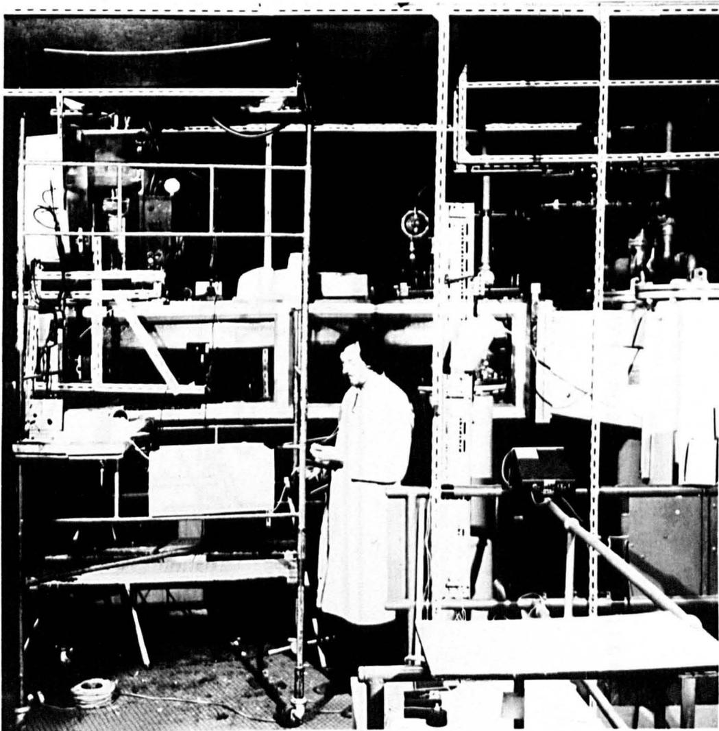
Figure 8.10 – Flow Visualisation Apparatus As Used With Blunt Biogive Suction Model In Free Surface Water Channel
