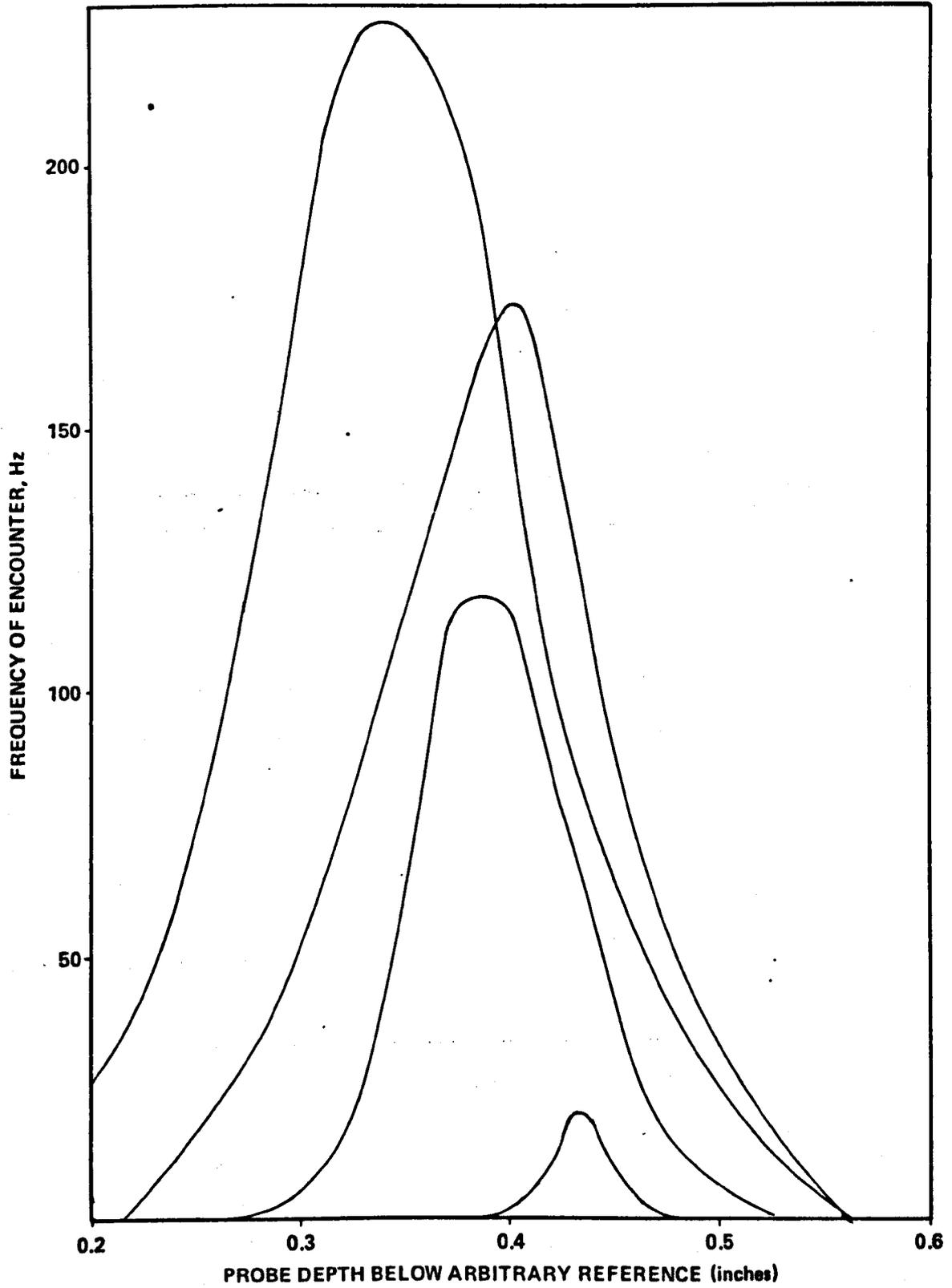
Figure 5.3 – Surface Quality of Channel: Frequency of Encounter with Disturbances vs Probe Depth. From Wright.<sup>5,6</sup>
