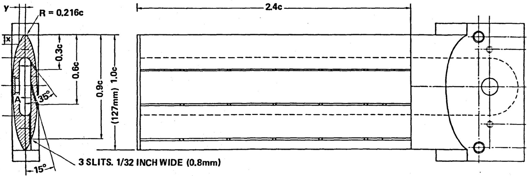
Figure 9.1 - NACA 16 021 Section Shape and Planform as Modified for Blowing. Chordlength 127mm, Design Submergence, 2c.
