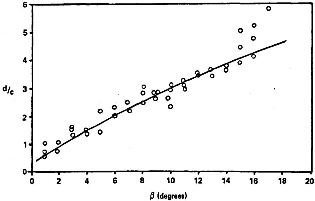
Figure 4.8 – Values of  $d/c$  Against Sideslip Angle  $\beta$  for a Flat Plate, Which Can Be Used to Determine Approximate Inception Angles for Tail Ventilation. From Swales, Wright, McGregor & Rothblum<sup>4.11</sup>.
