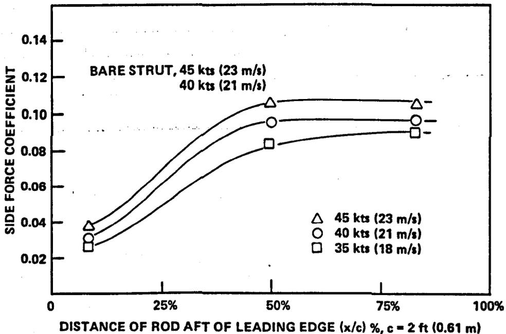
Figure 4.4 – Effect of Chordwise Position of Protuberance on Sideforce Coefficient at a Constant Angle of 5 degrees. From Rothblum, Dailey and Pattison<sup>4.10</sup>.
