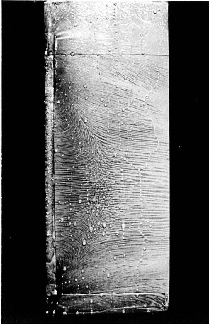
Figure 8.9 – Blunt Bio-give with Roughened Leading Edge. 20 ft/s
