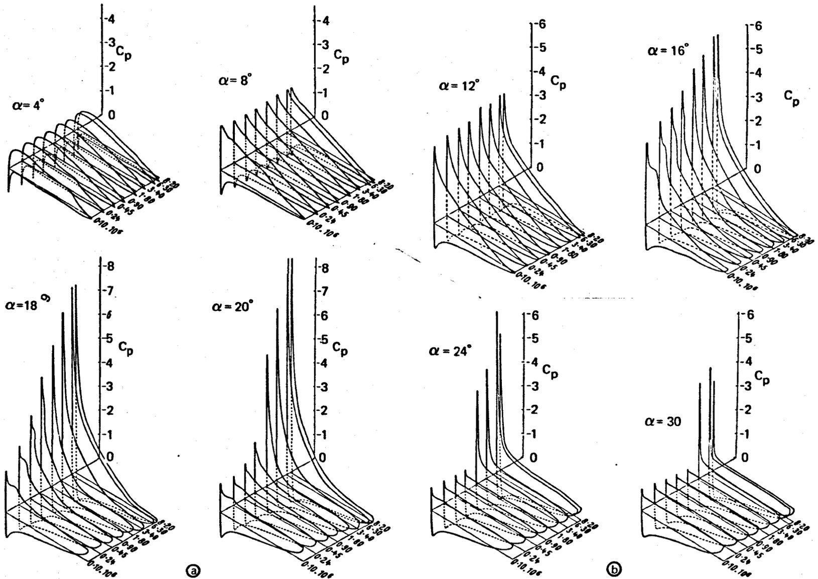
Figure 7.5 – Influence of Reynolds Number on the Pressure Distribution. Profile: 4412. VDT [R 613]. From Riegels<sup>7.4</sup>.
