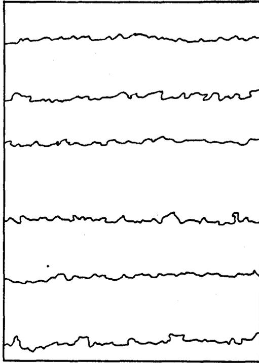
Figure 5.11 – Typical Surface Profiles of 180 Grit Emery Paper (magnification x 50).
