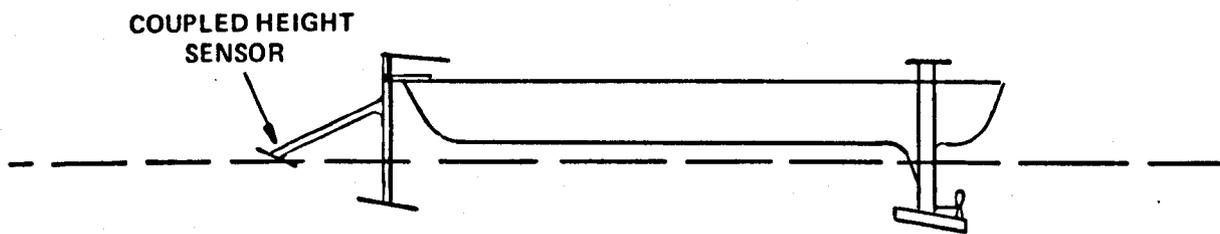
Figure 1.5 – Meacham Incidence Control System, from Hayward<sup>1.1</sup>, Probably Based on Patent Sketch (1896).
