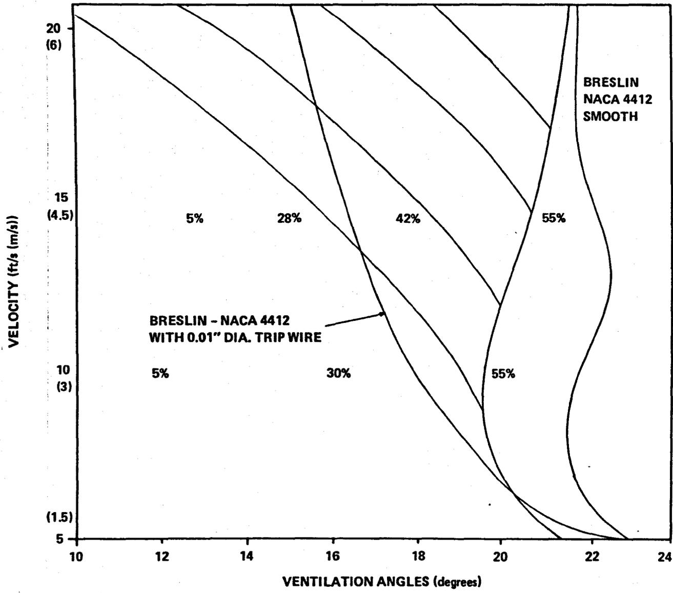
Figure 5.17 – Breslin<sup>5.9</sup> Trip Wire Data Compared to Results of Present Study.
