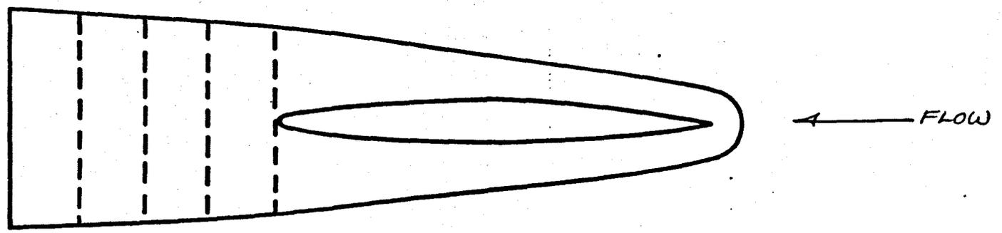
Figure 10.1 – Proportions of Typical Fence Found Effective Against Tail Ventilation.
