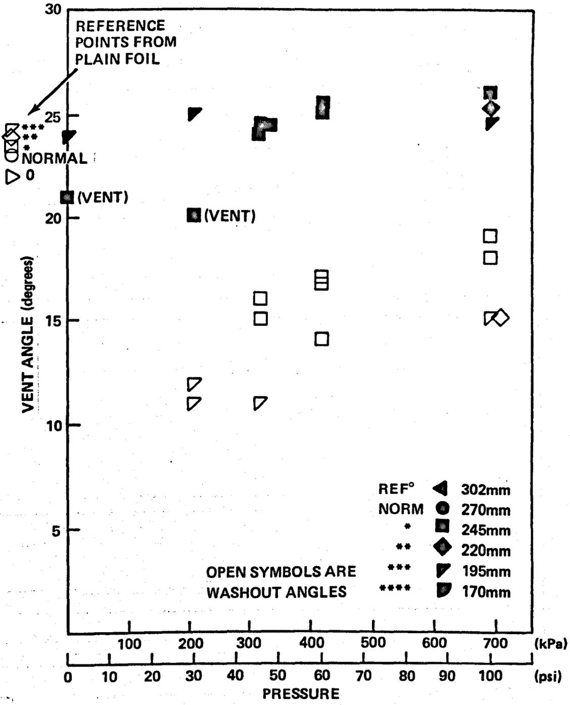
Figure 10.12 – Ventilation Angle Versus Reservoir Pressure, NACA 16 021 Foil With Horizontal Slot Blowing, 10 ft/s (3m/s) High Pressure Series (III).
