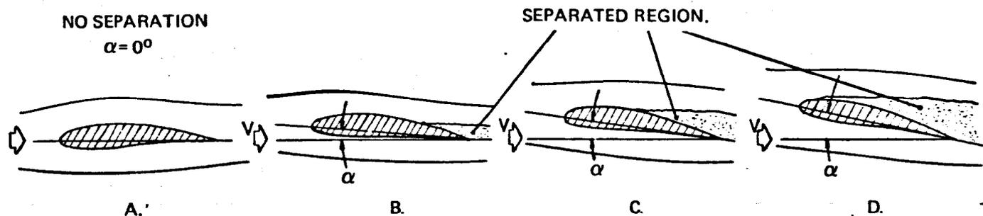
Figure 7.2c – Trailing Edge Stall (Turbulent Tail Separation).
