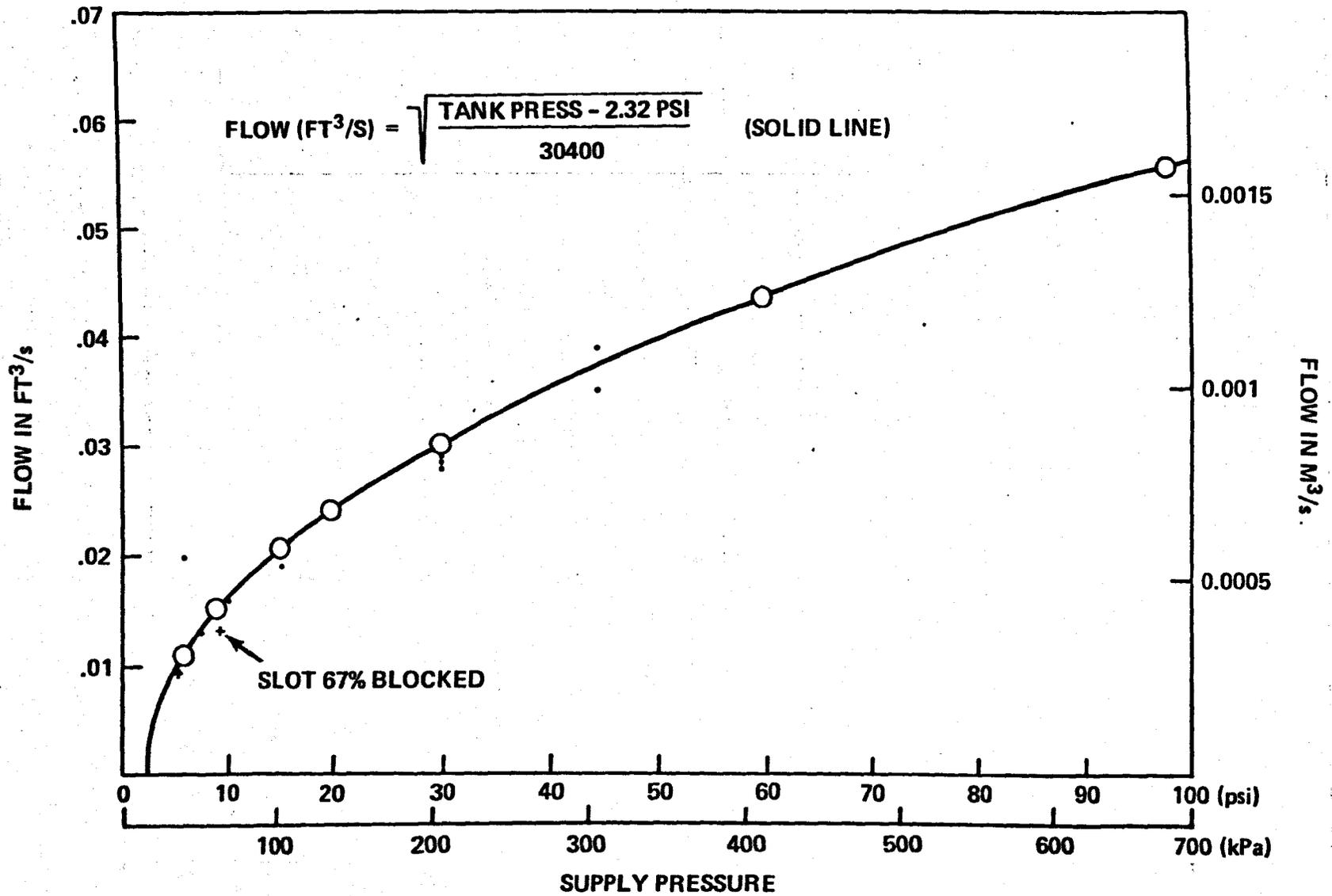
Figure 10.3 – Flow in Slots Versus Reservoir Pressure.
