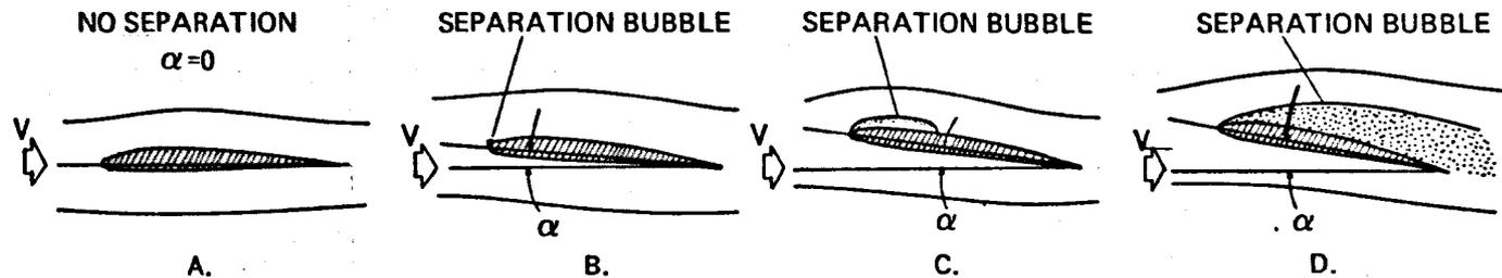
Figure 7.2a – Long, or Growing, Bubble (Thin Airfoil) Type Separation.
