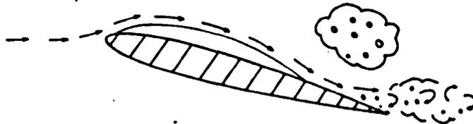
THE VAPOUR CAVITY EXPANDS DOWNSTREAM, WITH THE ATTACHED WATER PRECEDING IT, SWEEPING AWAY THE SEPARATED REGION.
