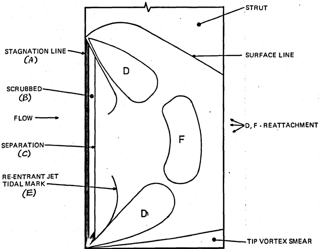
Figure 6.13 – Diagram of a Flow Visualisation Pattern.
