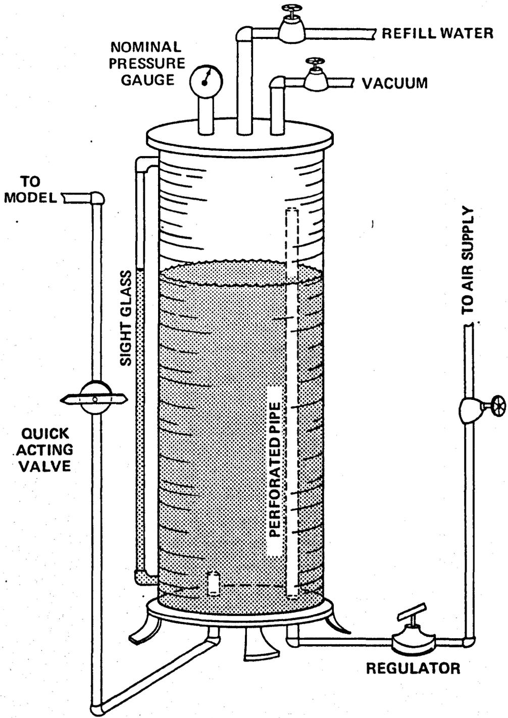
Figure 9.6 – High Pressure Water Supply for Mk I and II Models.
