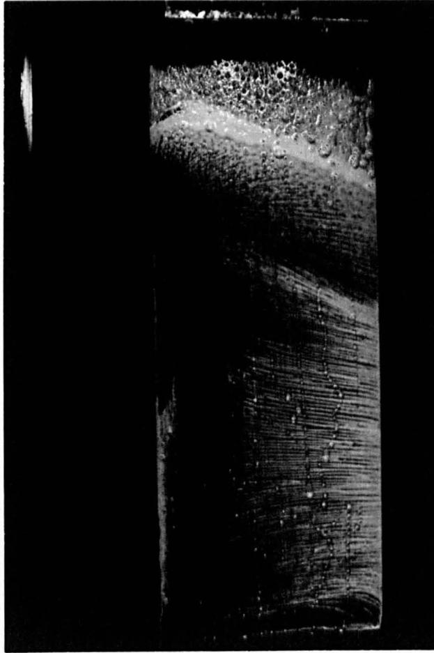
Figure 8.14 – Characteristic “Herringbone” Pattern Caused by Separation and Re-attachment.
