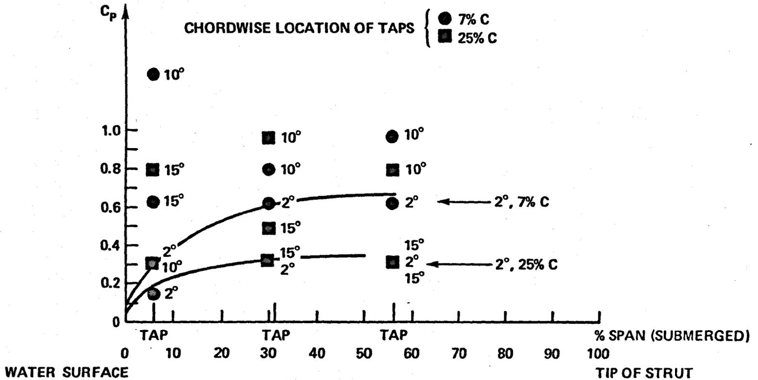
Figure 8.5 — Experimental Pressure Coefficient versus Span, 5ft/s, (1.5m/s),  $\beta = 2$  Degrees, 10 Degrees and 15 Degrees Blunt-Nosed Bioigive. Data From Reference 8.3, Taken at 0.07C and 0.25C.
