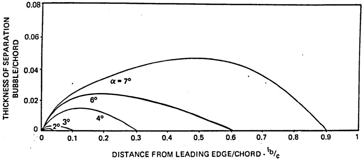
Figure 7.3a – Size of Separation Bubbles for Double Wedge Section for Various Angles of Attack
