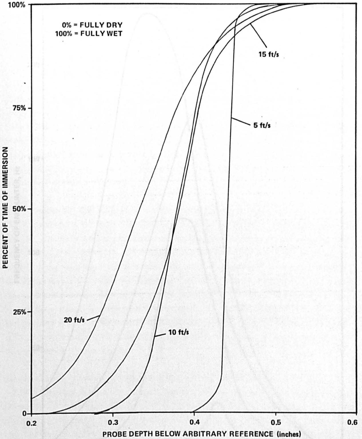
Figure 5.2 – Surface Quality of Channel: Percent of Time for Which a Probe Was Wetted vs Probe Depth. From Wright.<sup>5,6</sup>
