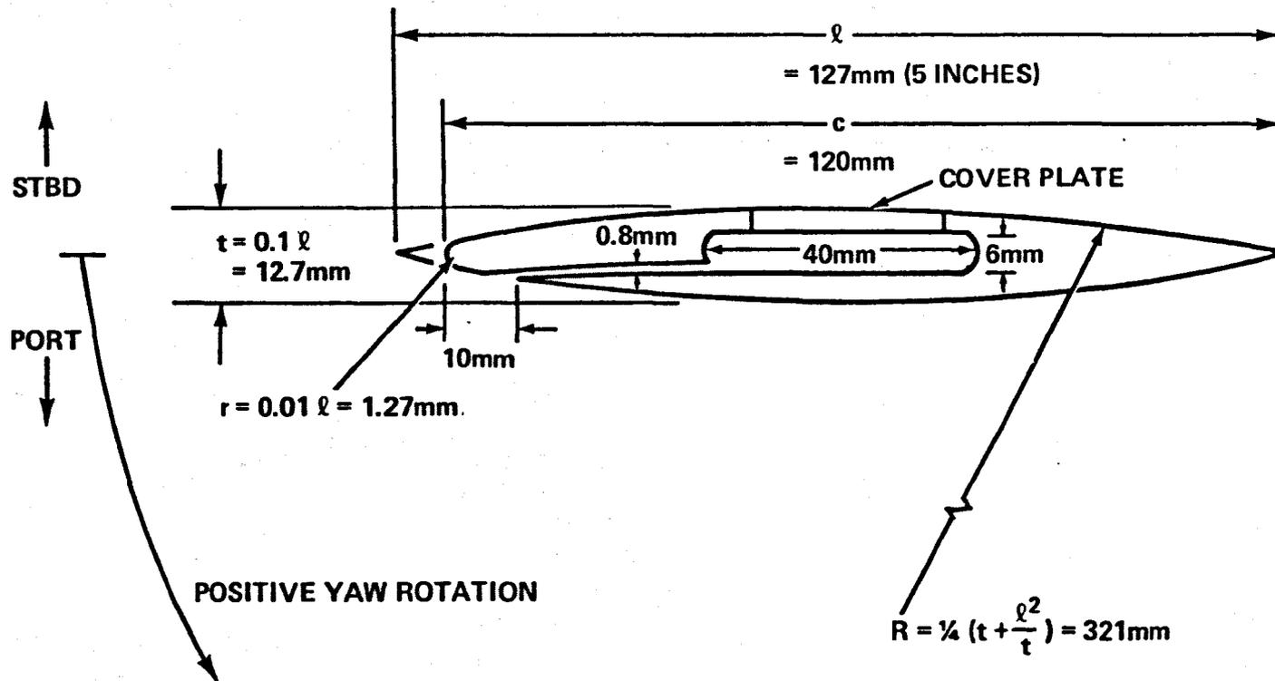
Figure 8.1 — Section of Blunt-Nosed Biogive Showing Principal Dimensions
