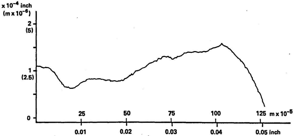
Figure 5.9 – Mk II NACA 0012 Foil Before and After Polishing (Note scale change on graphs). Reproductions of Tallysurf Roughness Traces.
