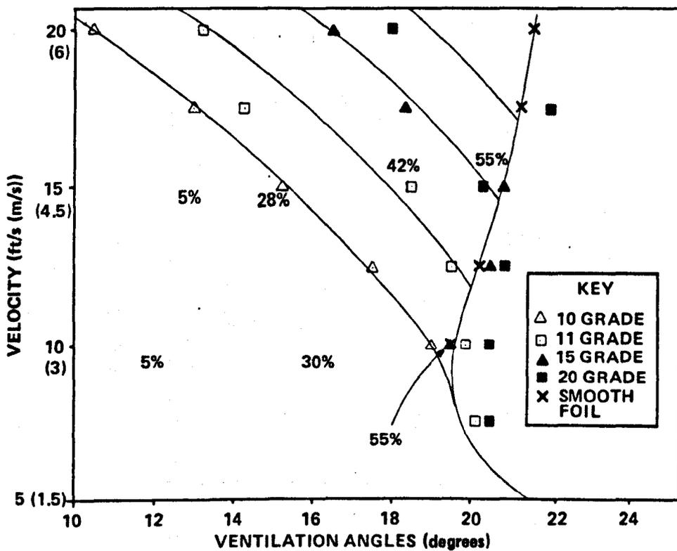
Figure 5.12 – Effect of Roughness on NACA 0012 Strut. Figures Show Amount of Separation Measured in Percent of Chord on Smooth Foil.
