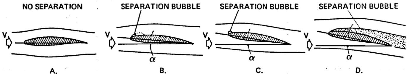
Figure 7.2b – Leading Edge Stall (Short or Shrinking Bubble).
