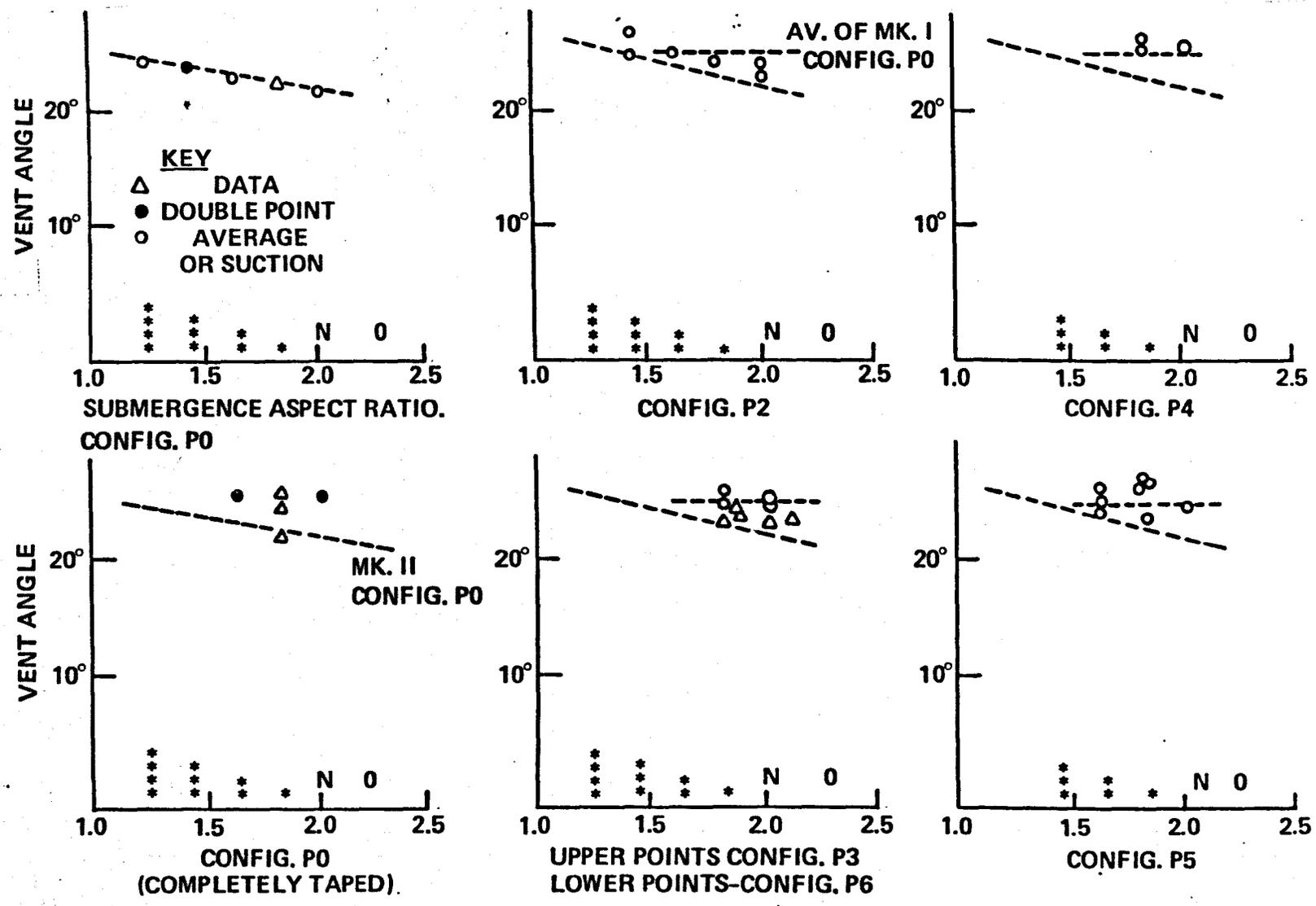
Figure 9.10 – Ventilation Angles Versus Submergence Aspect Ratio For Preliminary Tests With Suction From Vertical Slots, NACA 16 021 Model, 10 ft/s (3m/s).
