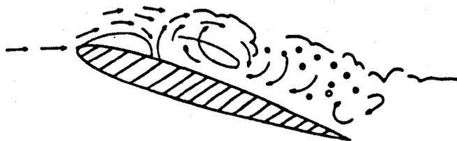
THE THICKNESS OF THE JET EXCEEDS THE CONFINES OF THE CAVITY WALL AND THE RE-ENTRANT FLOW IS SWEEP BACKWARDS AND DOWNSTREAM.
