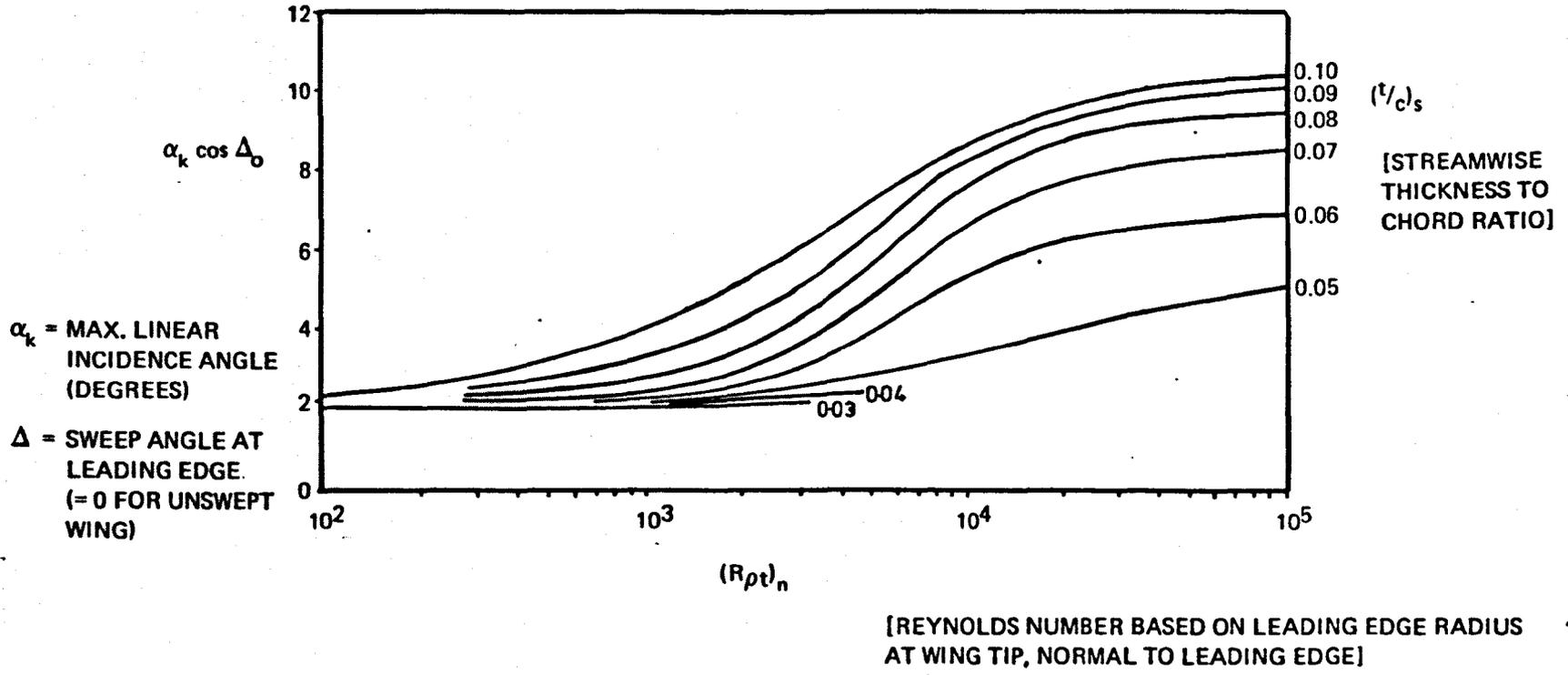
Figure 7.10 – Leading Edge Initial Separation Boundaries for Plane Wings with Constant Symmetrical Sections. (Chappell<sup>7.10</sup>)
