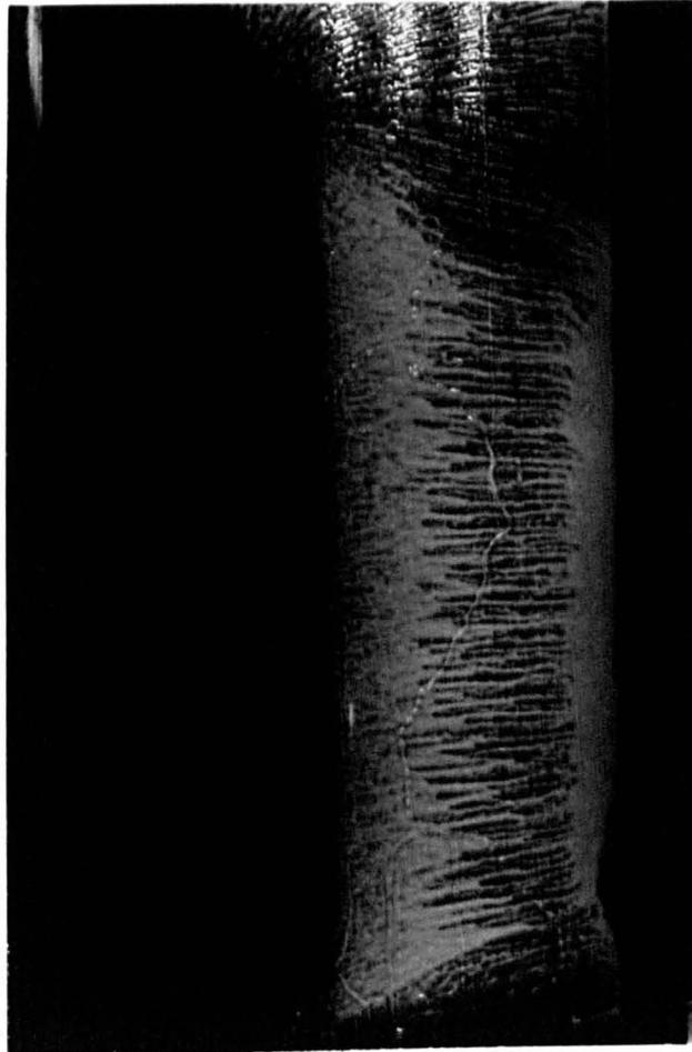
**Figure 8.12 – A Typical Oil Smear Pattern Showing Transition from Laminar to Turbulent Flow. The Fully Turbulent Region is Scoured by High Shear Stresses.**
