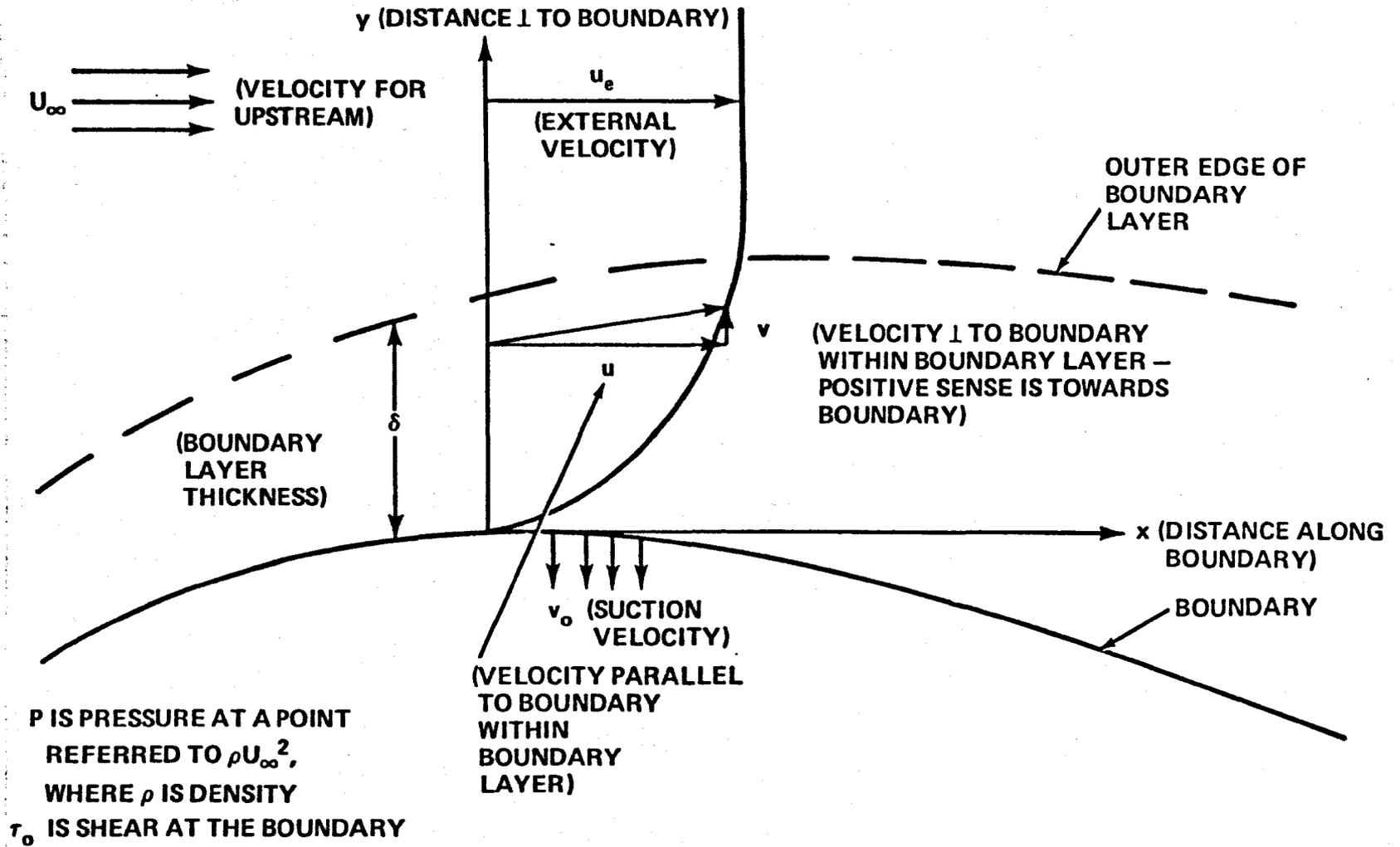
Figure 8.2 – Notation Used in Boundary Layer Theory
