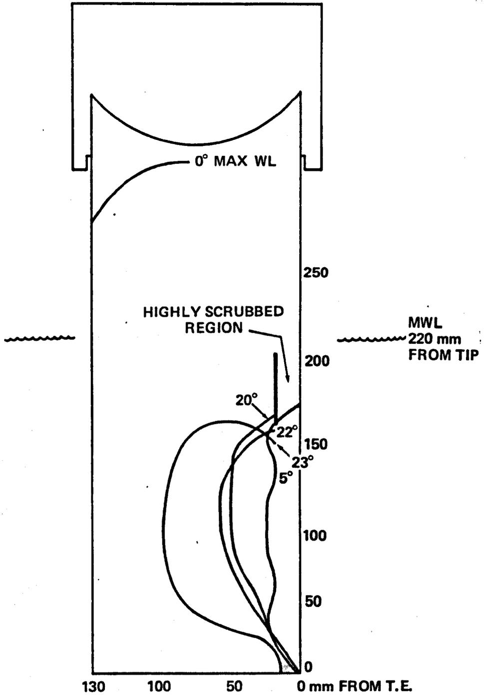
Figure 9.16 — Development of Separation on NACA 16 021 Strut, Configuration P6\*\*,
