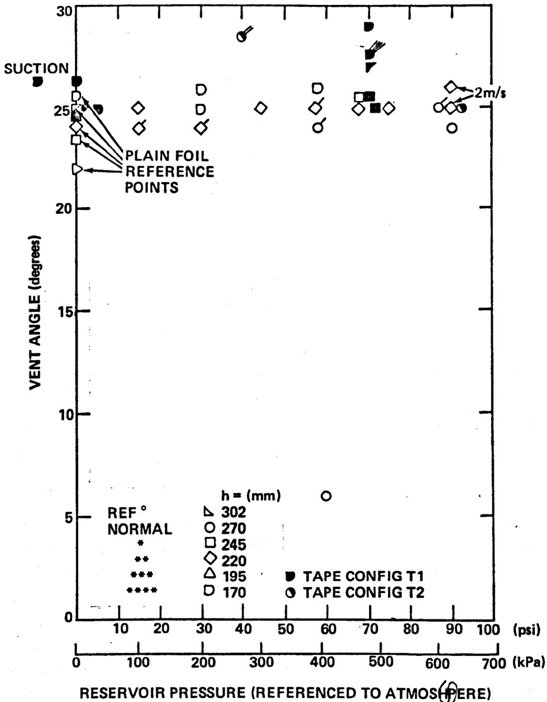
Figure 9.23 – Ventilation Angle Versus Reservoir Pressure, NACA 16 021 Foil With Long, Narrow, Vertical Slots, Plain and Taped, 10 ft/s (3m/s).
