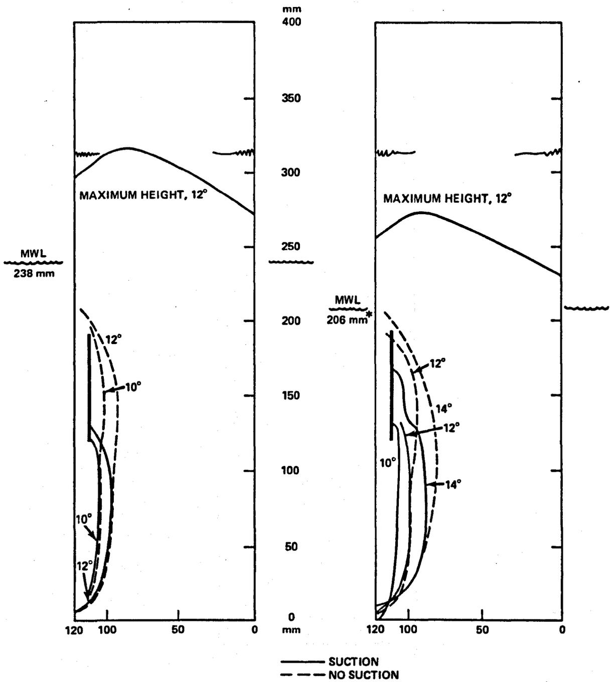
Figure 8.17 – Re-attachment Lines, Blunt Biogive, 20 ft/s (6m/s), Short Slot Below Surface.
