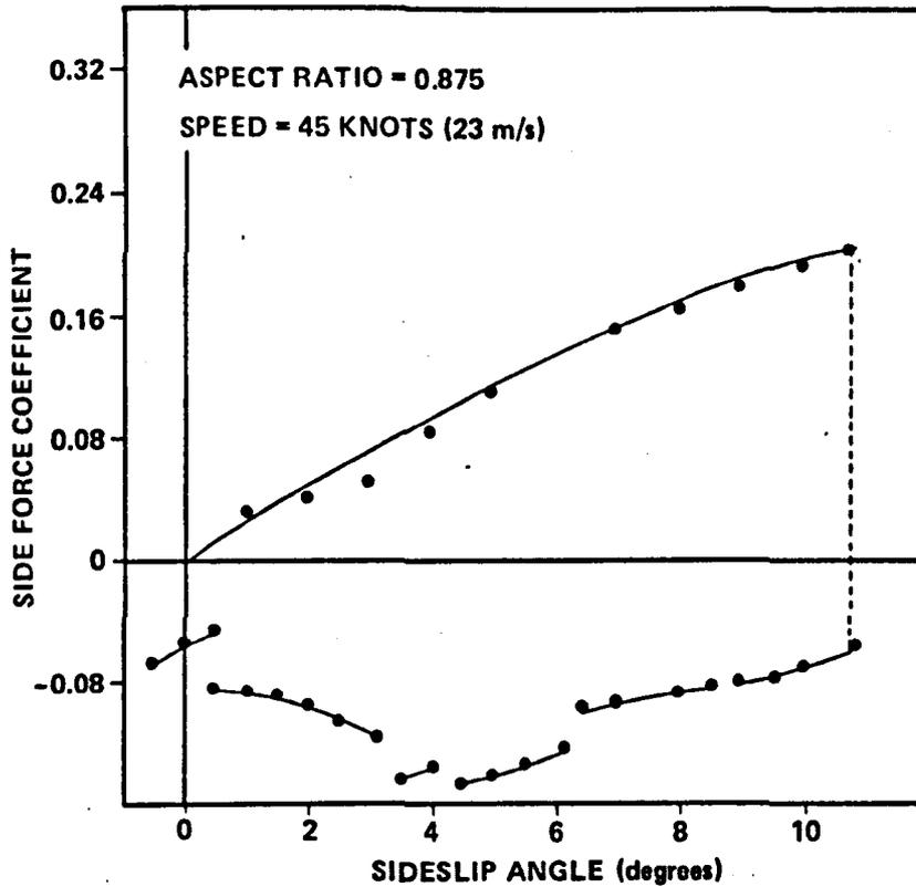
Figure 4.3 – Side Force Coefficient vs Sideslip Angle for Taylor Center Model 4, Ventilated and Non-Ventilated. From Rothblum, Mayer and Wilburn<sup>4.7</sup>.
