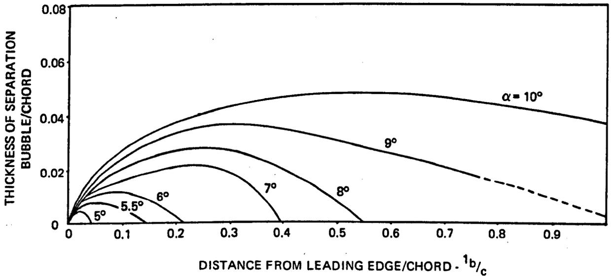
Figure 7.3b – Size of Separation Bubbles for NACA 64A006 Section for Various Angles of Attack. From Barr<sup>7.1</sup>, and McCullough<sup>7.2</sup>.
