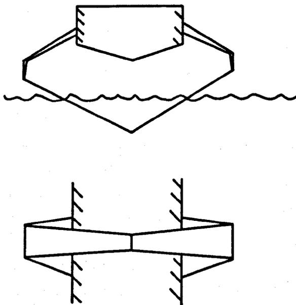
Figure 1.6 – Schertel-Sachsenberg Foil System, Based on Von Schertel<sup>1.2, 1.3</sup> Photographs and Sketches.
