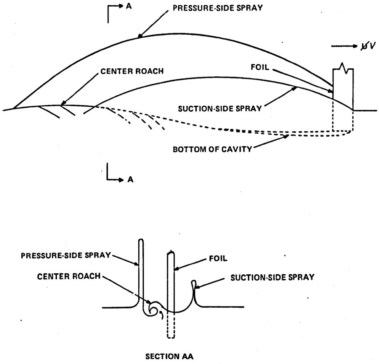
Figure 2.1(b) – Flow Pattern after Ventilation at High Froude Number, from Breslin and Skalak<sup>2,4</sup>.
