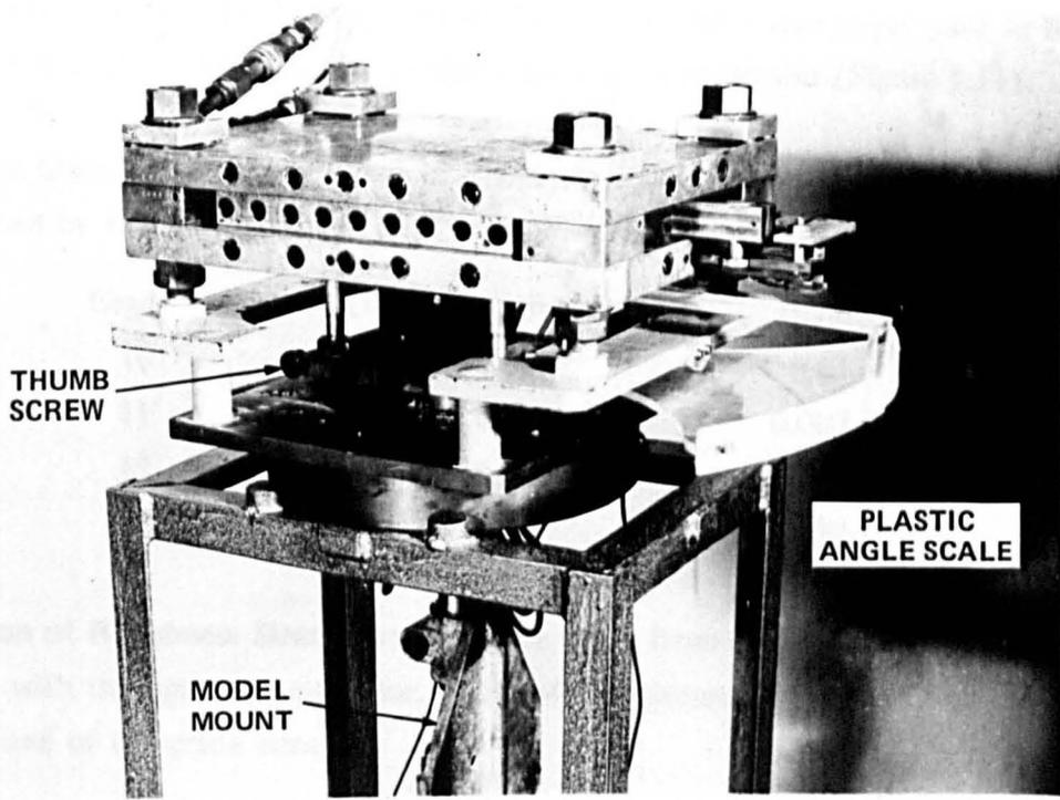
Figure 5.10 – Force Balance and Turning Apparatus.
