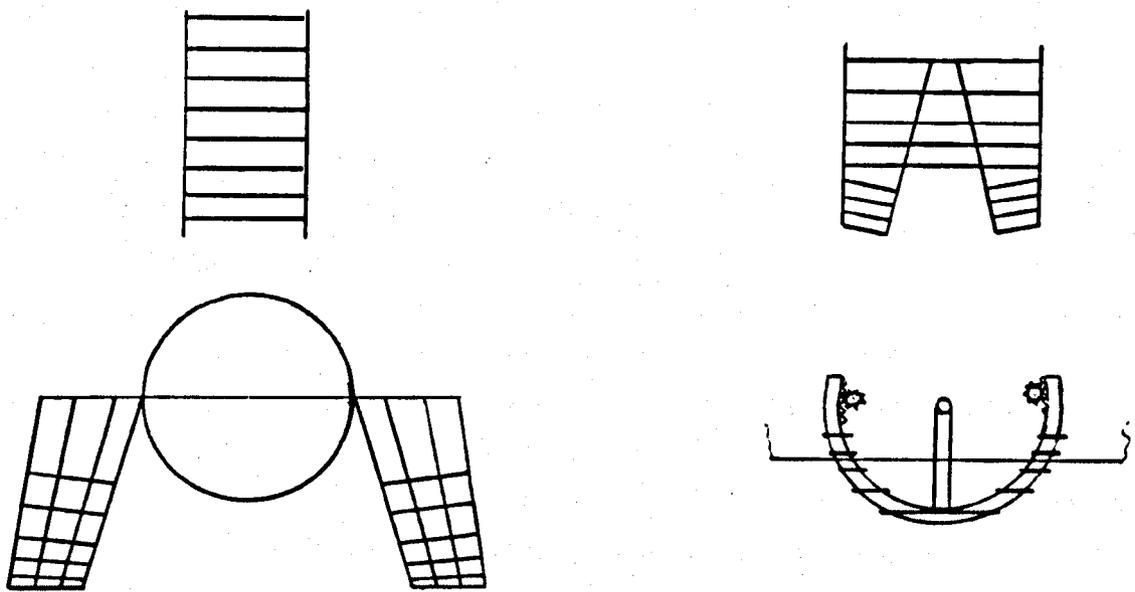
Figure 1.4 – Bell-Baldwin "Hydrodome" Showing Use of Ladder Foils, from Hayward<sup>1,1</sup>, Probably Based on Patent Sketch (1920).
