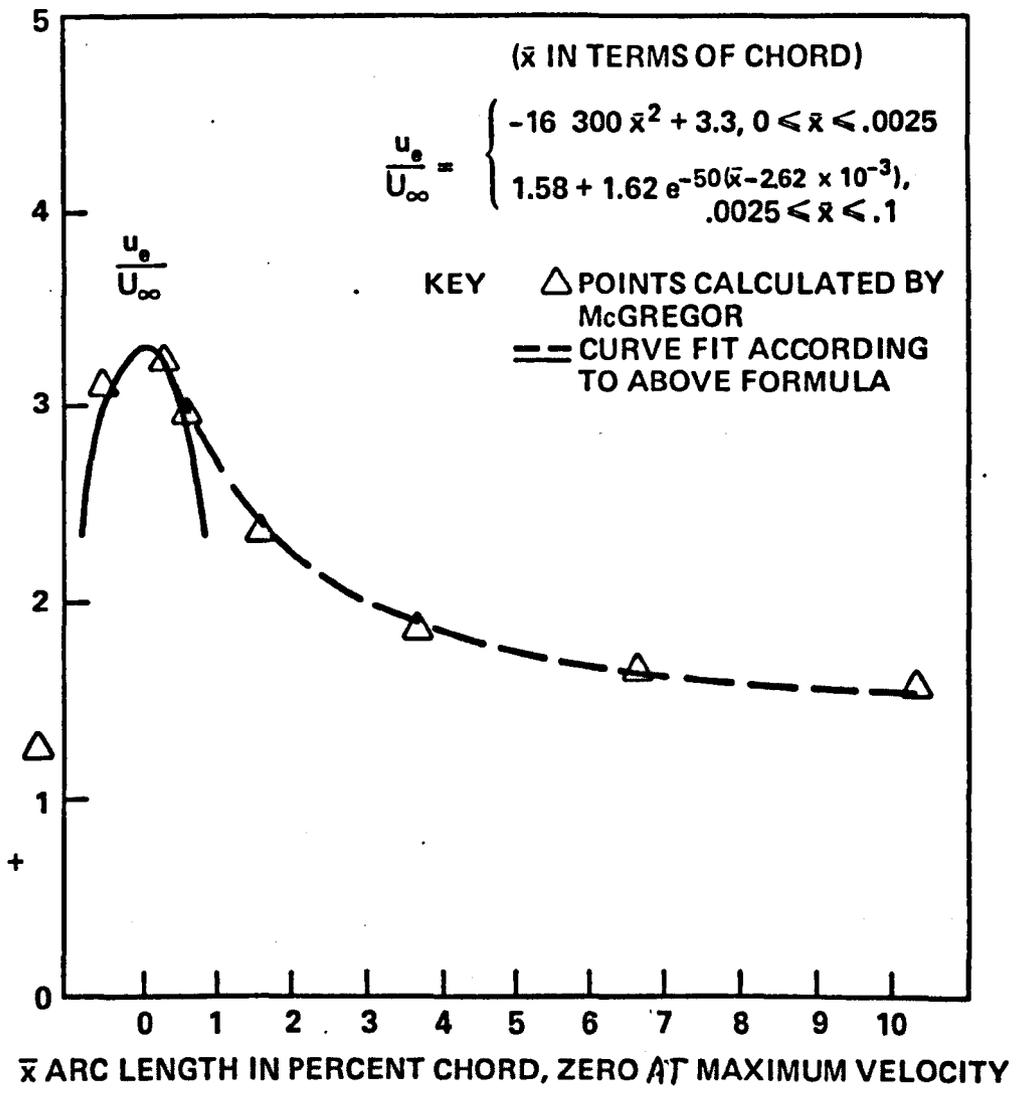
Figure 8.3 – Velocity Distribution Near Nose of Blunt Biogive as a Function of Arc Length from Point of Maximum Velocity.
