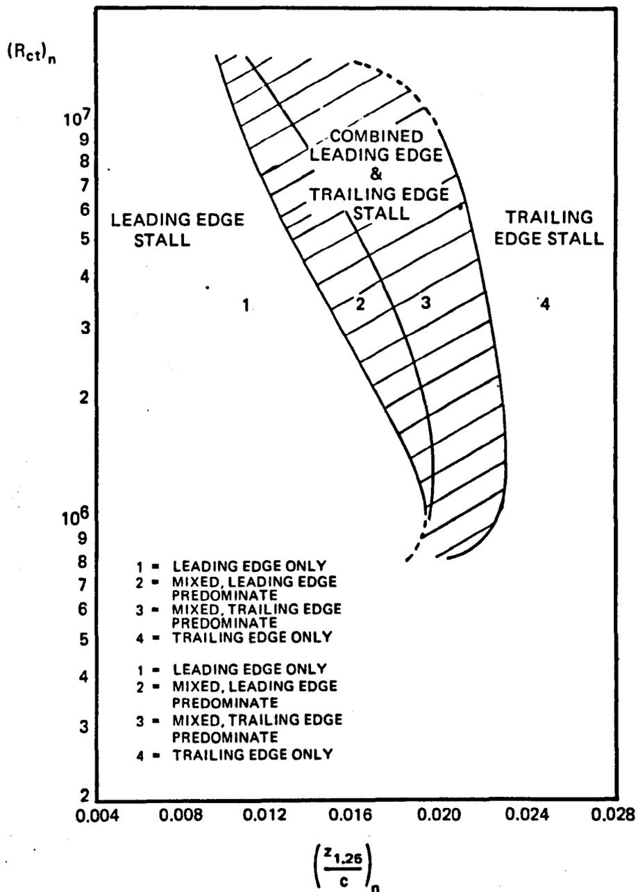
Figure 7.9 – Initial Separation Characteristics of Three-Dimensional Plane Wings with Constant Symmetrical Sections. (Chappell<sup>7.12</sup>)
