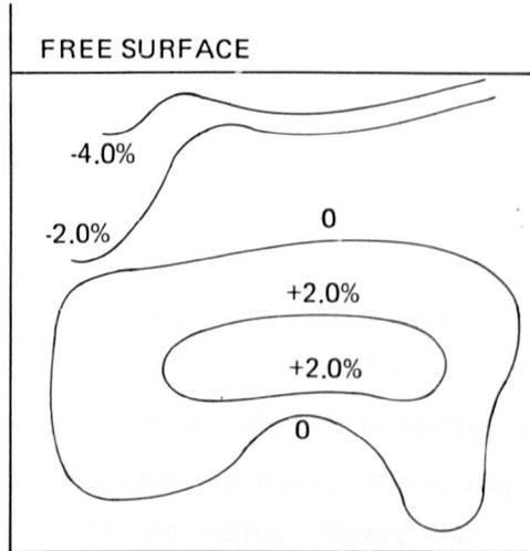
Figure 6.2 – Velocity Distribution in Channel Working Section at 15 ft/s (4.5 m/s). Figures Are Percentage Variations from Mean Velocity. From Hunter et al<sup>6.1</sup>.
