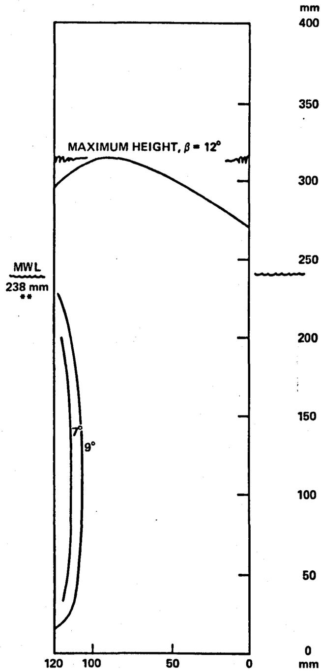
Figure 8.15 — Reattachment Lines, Leads Blunt Biogive, 20 ft/s (6m/s),  $7^\circ \leq \beta \leq 9^\circ$ , Bare Strut.
