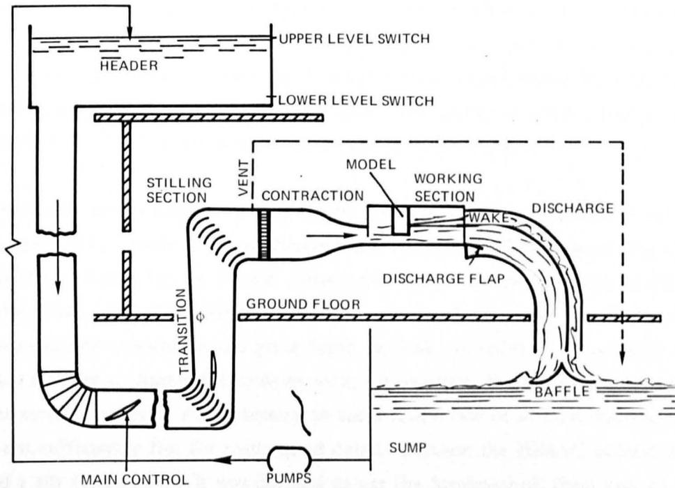
Figure 6.1a – Circuit Diagram of High Speed Channel.
