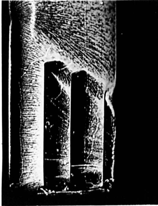
Figure 9.37b – Oil Smear Pattern,  $\beta = 24$  Degrees.
