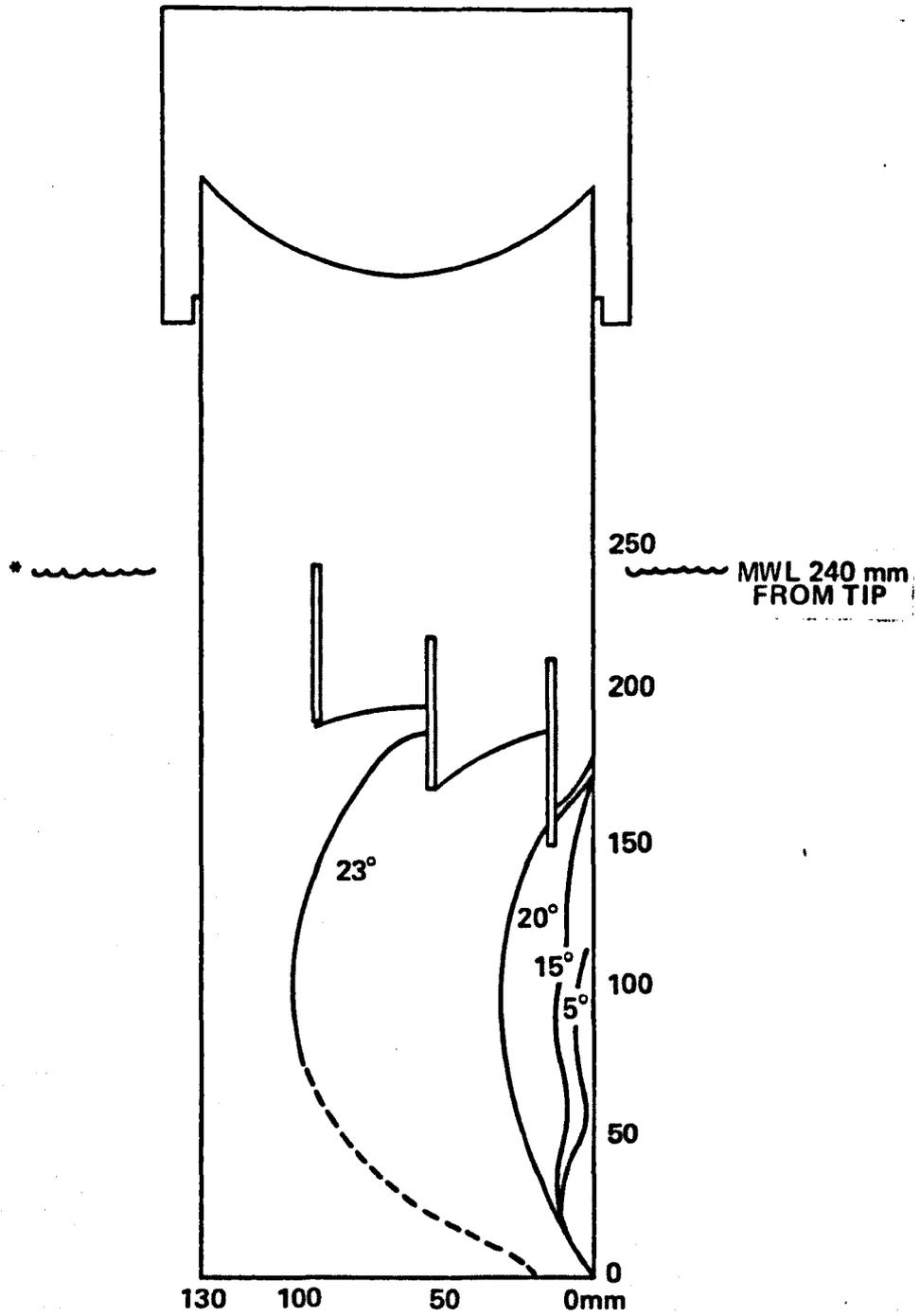
Figure 9.17 – Development of Separation on NACA 16 021 Strut, Configuration P7\*,
