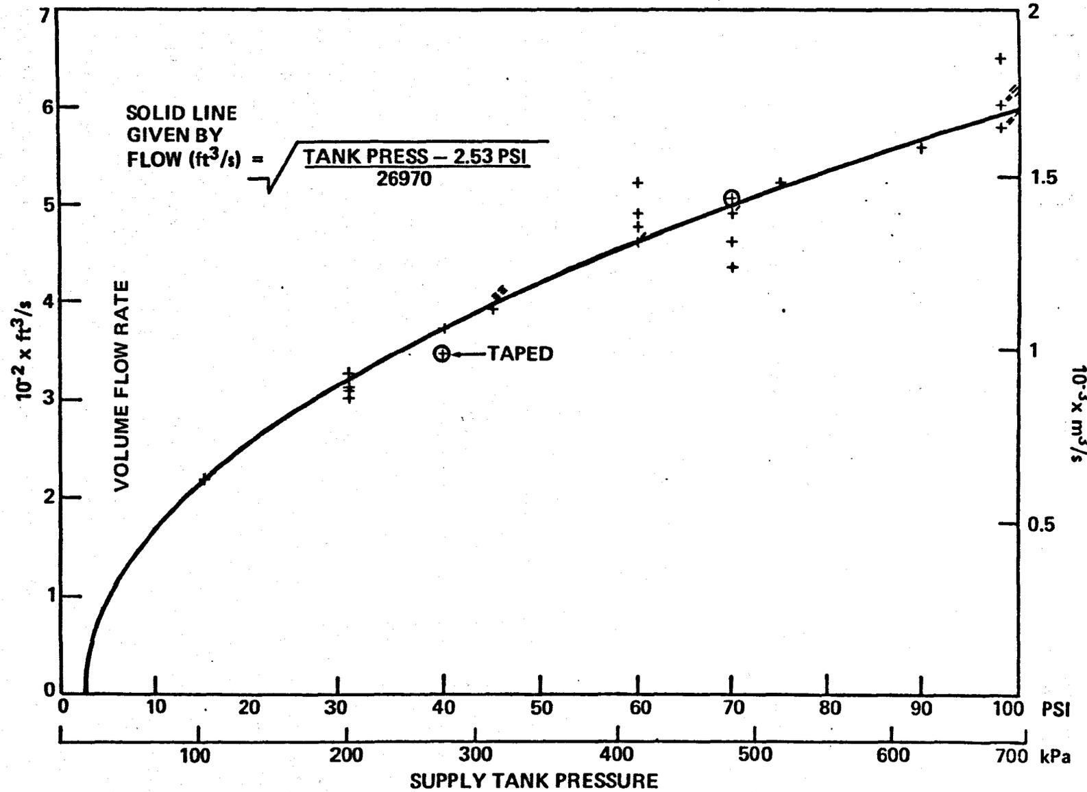
Figure 9.7 – Flow in Slots Versus Supply Pressure, Vertical Slot Model, All Configurations.
