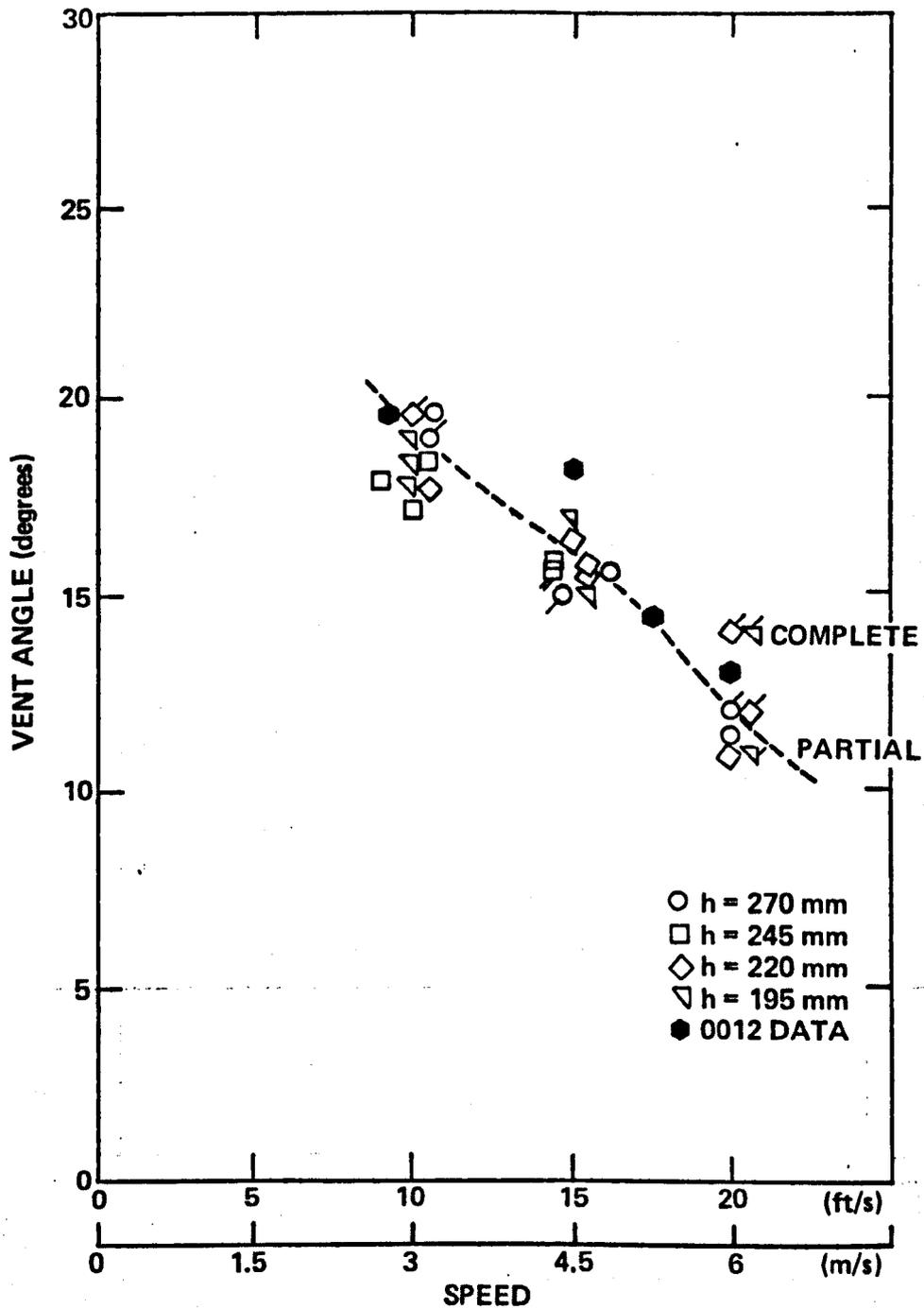
Figure 9.38 – Ventilation Angle Versus Speed For NACA 16 021 Foil With 11 Grade Microsphere Roughness Applied.
