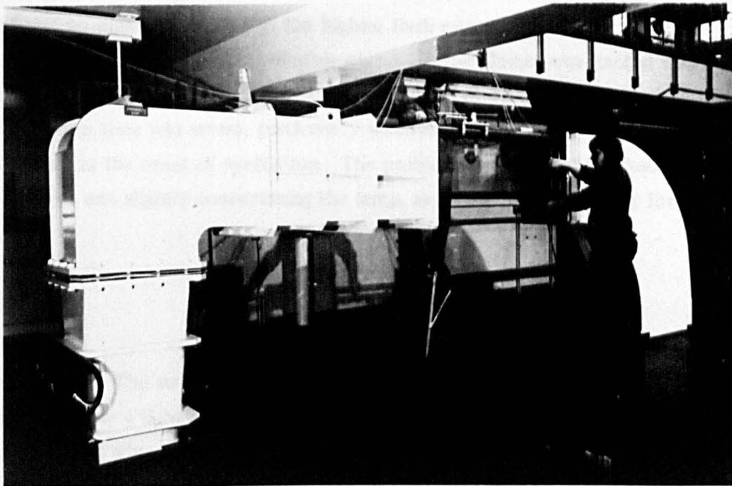
Figure 6.1b – Photograph of Working Section of High Speed Channel.
