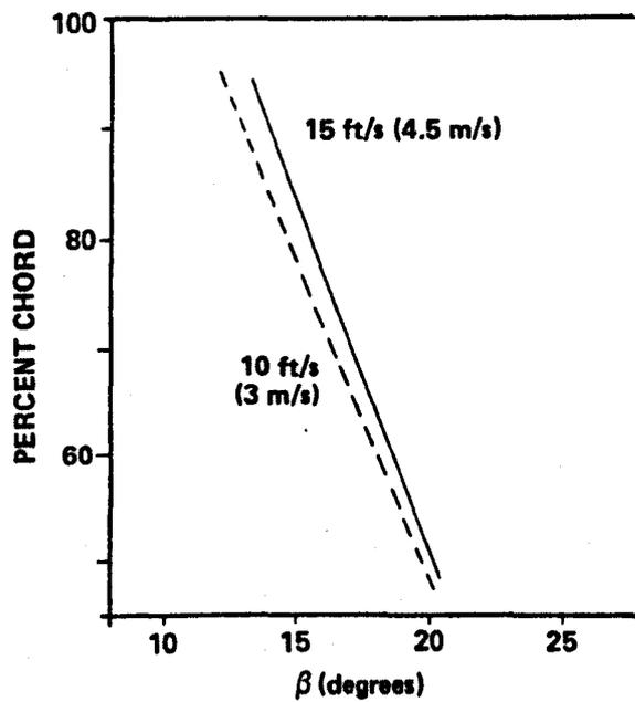
Figure 5.14 – Turbulent Tail Separation as a Percent of Chord for NACA 0012 Foil. From Wright and McGregor.<sup>5,6</sup>
