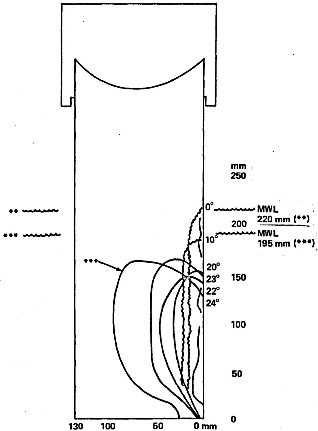
Figure 9.13 – Development of Separation on NACA 16 021 Strut, 10 ft/s (3m/s), 220mm Immersion.
