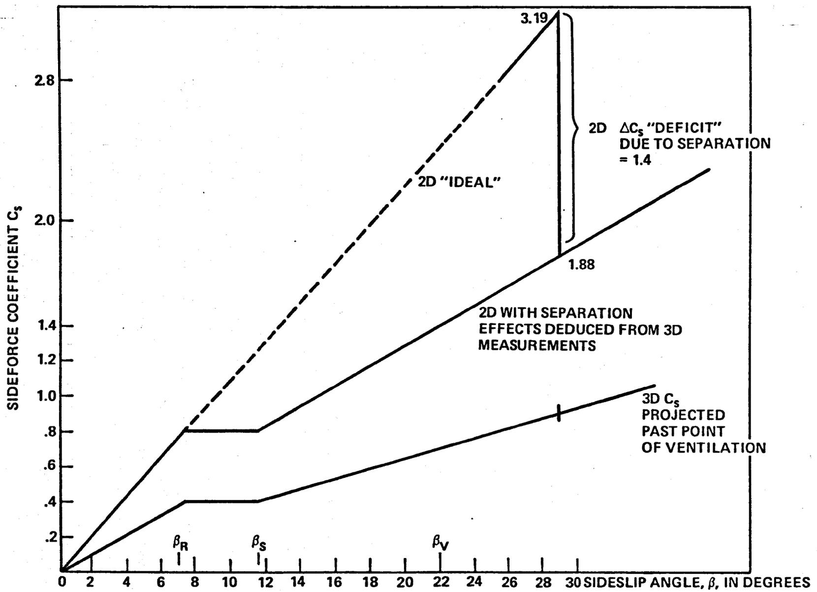
Figure 9.3 – Calculation of Sideforce "Deficit" From Idealised Force Coefficient.
