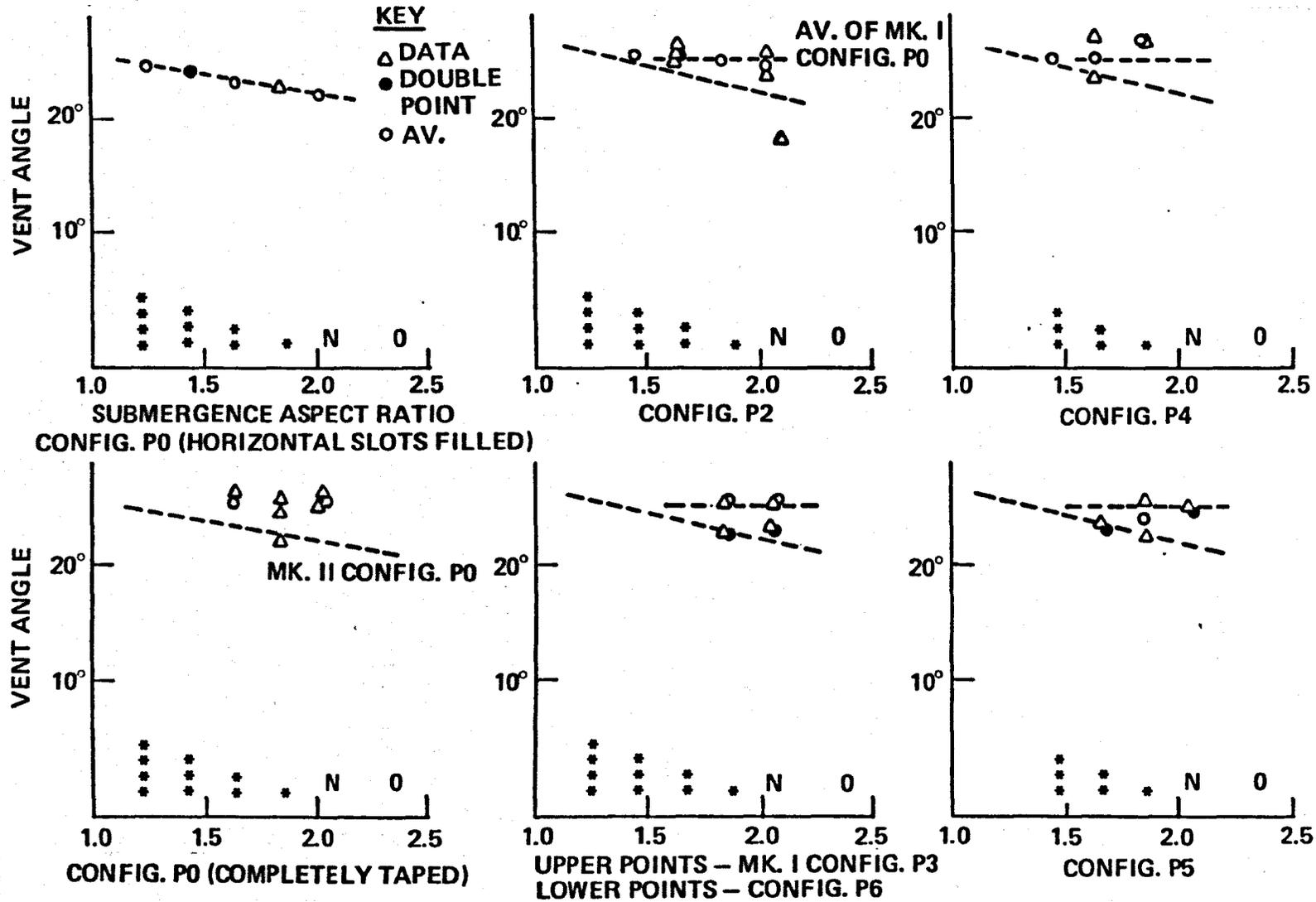
Figure 9.11 - Ventilation Angles Versus Submergence Aspect Ratio For Preliminary Tests, Neutral Pressure In Vertical Slot NACA 16 021 Model, 10 ft/s (3m/s).
