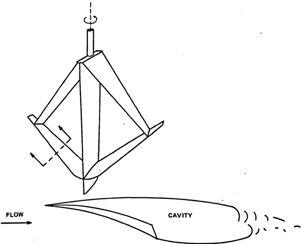
Figure 1.2 – Sketch Representing the Configuration of the Bow Foil of HCMS Bras d'Or (FHE 400), Based on Millman<sup>1,11</sup>. A Supercavitating Foil Section is Also Shown.
