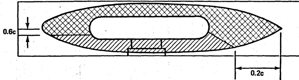
**Figure 10.2 – NACA 16 021 Section and Planform as Modified for Horizontal Slot Blowing.
