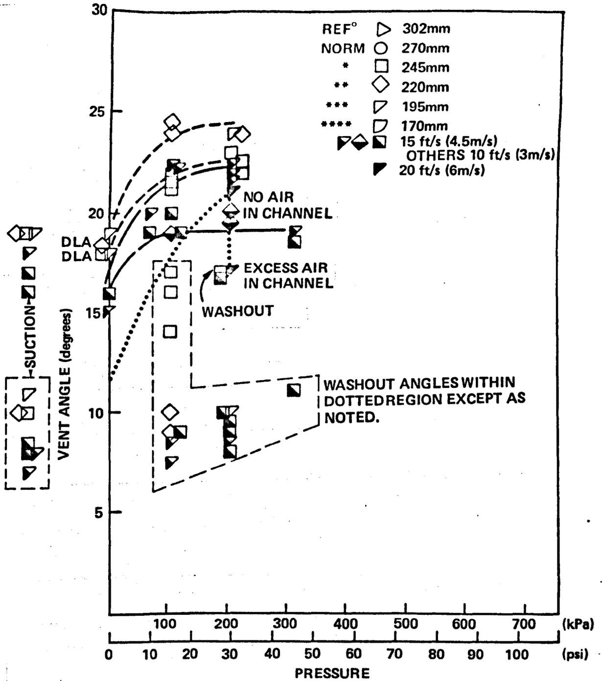
Figure 10.15 – Ventilation Angle Versus Blowing Reservoir Pressure, NACA 16 021 Foil With Horizontal Slot, Roughened With 11 Grade Glass Microspheres.
