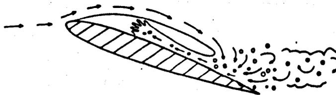
THE FROTHY RE-ENTRANT FLOW INTO THE BACK OF THE CAVITY THICKENS
