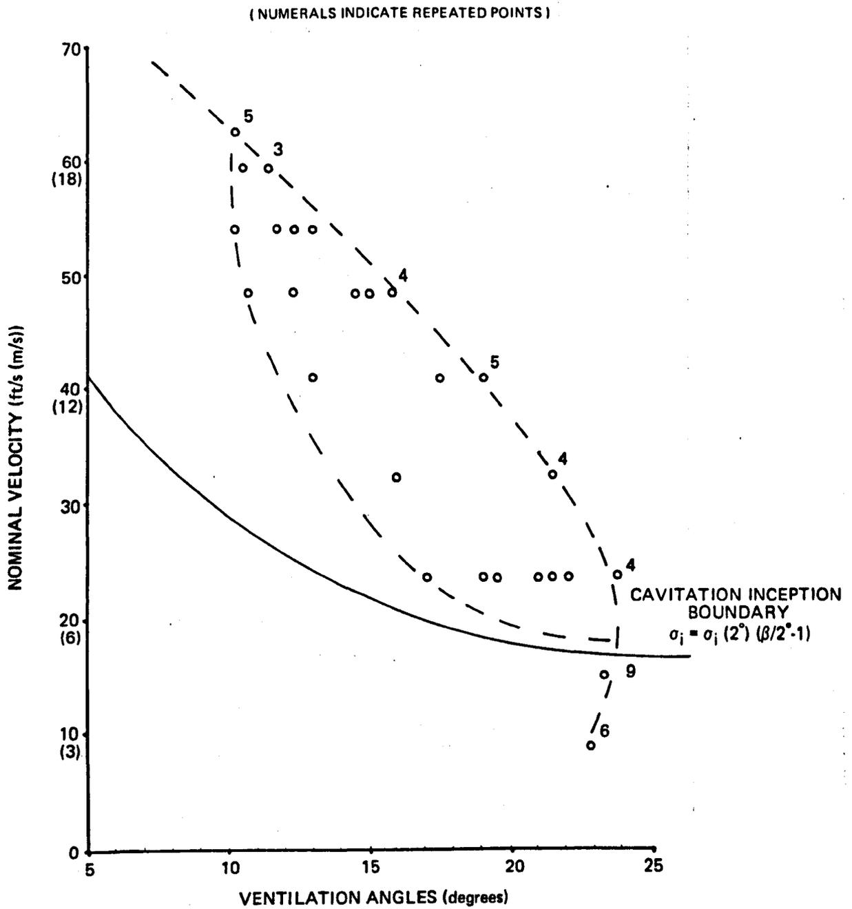
Figure 6.5 – Ventilation Angles vs Velocity NACA 0012 Foil.
