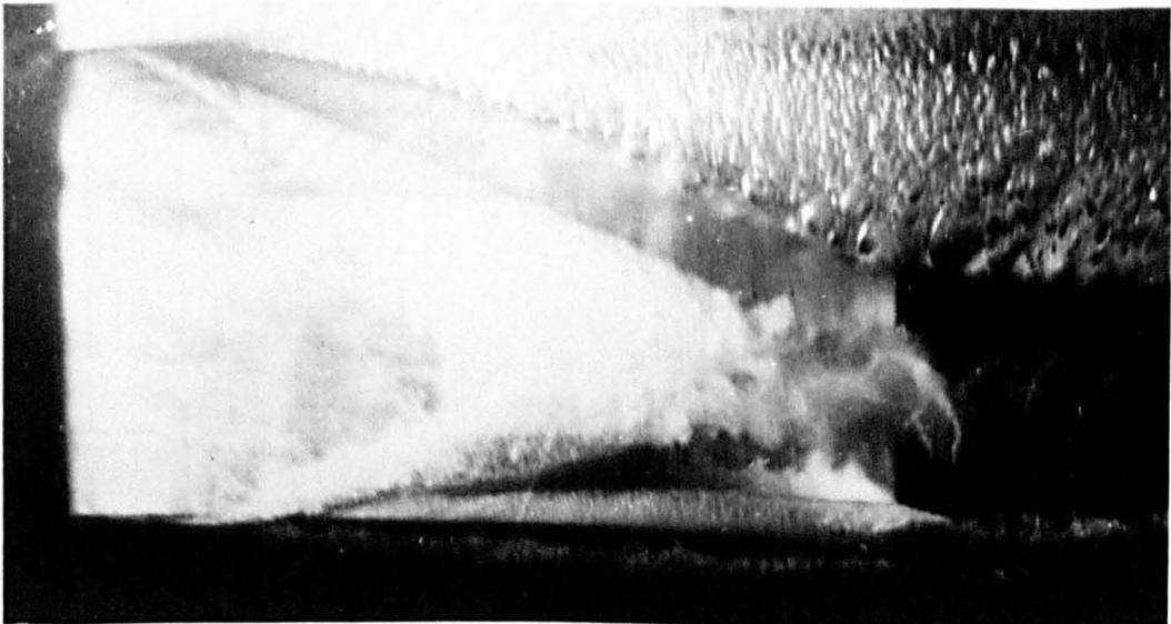
Figure 2.3b – Taylor Instabilities Photographed at the David W. Taylor Center Towing Tank at 55 kts (28 m/s), 600 mm chord model.
