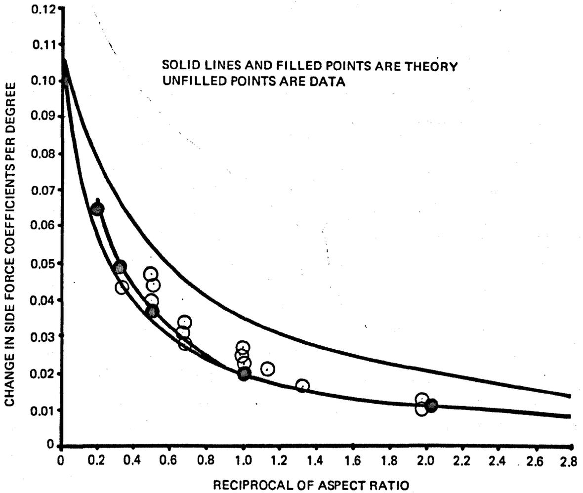
**Figure 7.6 – Sideforce Coefficient Slope Versus Reciprocal of Aspect Ratio.**
