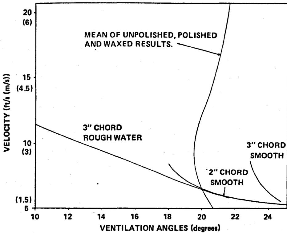
Figure 5.15 – Wetzel<sup>5.4</sup> Results with NACA 0012 Foil, in Smooth and Rough Water Compared to Results of Present Smooth Foil Tests.
