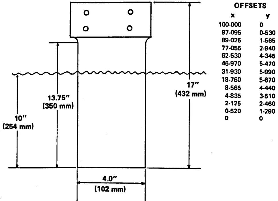
Figure 5.7 – NACA 0012 Struts, Mk I & Mk II, Nominal Planform Dimensions and Table of Offsets in Percent Chord.
