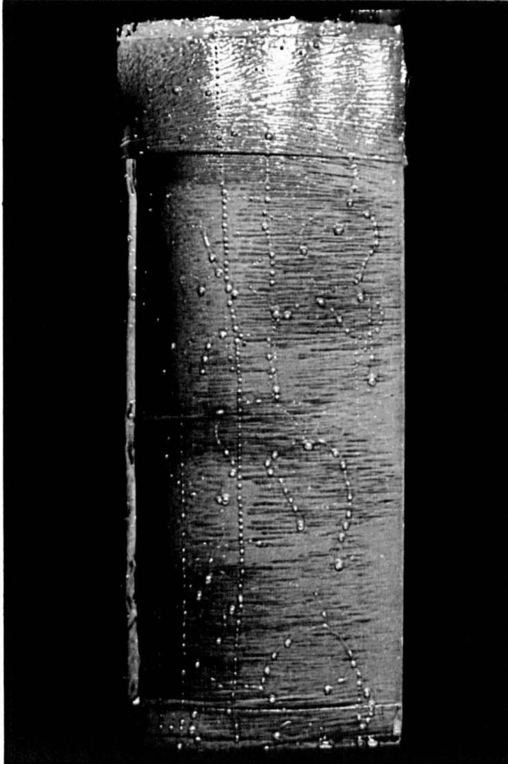
Figure 8.6 – Blunt Bio-give with Tape on Upper and Lower Part of Slot and Smoothed Leading Edge. 20 ft/s (6m/s),  $\beta = 0$  Degrees, Maximum Suction.
