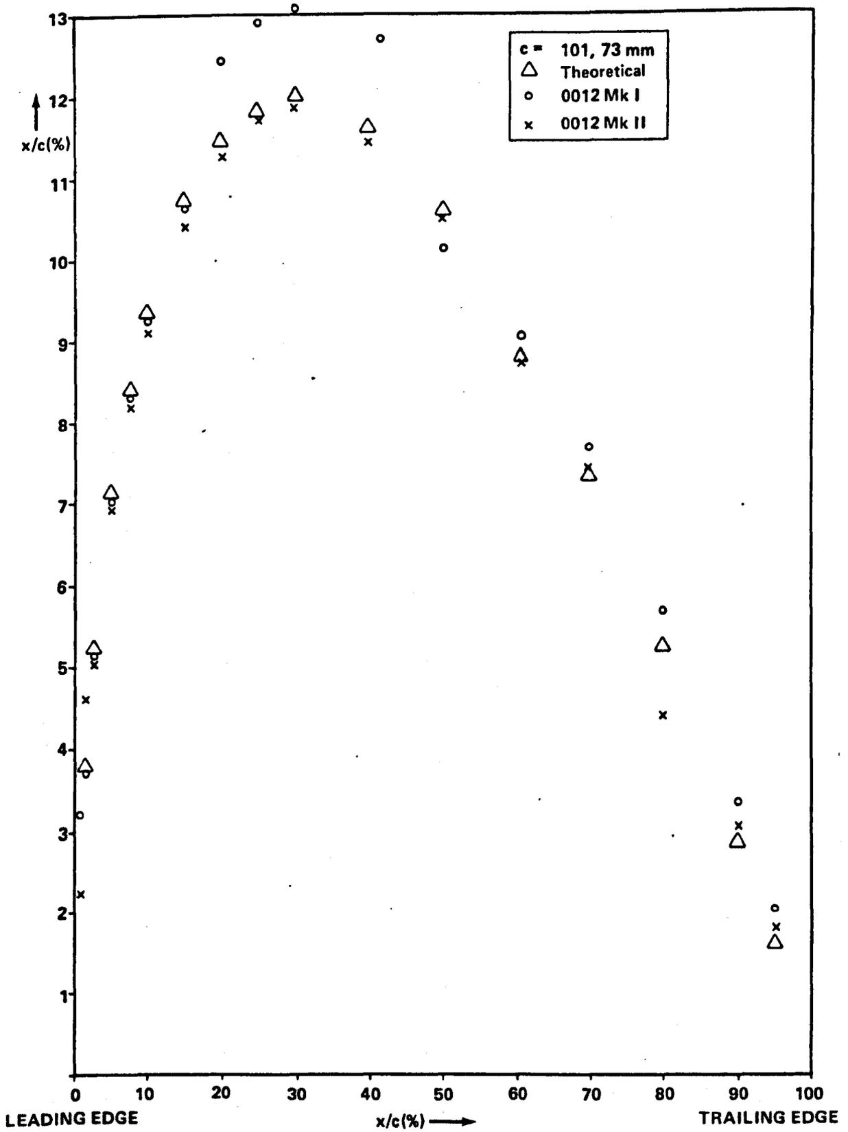
Figure 5.8 — Theoretical and Measured Profiles of NACA 0012 Models Mk I & Mk II.
