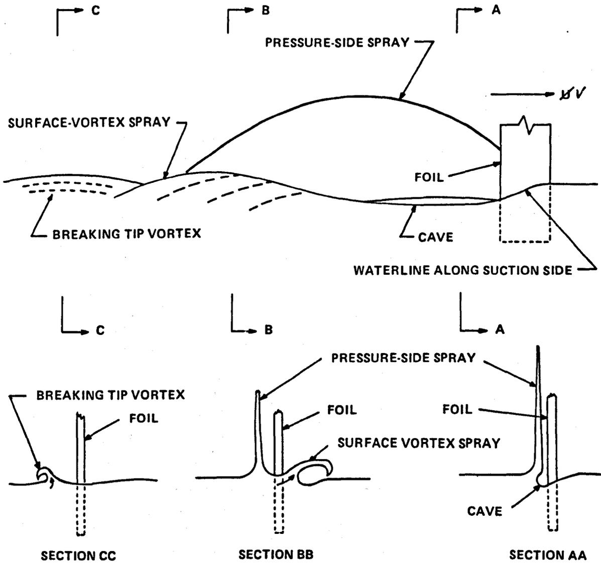
Figure 2.1(a) – Typical Flow Prior to Ventilation at High Froude Number, from Breslin and Skalak<sup>2,4</sup>.
