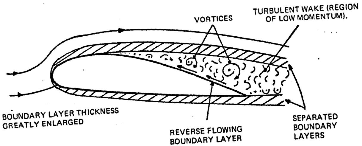
Figure 7.1 - Velocity Profiles and Physical Diagram of Separation on an Aerofoil.
