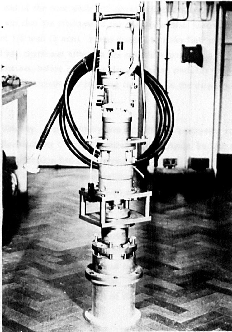
Figure 6.3 – Photograph of Rotation and Mounting Mechanism
