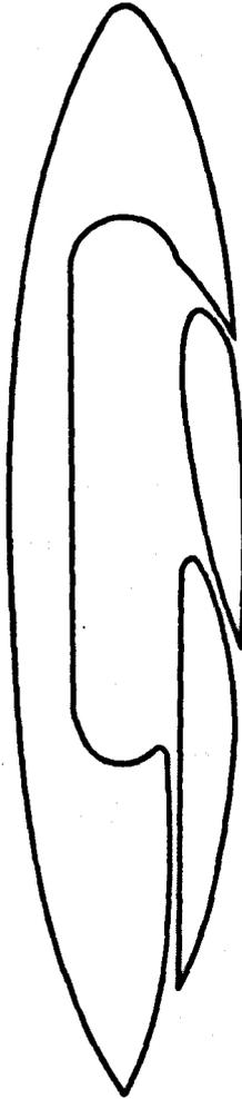
**Figure 9.5 – Modifications to the Slots to Encourage Uniform Flow.**
