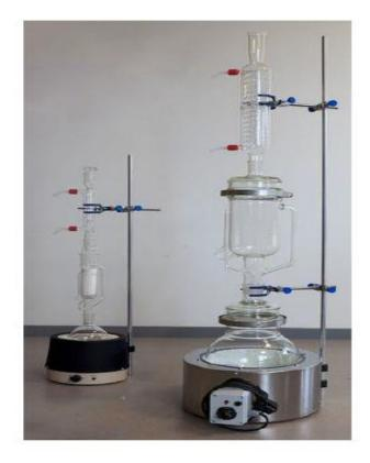
Figure 3.7 The Dean stark distillation apparatus for sample cleaning (taken from vinci Tech catalogue).
