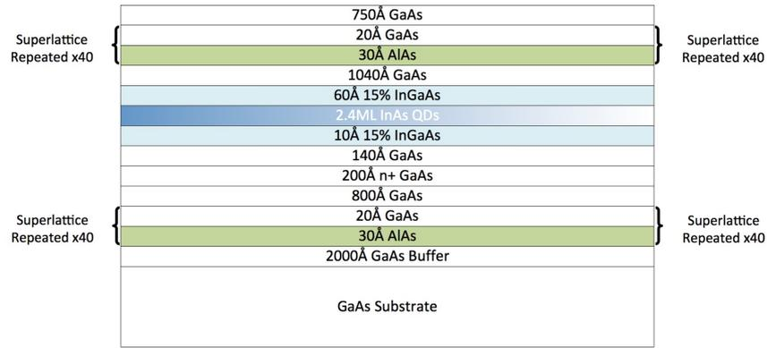
Figure 4.2.1: Schottky device structure, as grown for Heriot-Watt.
