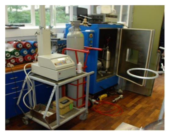
**Figure 7.4** Experimental set up. In the foreground, CO<sub>2</sub> bottle and ISCO pump. In the background, oven where the core holder and a container filled with CO<sub>2</sub>-saturated water are placed during the experiment.
