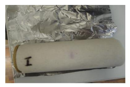
Figure 6.4 Hopeman sandstone disc and Lochaline core montage (with the lead foil unwrapped) used in the experiment.
