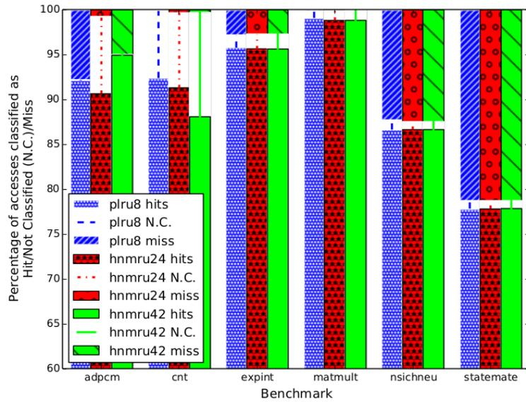
Figure 4.21: Comparison of the analysable performance of 8-way HNMRU and PLRU caches using the Mälardalen benchmarks
