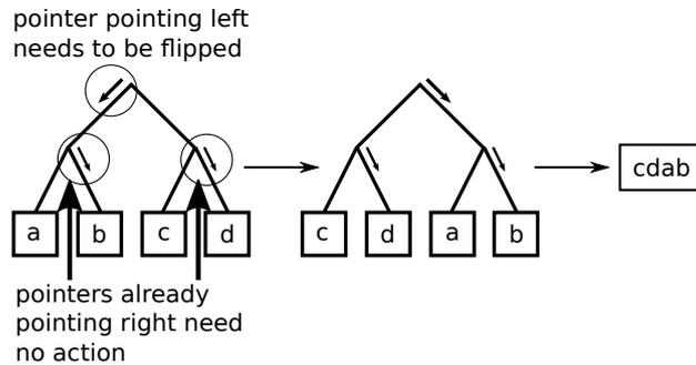
Figure 2.11: Assigning a name to a tree fill PLRU cache
