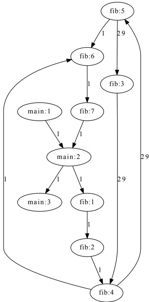
Figure 5.7: An annotated CFG for the `fibcall.c` benchmark. Labels on nodes are of the form “*function name:basic block number*”, and labels on edges denote the maximum number of times that edge may be taken.
