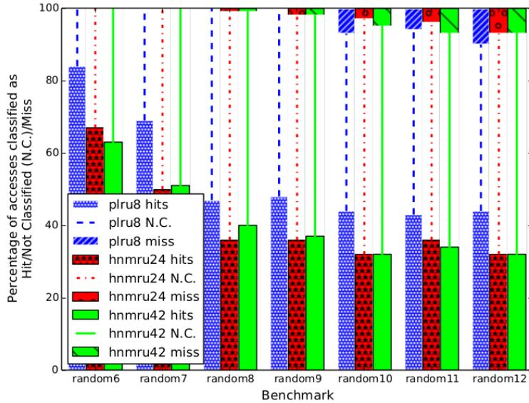
Figure 4.20: Comparison of the analysable performance of 8-way HNMRU and PLRU caches using the random benchmark
