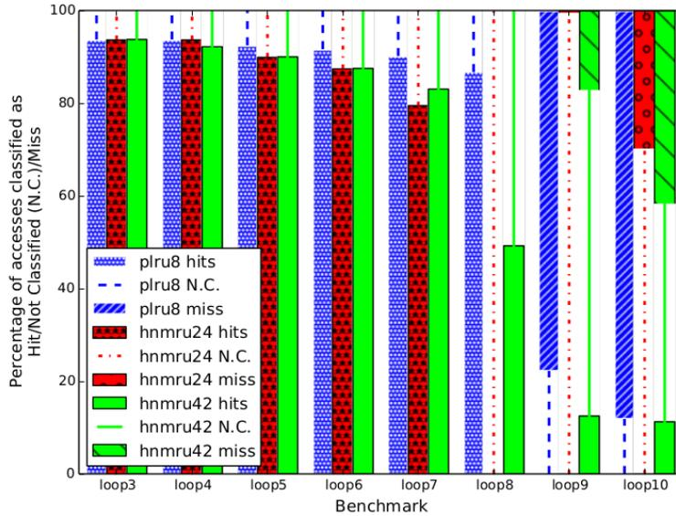
Figure 4.19: Comparison of the analysable performance of 8-way HNMRU and PLRU caches using the loop benchmark
