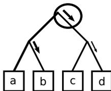
Figure 2.10: As an access to  $a$  sets the circled pointer,  $b$  can be unintentionally protected
