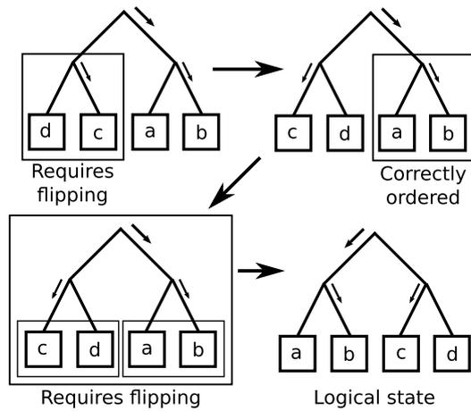
Figure 4.4: Illustrating how to find a cache signature, using alphabetical comparison, by moving from a physical state to an appropriate logical state without using pointers
