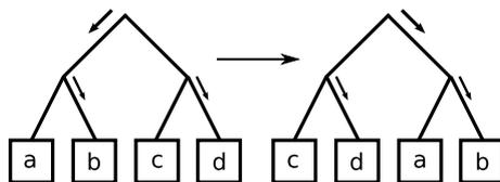
Figure 4.1: Putting all pointers to the right results in assigning a name to the logical state of a cache
