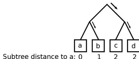
Figure 3.5: Subtree distances to element  $a$  in a 4-way cache
