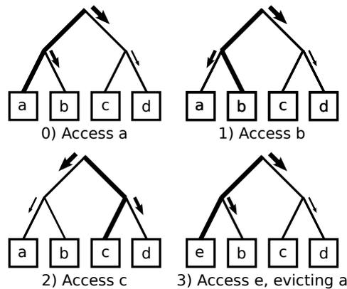
Figure 2.9: Illustrating the fastest a memory location can be evicted from a PLRU cache
