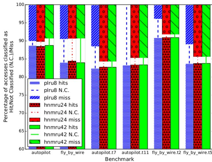
Figure 4.22: Comparison of the analysable performance of 8-way HNMRU and PLRU caches using the Papabench benchmarks
