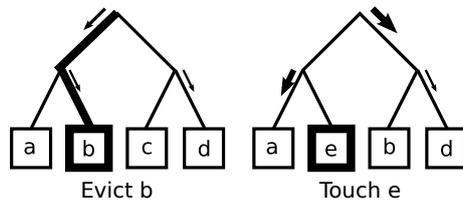
Figure 2.8: Showing the behaviours of a PLRU cache by demonstrating a cache eviction
