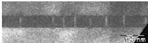
Figure 1.5: TEM image of quantum rods normal to growth direction. Image taken from Ref. 1.
