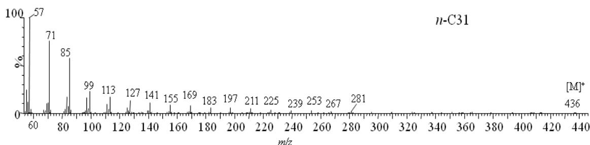
Figure 3.5: Example of an *n*-alkane (*n*-C31) mass spectrum.
