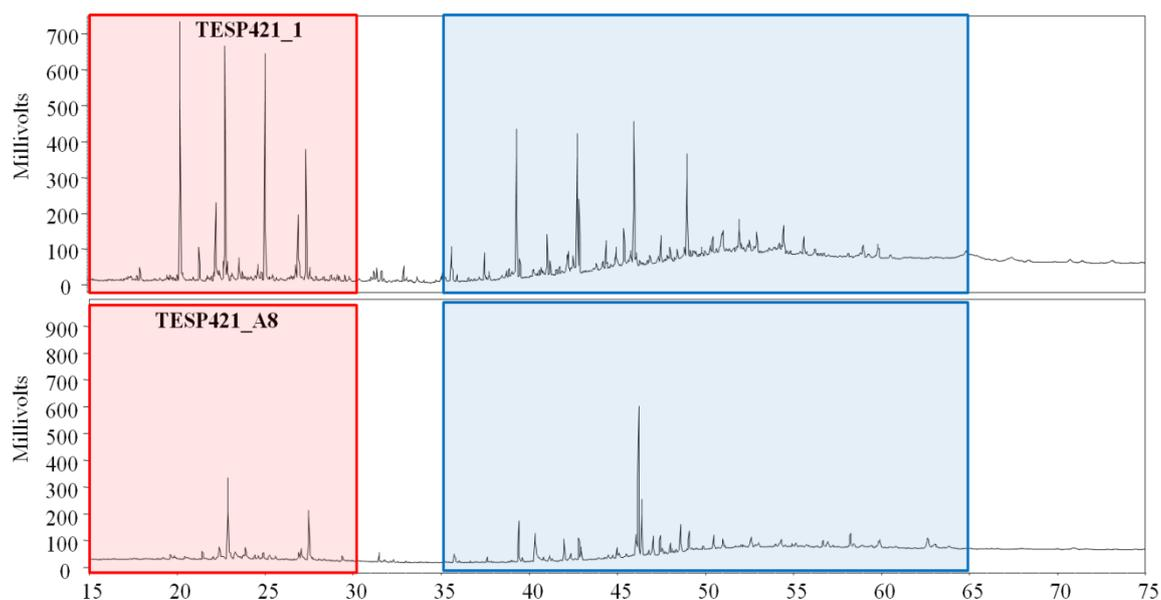
Figure 5.23: Partial GC-FID chromatogram from a) the skull (1), which represents the typical profile from all soils samples collected and b) from the bone sample (A8), which typifies the bone samples collected. The area highlighted in red shows the LMW components and the area highlighted in blue represents the HMW components. Originally in colour.
