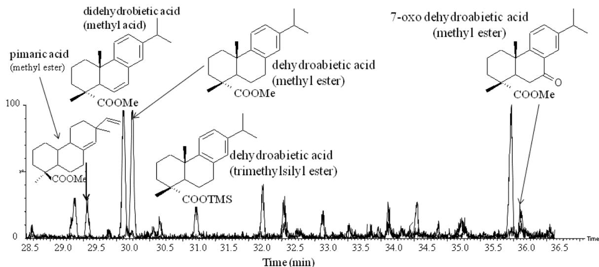
Figure 5.7: Combined partial mass chromatograms extracted for  $m/z$  197 and  $m/z$  257.
