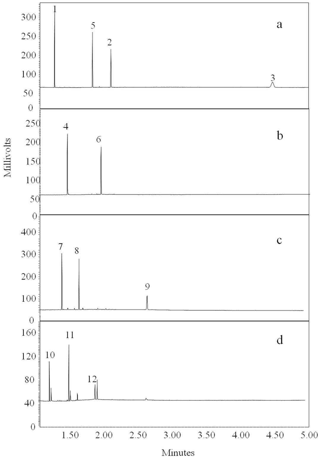
Figure 2.3: Partial fast GC-FID chromatograms of the various fractions collected from column chromatography of a mixture of standards: a) hydrocarbon fraction, b) aromatic fraction, c) medium polar fraction, d) high polar fraction. The peak numbers represent the standards discussed in Section 2.2.3.
