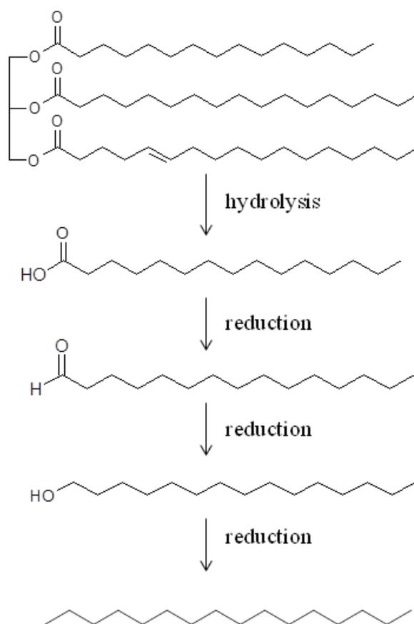
Figure 6.1: Putative pathway for the transformation of TAGs to *n*-alkanes, modified from Naccarato *et al.* (1972) where the reduction of tracer fatty acids to alcohols in the presence of a cell-free preparation of *E coli* and Day, (1978), where the biosynthesis of *n*-alkanals and alkanols by the bacterium *Clostridium butyricum* are discussed.
