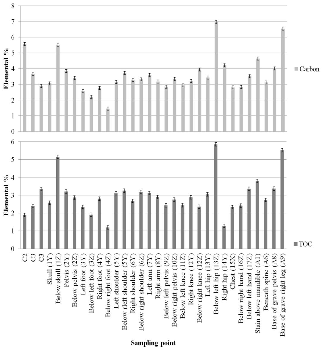
Figure 5.3: Bulk carbon, nitrogen and total organic carbon (TOC) elemental analyses of soil samples from HSM-11-116. Error bars represent  $\pm 1$  standard deviation calculated from replicates of standards ( $n=4$ ).
