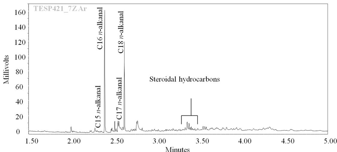
Figure 5.27: Partial GC-FID chromatogram of the aromatic fraction of the soil extract from sampling point 7Z, which represent the profile of all the soil extracts taken from TESP 421.
