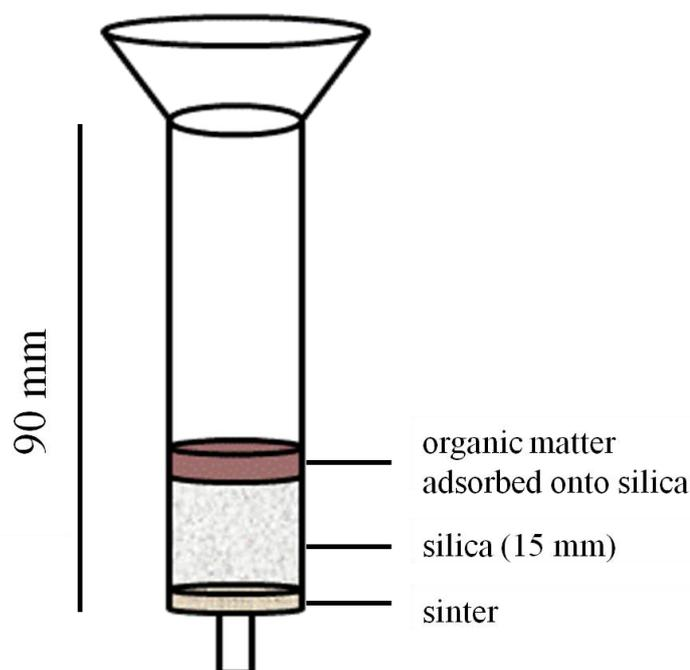
Figure 2.2: Schematic of column used for fractionation. Originally in colour.
