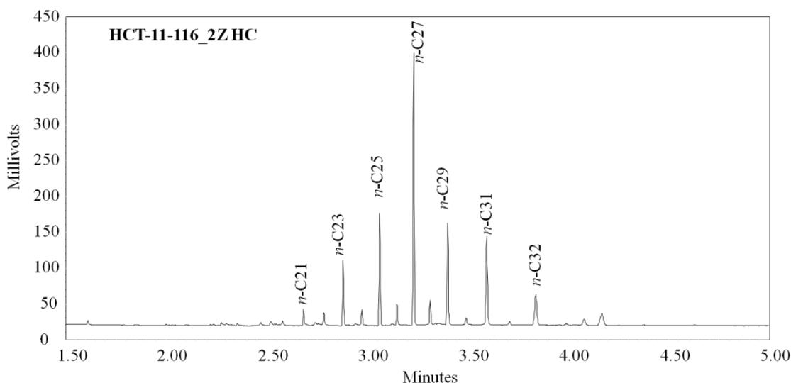
Figure 5.5: Partial GC-FID chromatogram of the hydrocarbon distribution from sampling point 2Z of grave HSM-11-116, which represents the hydrocarbon distribution from all of the sampling points.
