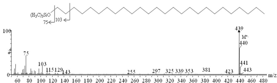
Figure 3.7: Example of an alcohol (C26) mass spectrum.
