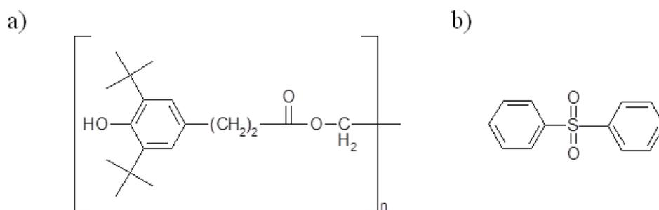
Figure 2.1: Example of plasticisers found in samples from the ASE; a) IRGANOX, b) diphenyl sulfone.
