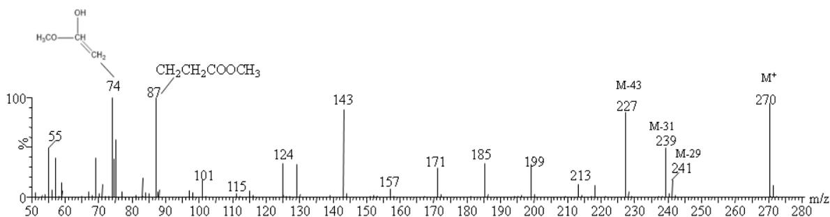
Figure 3.8: Example of an alkanone mass spectrum.
