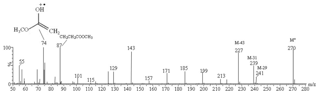
Figure 3.10: Example of a fatty acid mass spectrum (C16).
