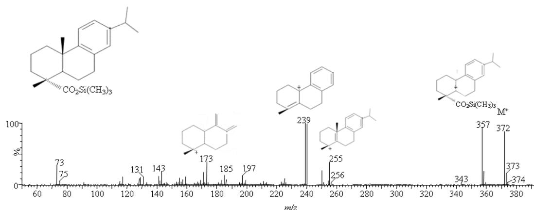
Figure 5.8: Mass spectrum of dehydroabiatic acid TMS showing diagnostic fragments.
