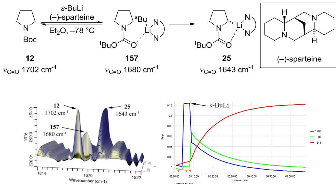
Scheme 2.15 *In situ* ReactIR<sup>TM</sup> spectroscopic monitoring of the lithiation of **12** with *s*-BuLi/(-)-sparteine.
