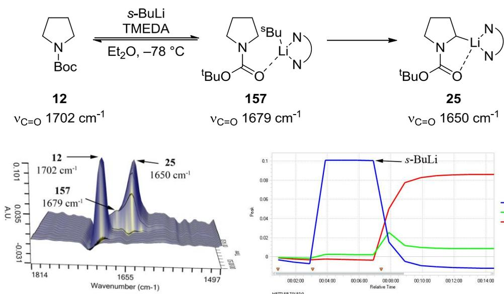
Scheme 2.14 *In situ* ReactIR<sup>TM</sup> spectroscopic monitoring of the lithiation of **12** with *s*-BuLi/TMEDA. The position of the arrow shows the time when the indicated reagent was added to the reaction mixture
