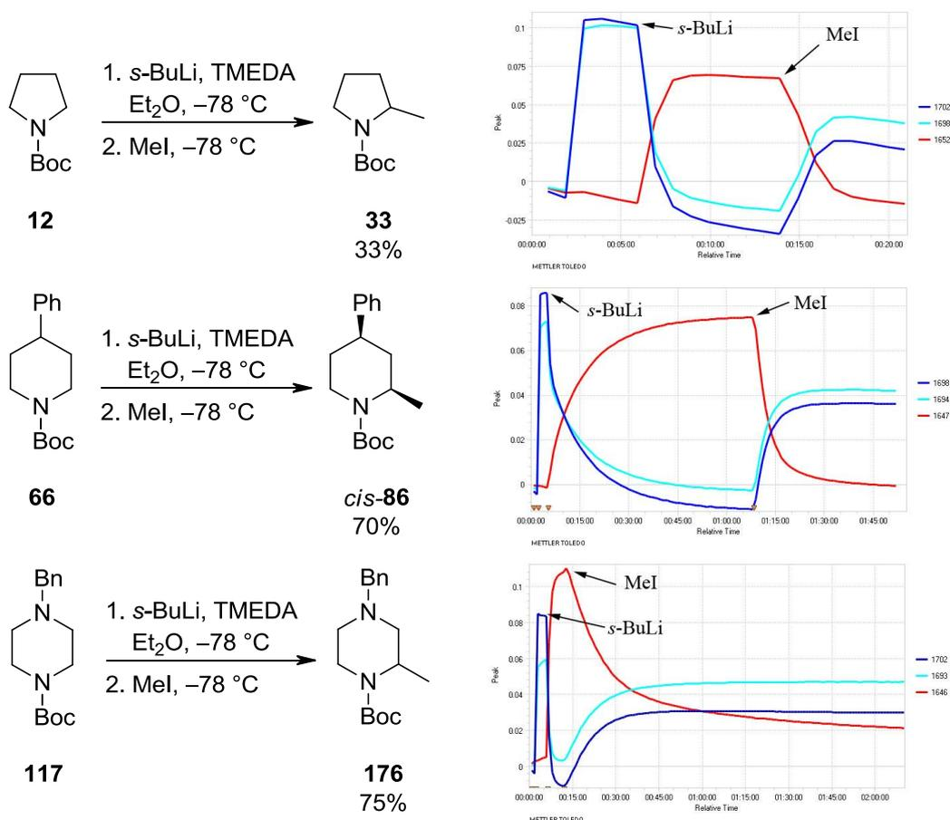
Scheme 2.29 *In situ* ReactIR<sup>TM</sup> spectroscopic monitoring of lithiation/trapping with *s*-BuLi/TMEDA and methyl iodide
