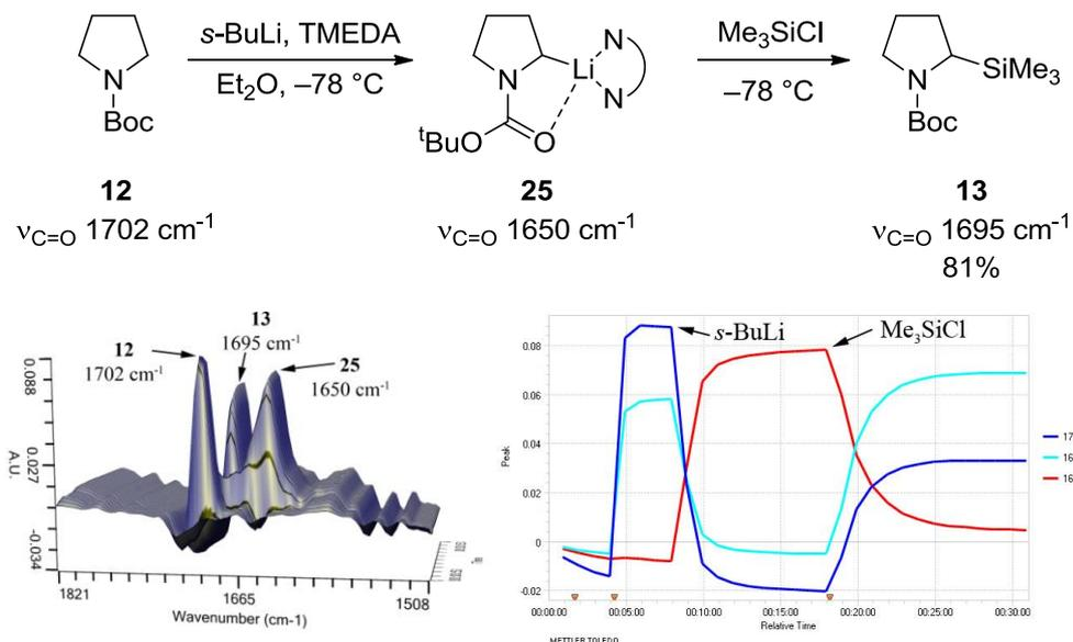
Scheme 2.25 *In situ* ReactIR<sup>TM</sup> spectroscopic monitoring of the lithiation/trapping of **12** with *s*-BuLi/TMEDA and  $\text{Me}_3\text{SiCl}$ . The position of the arrows show the time when the indicated reagents was added to the reaction mixture
