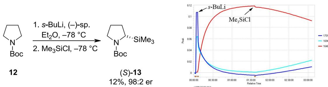
Scheme 2.31 *In situ* ReactIR<sup>TM</sup> spectroscopic monitoring of the lithiation/trapping of **12** with *s*-BuLi/(–)-sparteine and Me<sub>3</sub>SiCl at –78 °C
