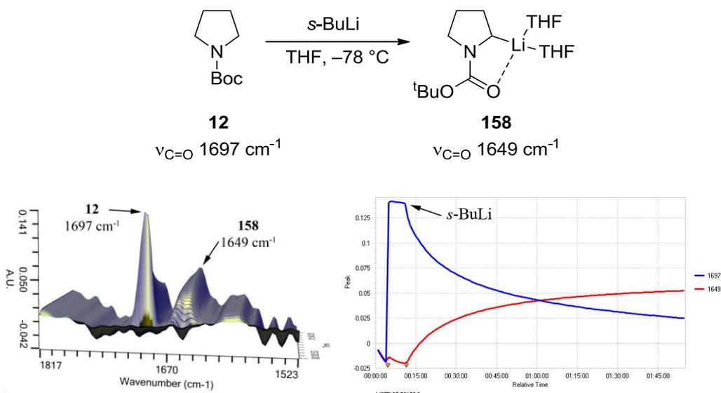
Scheme 2.17 *In situ* ReactIR™ spectroscopic monitoring of the lithiation of **12** with *s*-BuLi in THF
