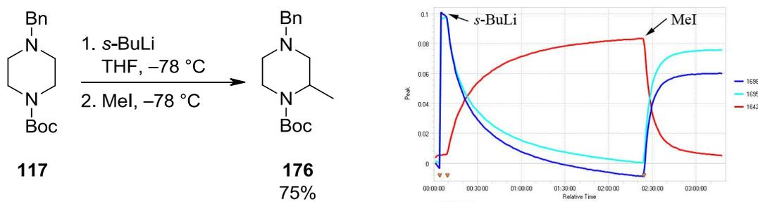
Scheme 2.30 *In situ* ReactIR<sup>TM</sup> spectroscopic monitoring of the lithiation/trapping of **117** with *s*-BuLi in THF and methyl iodide
