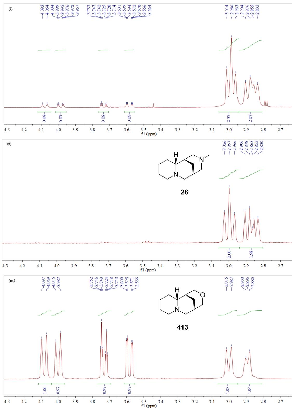
Figure 5.5  $^1\text{H}$  NMR spectra of i) 90:10 mixture of **26**:**413**, ii) sparteine surrogate **26** and iii) tetrahydropyran **413**
