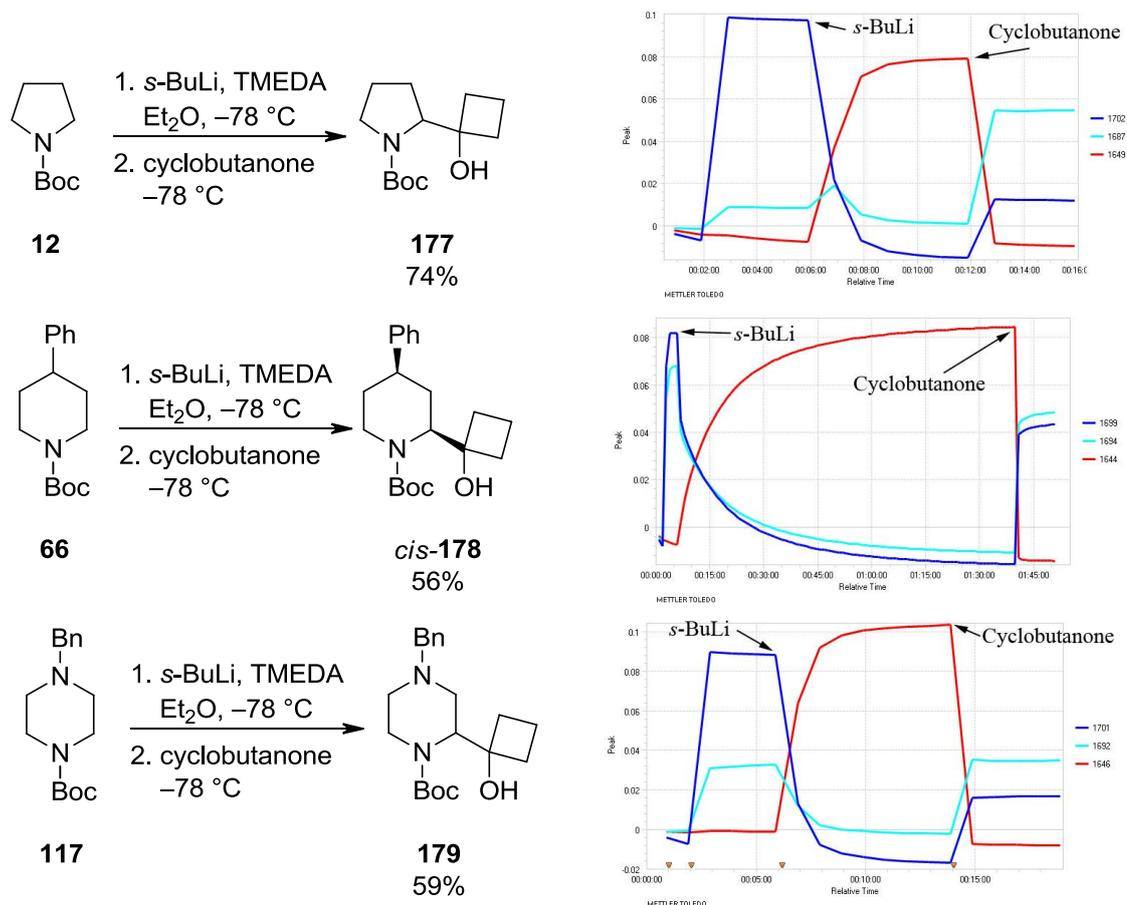
Scheme 2.33 *In situ* ReactIR<sup>™</sup> spectroscopic monitoring of lithiation/trapping with *s*-BuLi/TMEDA and cyclobutanone
