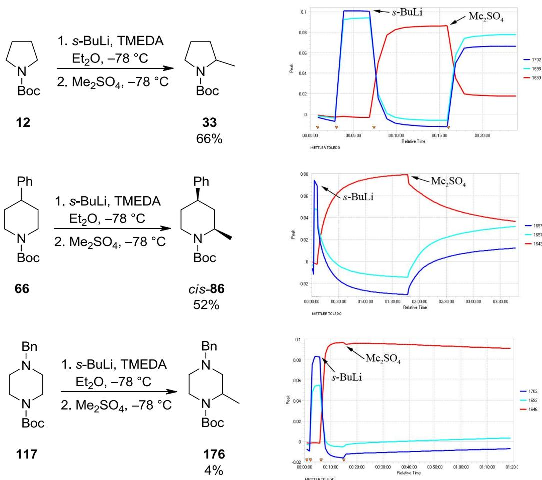
Scheme 2.28 *In situ* ReactIR<sup>™</sup> spectroscopic monitoring of lithiation/trapping with *s*-BuLi/TMEDA and dimethyl sulfate
