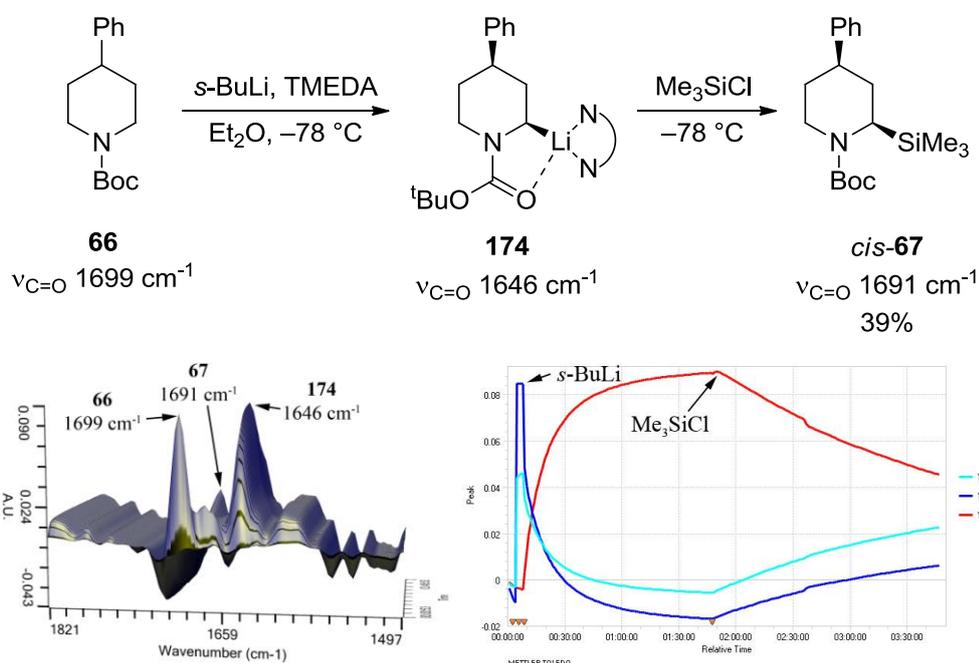
Scheme 2.26 *In situ* ReactIR<sup>TM</sup> spectroscopic monitoring of the lithiation/trapping of **66** with *s*-BuLi/TMEDA and  $\text{Me}_3\text{SiCl}$
