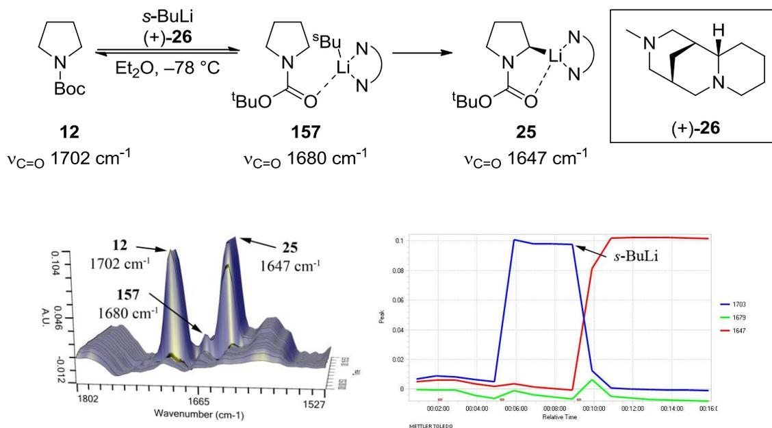
Scheme 2.16 *In situ* ReactIR<sup>TM</sup> spectroscopic monitoring of the lithiation of **12** with *s*-BuLi/(+)-sparteine surrogate (+)-**26**
