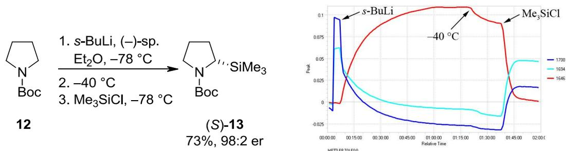
Scheme 2.32 *In situ* ReactIR<sup>TM</sup> spectroscopic monitoring of the lithiation of **12** with *s*-BuLi/(–)-sparteine at –78 °C and trapping with Me<sub>3</sub>SiCl at –40 °C
