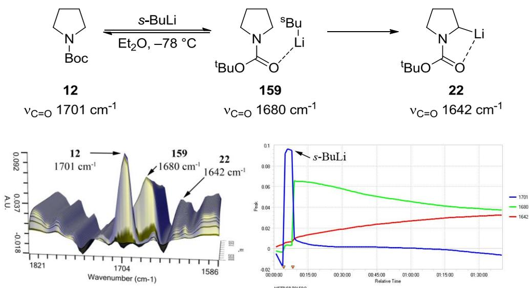
Scheme 2.18 *In situ* ReactIR<sup>TM</sup> spectroscopic monitoring of the lithiation of **12** with *s*-BuLi in Et<sub>2</sub>O
