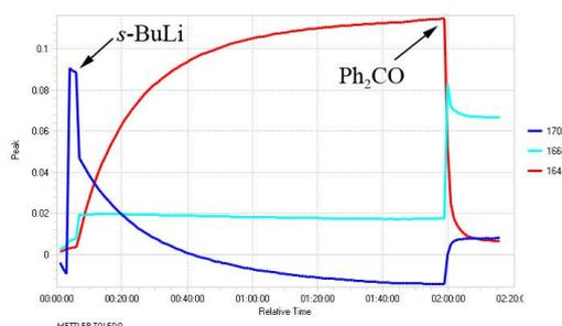
Scheme 2.38 *In situ* ReactIR<sup>TM</sup> spectroscopic monitoring of the lithiation/trapping of **117** with *s*-BuLi/(-)-sparteine and benzophenone
