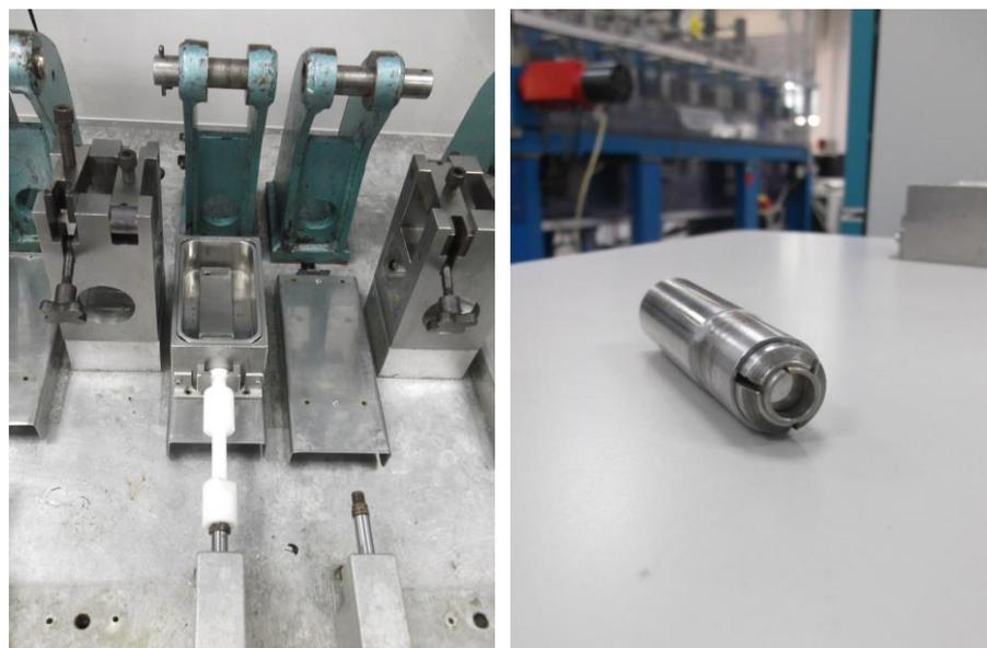
**Figure 3.7. The plate set up and pin holding assembly. A.** The bath well, bath insert and plate were assembled before being placed onto the reciprocating stage. The assembly was then secured with the connecting rod. **B.** The osteochondral pin was placed inside the set up shown with the cartilage surface protruding.
