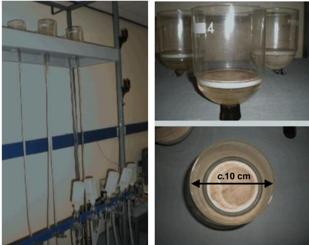
**Figure 3.21** Hanging water columns used for determining water retention of the soil cores collected from Birnie Hill (left image).
