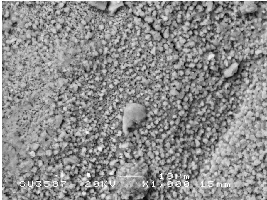
Figure A. 35 SEM BEI of the surface of aluminium encapsulated in CAP 2 for 180 days (x1000)
