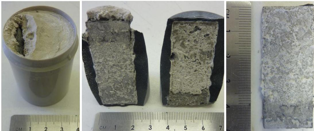
**(c) 360 days**
