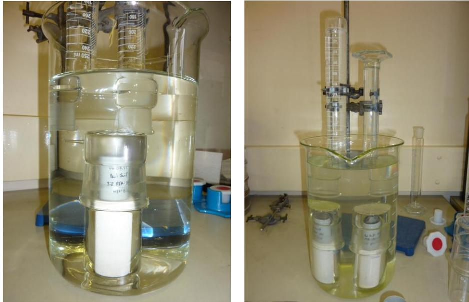
Figure 3.5 Photos of water displacement experimental setup for measuring hydrogen gas generation
