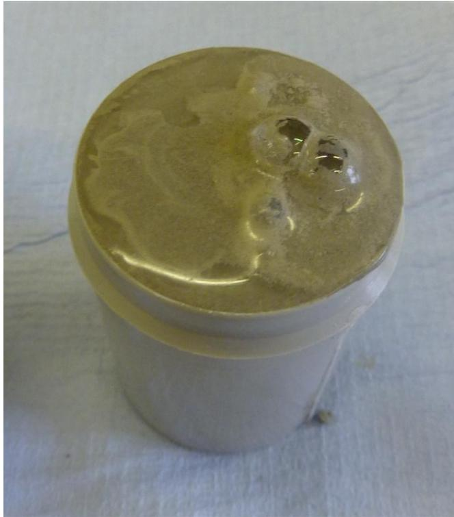
**Figure 6.3 Gas bubbles formed from aluminium encapsulated in BFS/PC**
