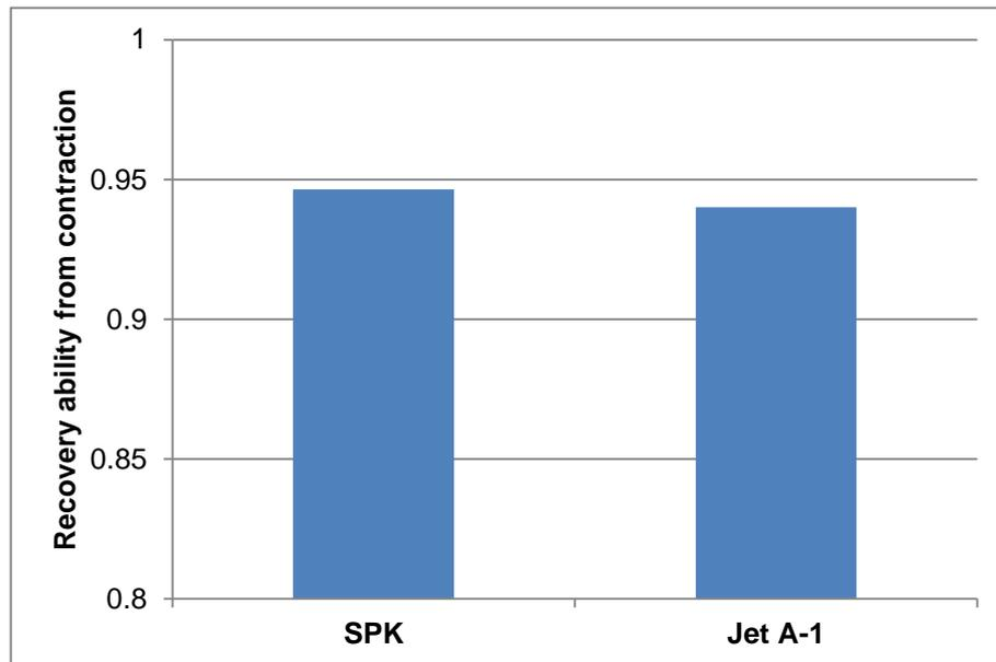
**Figure 121** Average recovery ability of fluorosilicone O-rings in Jet A-1 and SPK during the 24h-cycle testing without grooves.
