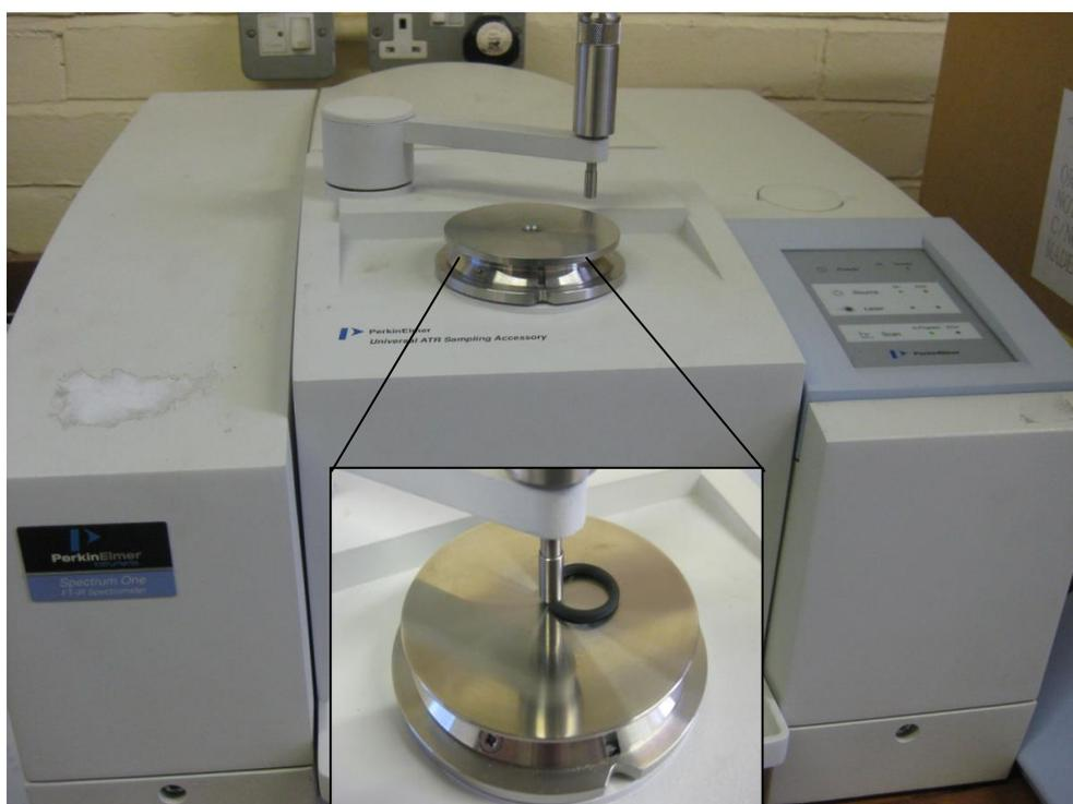
**Figure 35** Perkin-Elmer Spectrum One FTIR spectrometer with ATR accessory.
