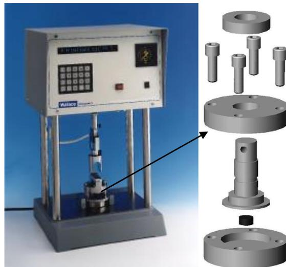
**Figure 23** A discontinuous stress relaxation test rig [53]
