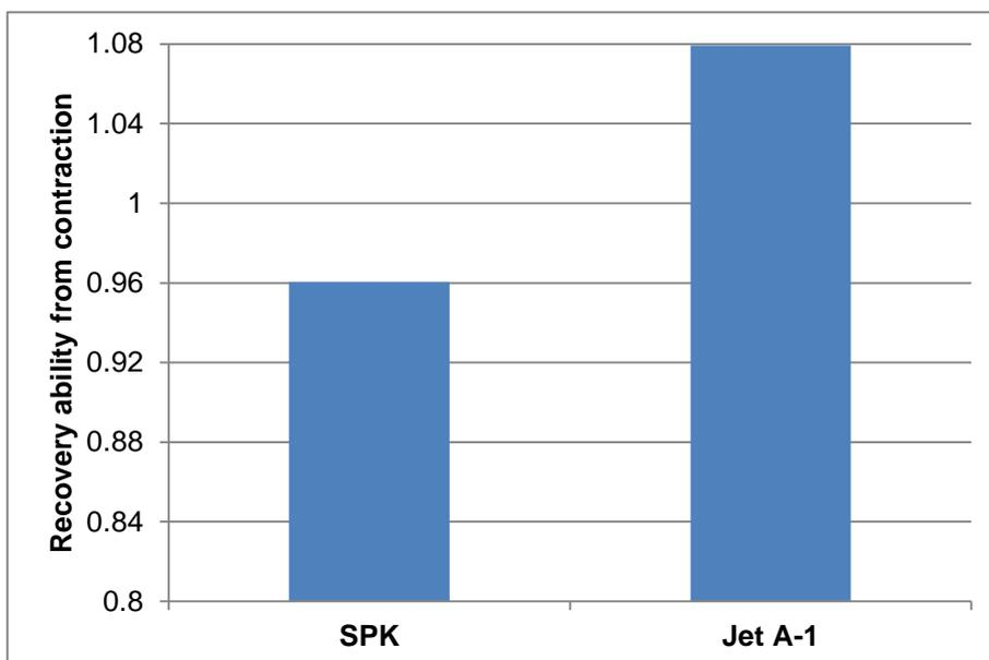
**Figure 113** Average recovery ability of fresh nitrile O-rings in Jet A-1 and SPK during the 24h-cycle testing without grooves.
