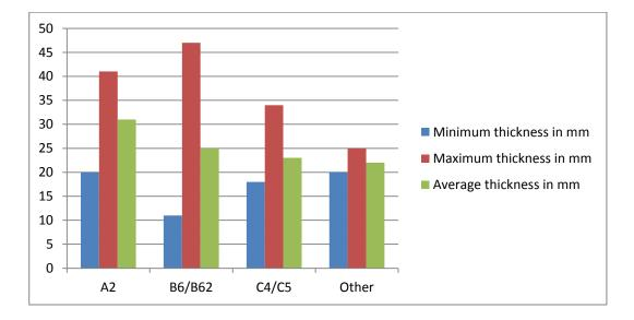
Figure 5. Maximum, minimum and average thickness of tegulae in mm in relation to lower cutaway forms (associated data in Table 29).
