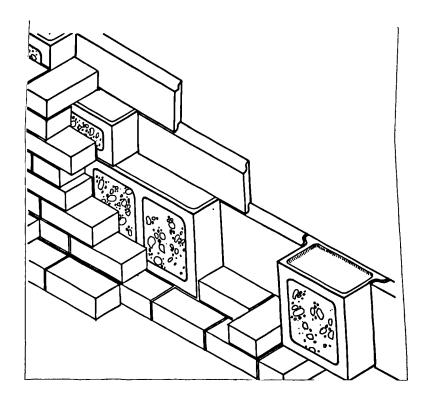
Figure 11.16. Filled terra cotta blocks bonded into the structural brickwork at the Natural History Museum, London, completed 1881. [From John Olley and Caroline Wilson, <u>Architects Journal</u> (1985) p.41]
