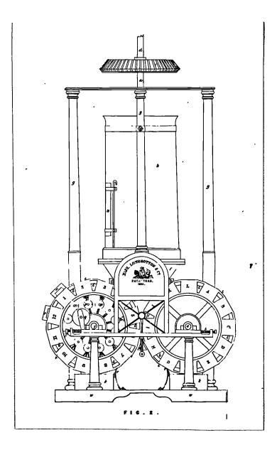
Figure 4.4. Vertical wheel moulding machine, British Patent No.6257, 1832, John J. Clark, John Nash and John Longbottom. [Drawing enrolled with patent]
