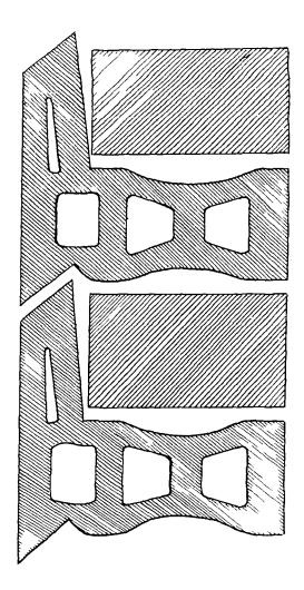
Figure 11.9. Interlocking facing bricks patented by W. Walton, British Patent No. 1093, 1861. [Adapted from drawing enrolled with patent]
