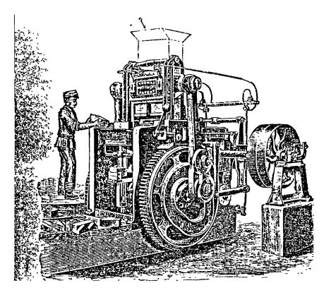
Figure 7.15. Semi-dry brickmaking machine manufactured by Christopher Whittaker and Company, Accrington, c.1890. [From M. Powis Bale, <u>The Building News</u> (1890) p.443]
