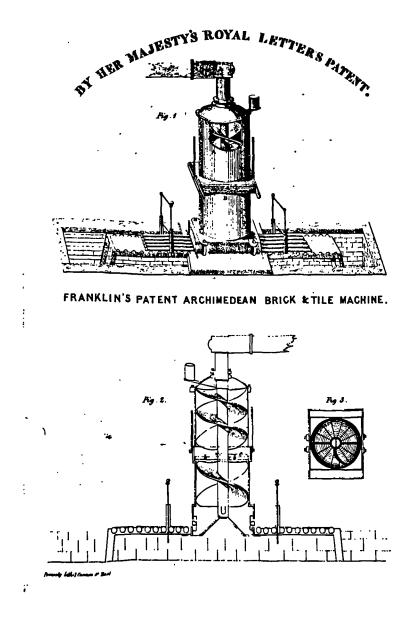
Figure 5.3. Franklin's Patent Archimedean Brick and Tile Machine [From Henry Franklin Trade Catalogue, 1847]
