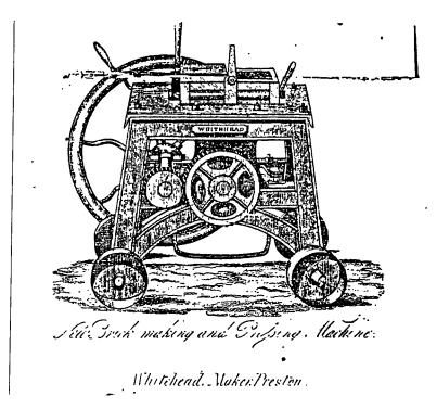
Figure 4.9. Brickmaking and pressing machine, John Whitehead, manufacturer. [From John Whitehead's Trade Catalogue, 1851]
