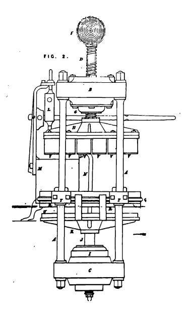
Figure 4.8. Hydraulic brick press by William Mencke, British Patent No.5681, 1828. [Drawing enrolled with patent]
