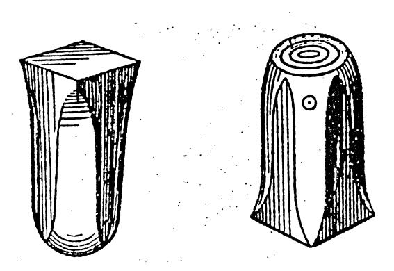
Figure 9.4. Hollow clay pots used in England for vaulting at the end of the eighteenth century. [From S.B. Hamilton, <u>Transactions of the British Ceramic Society</u> (1958) p.42, after C.W. Pasley, <u>Outline of a Course of Practical</u> <u>Architecture</u> (1826) p.178] Figure 9.5. Hollow pots used by William Strutt in a roof at Belper. [From S.B. Hamilton, <u>A Short History of the Structural Fire</u> <u>Protection of Buildings Particularly in England</u> (1958) plate 1]
