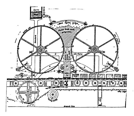
Figure 5.5. Hunt's improvement on Tweeddale's brickmaking machine, British Patent No.9243, 1842. [Drawing enrolled with patent]
