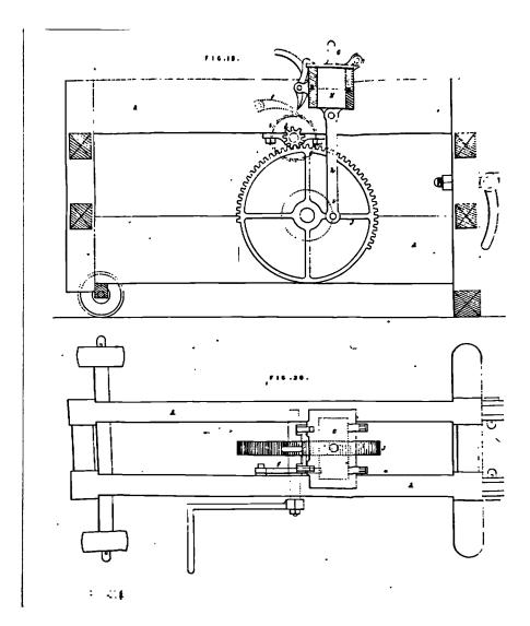
Figure 4.6. Brick press by Samuel Roscoe Bakewell, British Patent No.5985, 1830. Top, side view; Bottom, top view. [Drawing enrolled with patent]
