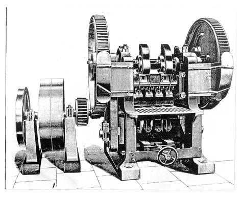
Figure 7.16. Johnson's Patent "Universal" Moulding and Pressing Machine. [From William Johnson, Armley, Leeds trade catalogue, 1894]
