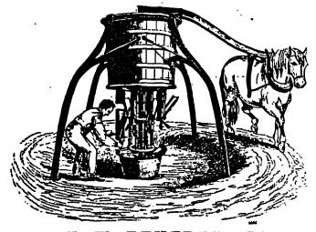
F. W. ETHEREDGE'S PUBORIEBO WITH NHA PATENT TILE-MAKING APPARATUS ATTACHED THERETO, AS SEEN WHEN AT WORK.
