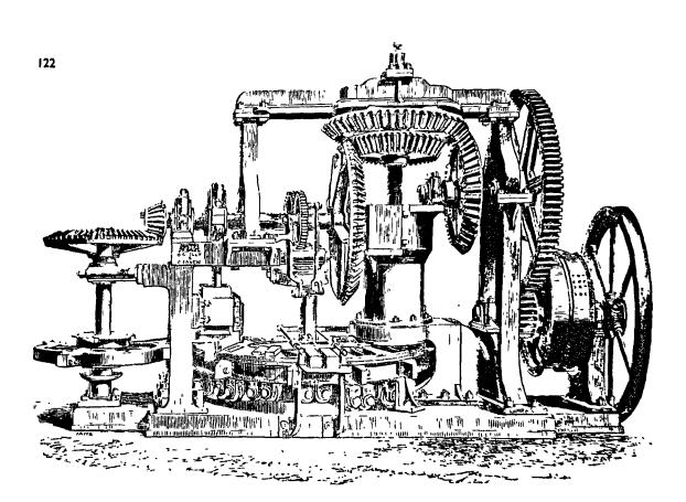
Figure 7.14. Bradley and Craven's semi-dry brick moulding and pressing machine, c. 1862. [From Bradley and Craven, Limited, <u>The First Hundred Years</u> (1963) p.80 and John Woodforde, <u>Bricks to Build a House</u> (1976)]
