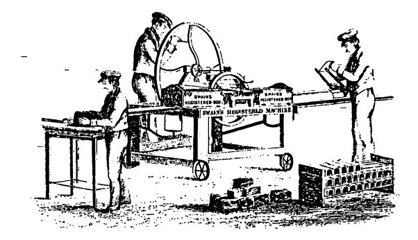
Figure 5.11. "Swain's Registered Pipe and Tile Machine", c.1847. [From trade card, c.1847]
