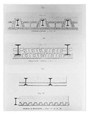
Figure 11.6. Patented fireproof flooring systems. Top, by Lewis Hornblower; middle, by Doulton and Peto; bottom, by Homan and Rogers. [From S.B. Hamilton, <u>A Short History of the Structural Fire</u> <u>Protection of Buildings, Particularly in England</u> (1958)] Figure 11.7. Johnson's hollow building bricks, British Patent No. 3622, 1869.
