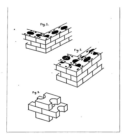
Figure 9.10. Beedle and Rogers ventilating bricks. [From Edward Dobson, <u>A Rudimentary Treatise on the Manufacture of</u> <u>Bricks and Tiles</u> (1850) p.35]
