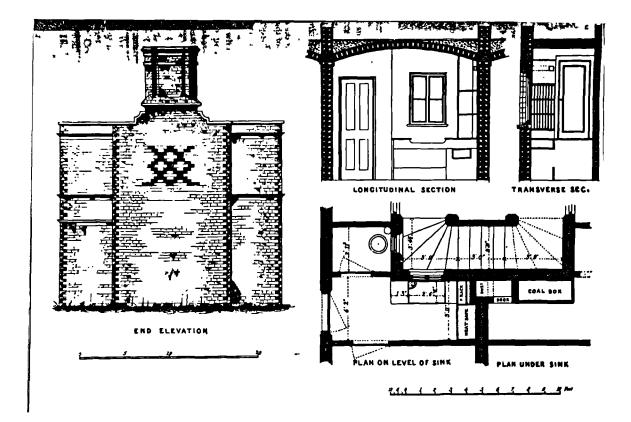
Figure 10.4. Prince Albert's Model Houses for Families at the Great Exhibition, 1851; end elevation, longitudinal and transverse sections, and detailed plan around common stair. [From James Steven Curl, <u>The Life and Work of Henry Roberts, 1803-1876</u> (1983) p.95] Figure 10.5. Prince Albert's Model Houses for Families at the Great Exhibition, 1851; section showing the floor and roof arches. [From Henry Roberts, <u>The Dwellings of the Labouring Classes</u> (1853) p. 34]
