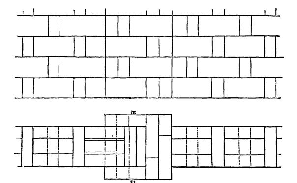
Figure 11.2. Plan and elevation of Silverlock's hollow walls. [From J.C. Loudon, <u>Encyclopedia of Cottage</u>, Farm, and Villa <u>Architecture</u> (1839) p. 186]
