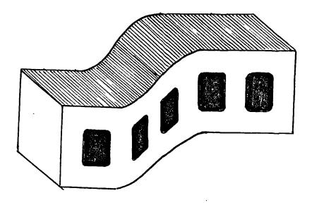
Figure 11.5. Hollow bonding bricks with modified S-curve designed by John Taylor. [From Rivington's <u>Notes on Building Construction</u> Part III (1879) p.135]
