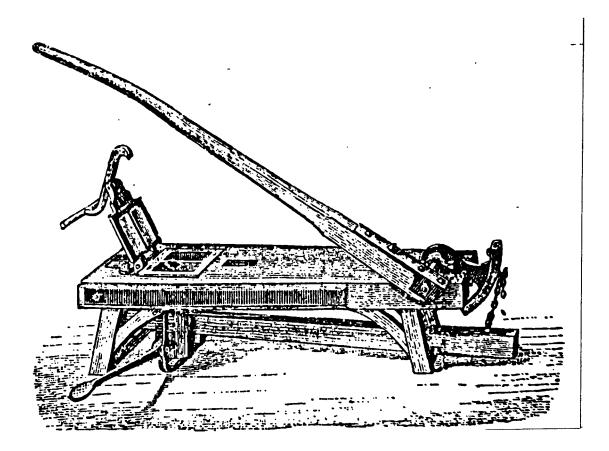
Figure 4.7. Early lever-operated brick press. [From Emile Bourry, <u>A Treatise on Ceramic Industries</u> (1901) p.288]
