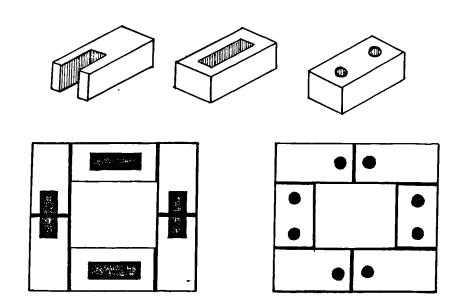
Figure 9.6. Benford Deacon's ventilating hollow bricks, British Patent No.3664, 1813. [Adapted from <u>The Building News</u> (1858) p.317] Figure 9.7. Hollow bricks for vaultings by Thunderer and Stellewerk of Vienna, c. 1841. [Adapted from <u>The Building News</u> (1858) p. 317]
