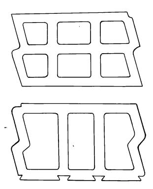
Figure 10.8. Interlocking hollow bricks for fire-proof floors and ceilings patented by J. Bunnett, British Patent No. 1292, 1859. [Adapted from drawing enrolled with patent] Figure 10.9. Section of machine-made hollow bricks used for arched fireproof flooring at Saltaire, c.1851. [Adapted from William Fairbairn, <u>The Application of Cast and</u> <u>Wrought Iron to Building Purposes</u> (1864) Plate III]
