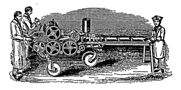
Figure 5.4. Tilemaking machine by the Marquess of Tweeddale, British Patent No. 7253, 1836. [From <u>The Builder</u> Vol. 1 1843, p. 195]
