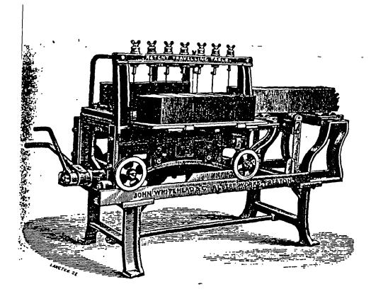
Figure 7.13. Travelling cutting table patented by J.D. Pinfold and manufactured by John Whitehead, c.1890. [From M. Powis Bale, <u>The Building News</u> (1890) p.301]
