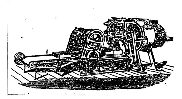
Figure 5.6. Brick and tile machine patented by John Ainslie, British Patent No.8965, 1841. [From <u>Civil Engineer and Architect's Journal</u> Vol.V 1842, p.427]
