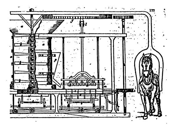
Figure 4.3. Brickmaking machine patented by Thomas Staniford (or Stainford) and George Henry Lyne, British Patent No.5246, 1825. [From Andrew Ure, <u>A Dictionary of Arts, Manufactures and Mines</u> (1835) p.186]
