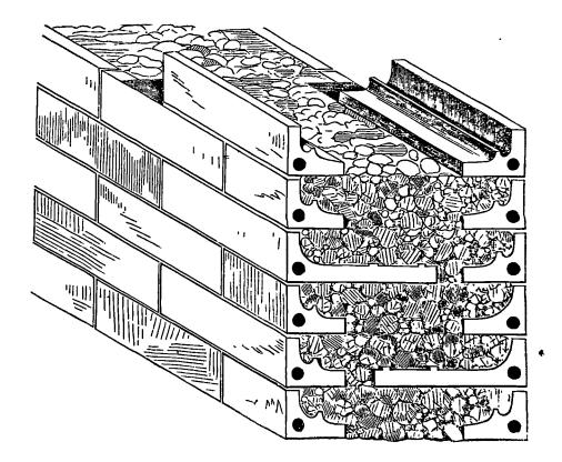
Figure 11.12. John Taylor's perforated facing bricks built into a concrete wall. [From John Taylor, Junior, <u>RIBA Papers, Etc.</u> (1863) p.86]
