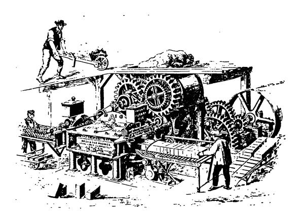
Figure 7.4. Henry Clayton's Universal "A 1" Combined Three-Process Brick Machine. [From Henry Clayton and Company trade catalogue c.1862] Figure 7.5. Extrusion brickmaking plant with three sets of crushing rolls, pug mill, die and cutting table. [From Alfred Searle, <u>Modern Brickmaking</u> (1931) p.138]
