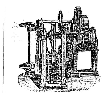
Figure 7.19. Stiff-plastic brickmaking machine by Bradley and Craven of Wakefield, c.1890. [From M. Powis Bale, <u>The Building News</u> (1890) p.443]
