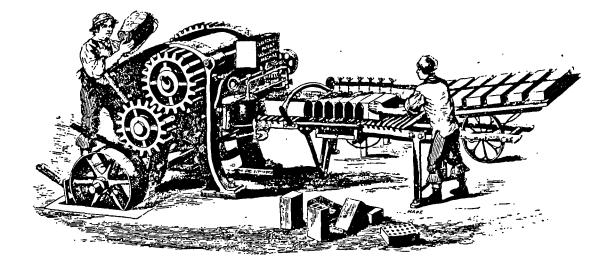
Figure 7.7. Henry Clayton's One-Process Brickmaking Machine. [From Henry Clayton, Son & Howlett, <u>Atlas Works</u> (1871) p.30]
