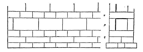
Figure 11.1. Dearn's method of building hollow walls; elevation and section of part of a wall. [From J.C. Loudon, <u>Encyclopedia of Cottage</u>, <u>Farm</u>, <u>and Villa</u> <u>Architecture</u> (1839) p. 168]
