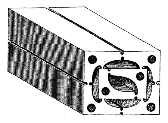
Figure 11.11. John Taylor's perforated facing bricks for bonding in with concrete; machine-extruded in one piece to prevent breakage, 1863.
