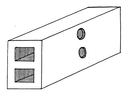
Figure 9.8. Hollow partition bricks patented in France by M. Collas, c.1842. [From <u>The Building News</u> (1858) p.318]
