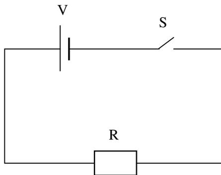
**Figure 1:** A simple circuit
