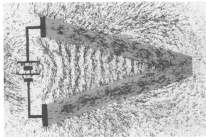
FIG. 2. Electric field of two intersecting straight conductors.
