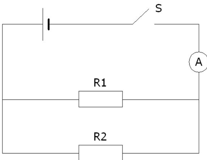
**Figure 5.4: Circuit diagram showing resistances connected in parallel**
