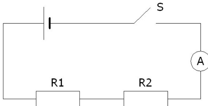
**Figure 5.3: Circuit diagram showing resistances connected in series**
