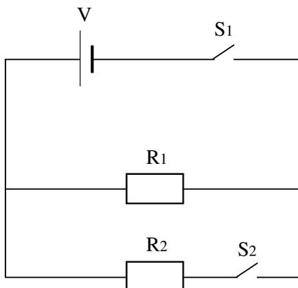
**Figure 3: A parallel circuit**
