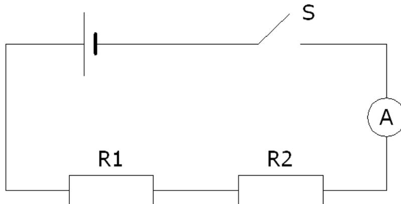
**Figure 2: A series circuit**
