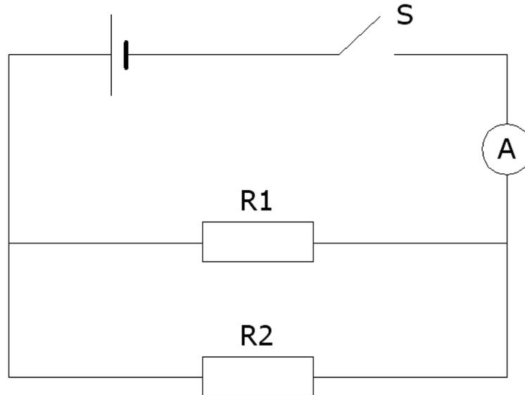
**Figure 3: A parallel circuit**
