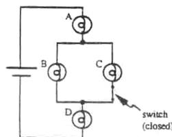
**Figure 2.7: Predicting the brightness of identical bulbs when the switch is closed (from McDermott and Shaffer, 1992, p. 998)**
