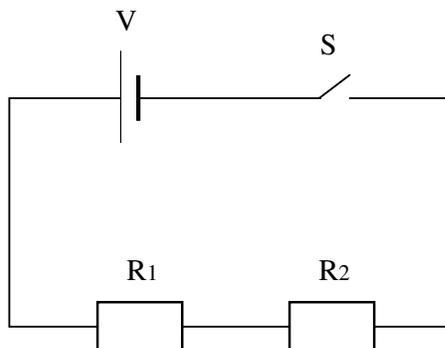
**Figure 2:** A series circuit
