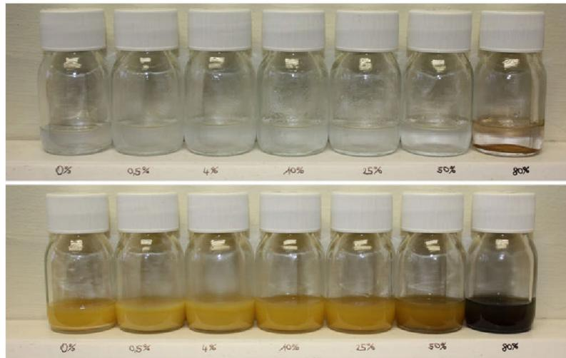
**Fig. 3** 1.3 %v/v aqueous H<sub>2</sub>SO<sub>4</sub> dispersed in C<sub>30</sub>H<sub>62</sub> (a) and HVI160B (b) after 72 h of settling. From left 0, 0.5, 4, 10, 25, 50 and 80 %w/w
