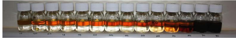
**Fig. 13** API Group I base oil HVI160B in contact with various concentrations of aqueous H<sub>2</sub>SO<sub>4</sub>, rising from 0 to 98 %w/w. From left: 0, 0.5, 1.5, 4, 10, 20, 30, 40, 50, 60, 70, 80, 90 and 98 %w/w
