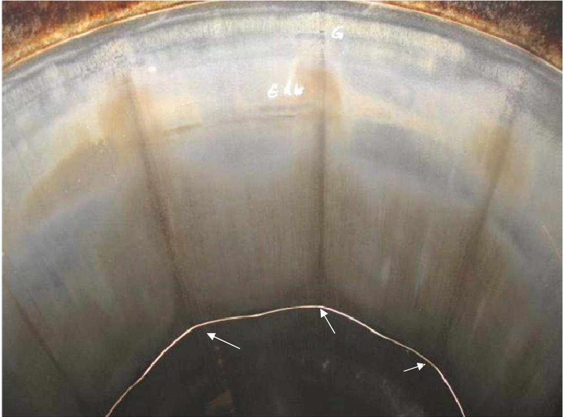
**Figure 1.8: Cylinder liner surface after 6293 running hours (Spahni, et al., 2010). Arrows indicate position of oil quills in the oil distribution groove, Figure 1.9**
