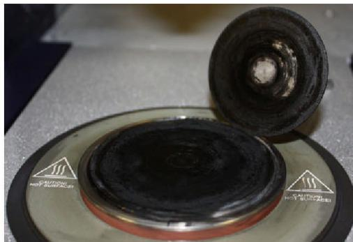
**Fig. 12** Solidification of bitumen formed between HVI160B and 98 %w/w  $H_2SO_4$  during viscosity measurements at 150 °C
