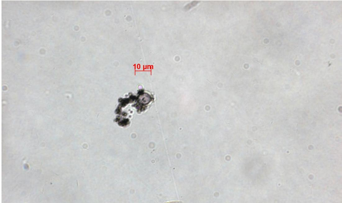
**Figure 3.3: Transmission microscopic image of the oil phase ( $C_{30}H_{62}$ ) on top of 80 %w/w  $H_2SO_4$  exposed to 165 °C**
