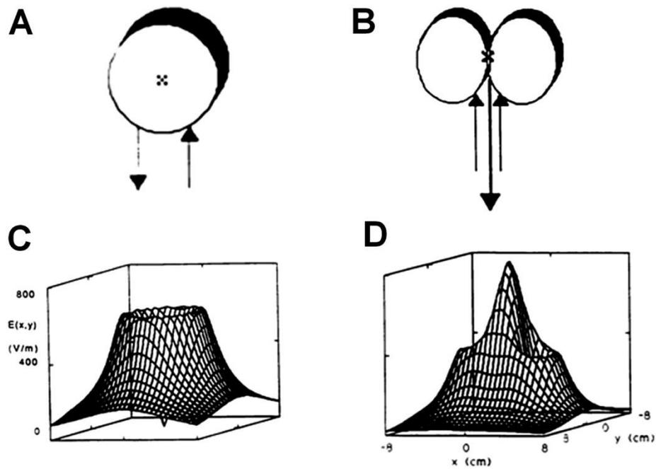
**Figure 3.3.** Electric fields produced by different magnetic coils. (A) Round coil and (C) resultant field. (B) Figure-8 coil and (D) resultant field. From Hallett (2007), with permission.
