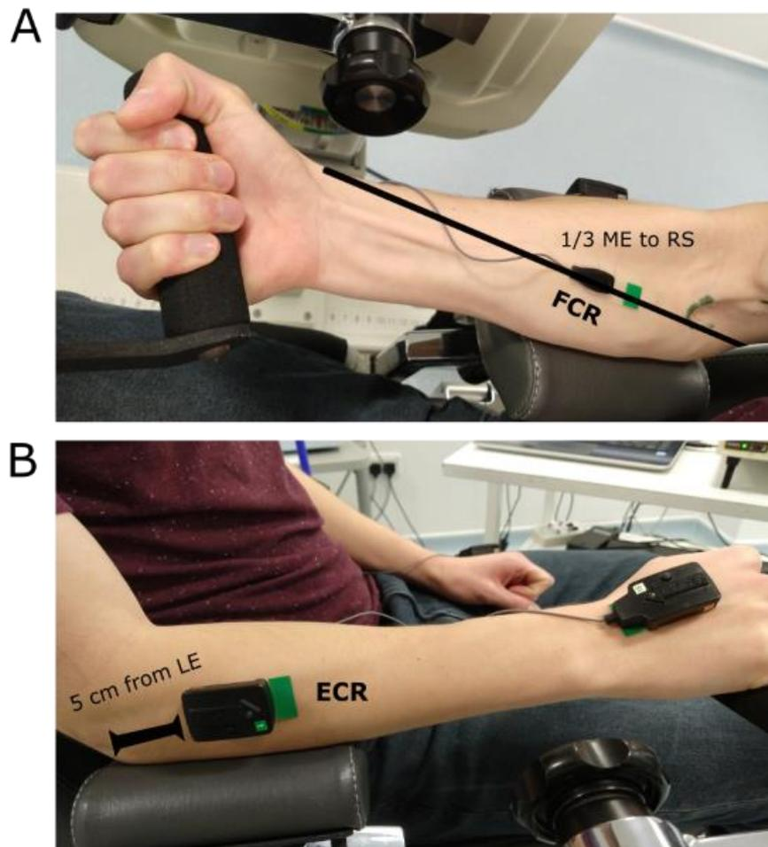
**Figure 3.2.** EMG sensor positioning. Sensor positioning to record activity from the FCR muscle (A) and ECR muscle (B). ME = medial epicondyle; RS = radial styloid; LE = lateral epicondyle.
