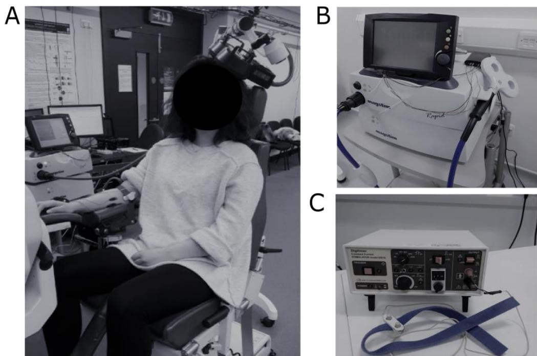
**Figure 3.1.** Setting and instrumentation. (A) Position of the participant while sitting on the dynamometer. (B) Magstim Rapid stimulator used for delivering TMS and (C) Digitimer DS7A used for delivering median nerve stimulation.
