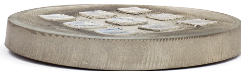
Figure 4.2: Image of a substrate following EBM of tungsten powder directly onto the surface.
