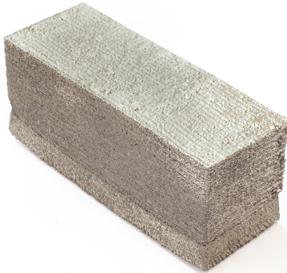
Figure 5.8: Photograph of manufactured cuboid used for 3-point bend tests
