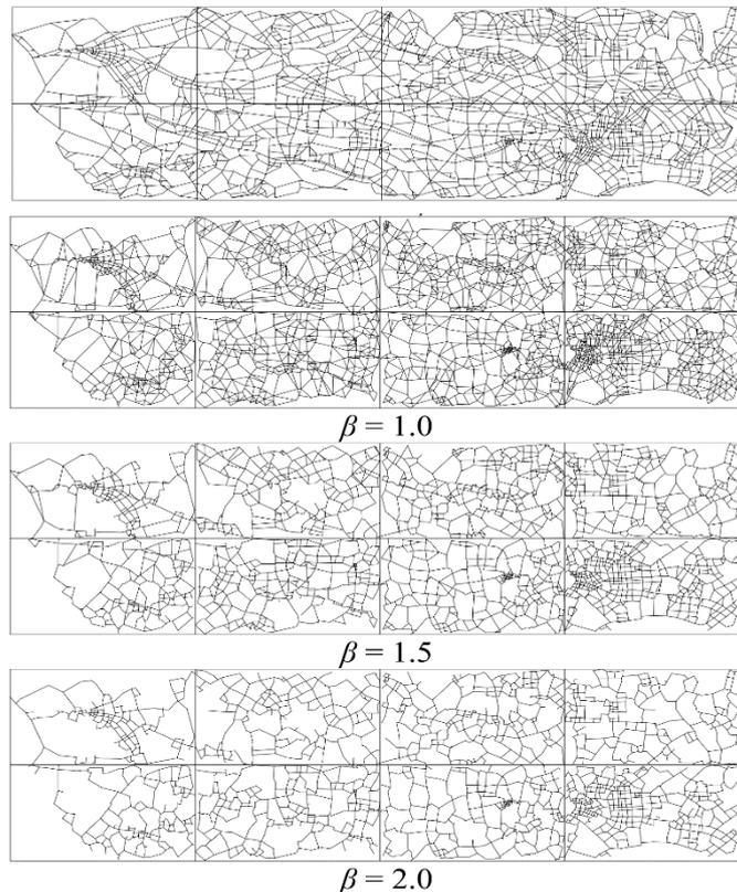
**Figure 4.6  $\beta$ -skeleton networks:** The four panels compare the Tokyo road network (top) and constructed  $\beta$ -skeleton networks on the spatial distribution of Tokyo road network nodes with  $\beta = 1.0, 1.5,$  and  $2.0$ . (Osaragi and Hiraga, 2014)
