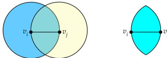
**Figure 4.4 Relative Neighbourhood Graph:** The two plots illustrate the definition of RNG neighbourhood of nodes  $v_i$  and  $v_j$ .  $v_i$  and  $v_j$  are RNG neighbours, if the lune (right) of two circles drawn with radius equals the distance  $d_{ij}$  between  $v_i$  and  $v_j$  respectively (left), is empty. (Toussaint, 2014)
