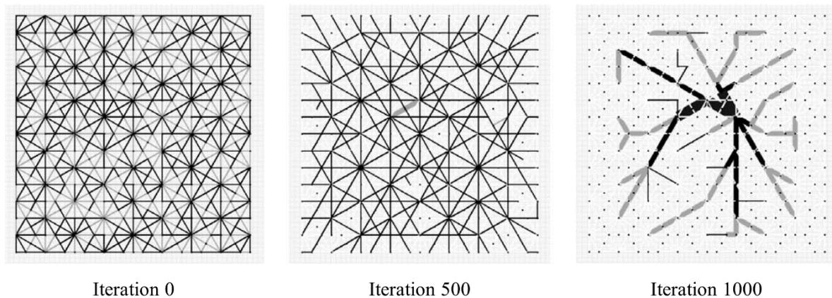
**Figure 4.13 Transport Demand Modelling and Network Evolution:** The three plots show the evolution process of a simulated road network from an initial condition of an asymmetric hexagon to a hub-and-spoke network (Xie and Levinson, 2009).
