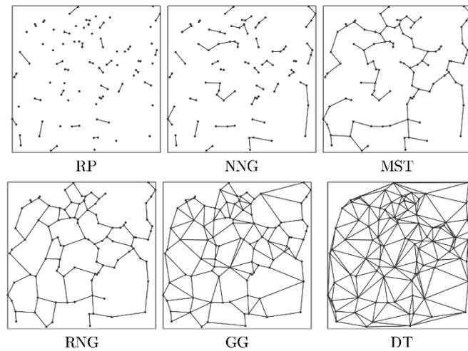
**Figure 4.5 Proximity Graphs:** The two panels include members of the proximity graphs family - Reciprocal pairs (RP), Nearest Neighbourhood Graph (NNG), RNG, Minimal Spanning Tree (MST), Gabriel Graph (GG), and Delaunay Triangulation (DT);  $RP \subseteq NNG \subseteq MST \subseteq RNG \subseteq GG \subseteq DT$ . (Watanabe, 2008)
