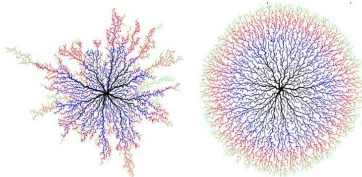
**Figure 4.16 Fractal Urban and Transport Network Evolution:** These two plots show simulated distribution networks by minimising the cost of link length (left) and maximising efficiency (right), both having dendritic structure. (Gastner and Newman, 2006a)
