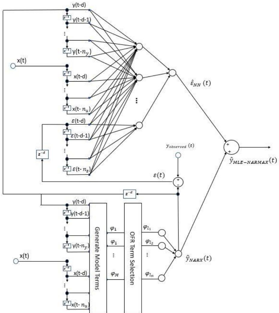
**Figure 5.2.** The MLE-NARMAX model structure
