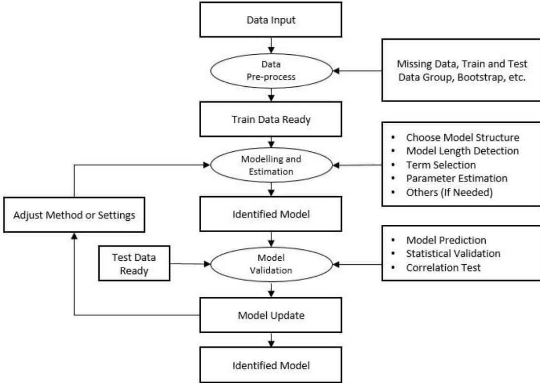
**Figure 2.1** The general procedure of system identification
