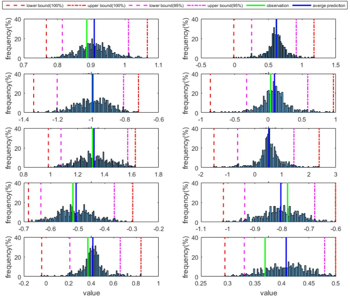
**Figure 4.6** Prediction of Cloud-NARX model on 10 randomly selected test data points
