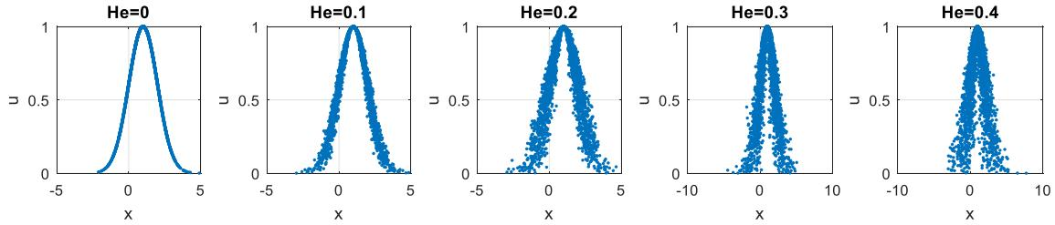
**Figure 4.1** The cloud membership functions of cloud models with different values of  $he$  ( $ex = 1$ ,  $en = 1$ )
