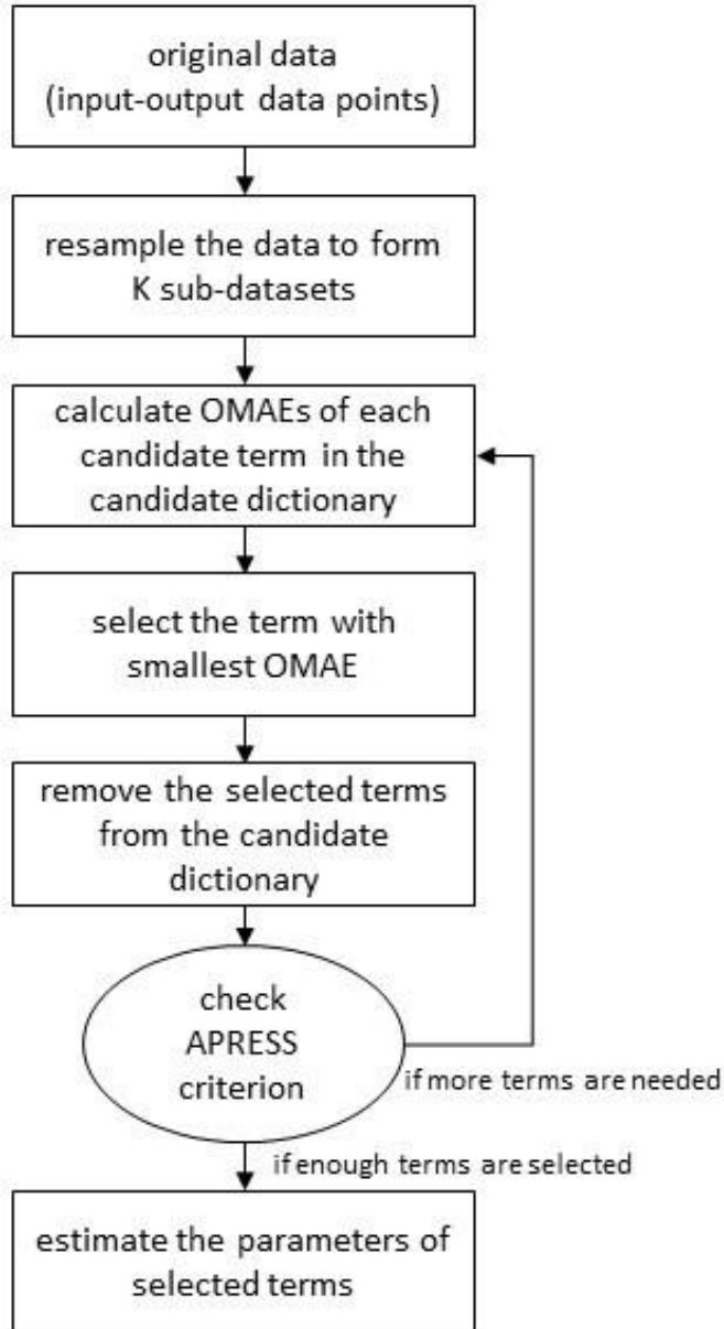
**Figure 3.1** Robust model structure selection (RMSS) method
