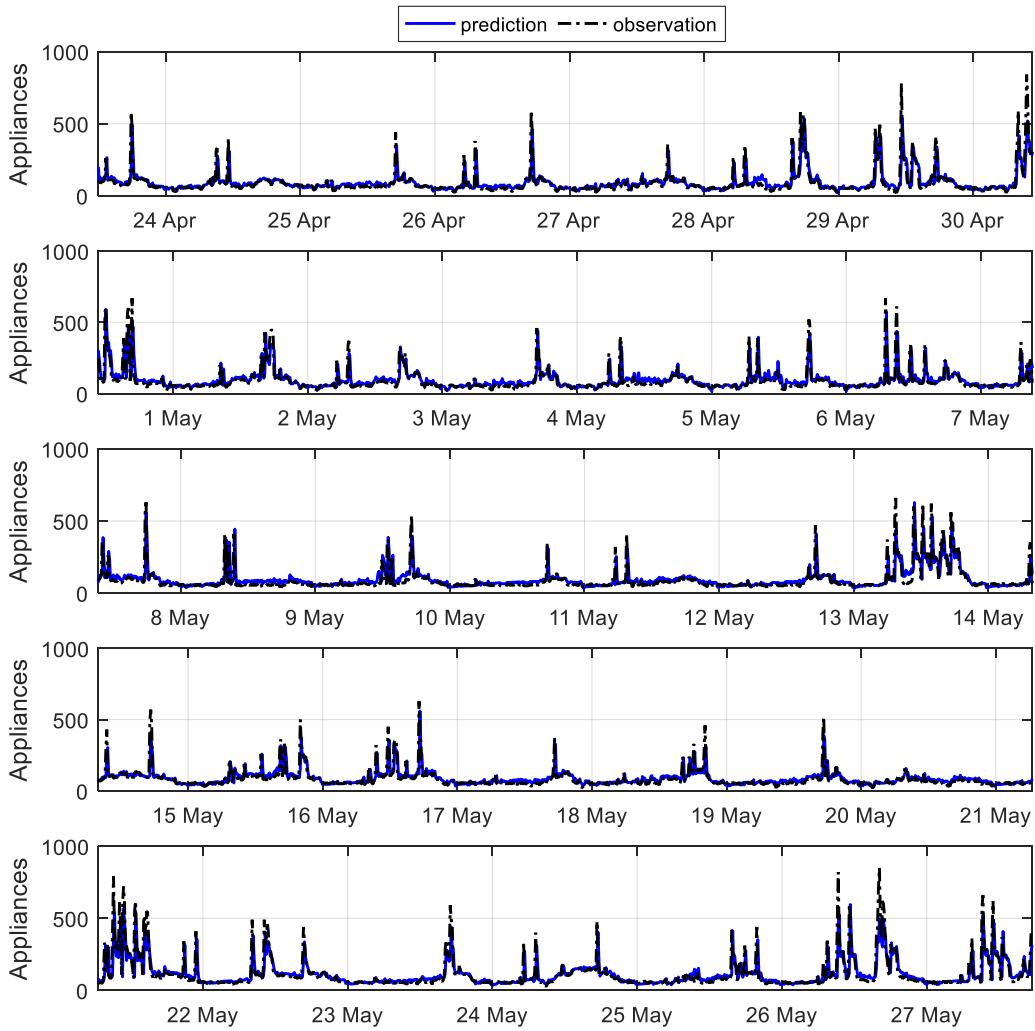
**Figure 5.12** Comparison of observed and predicated appliances energy use of MLE-NARMAX model
