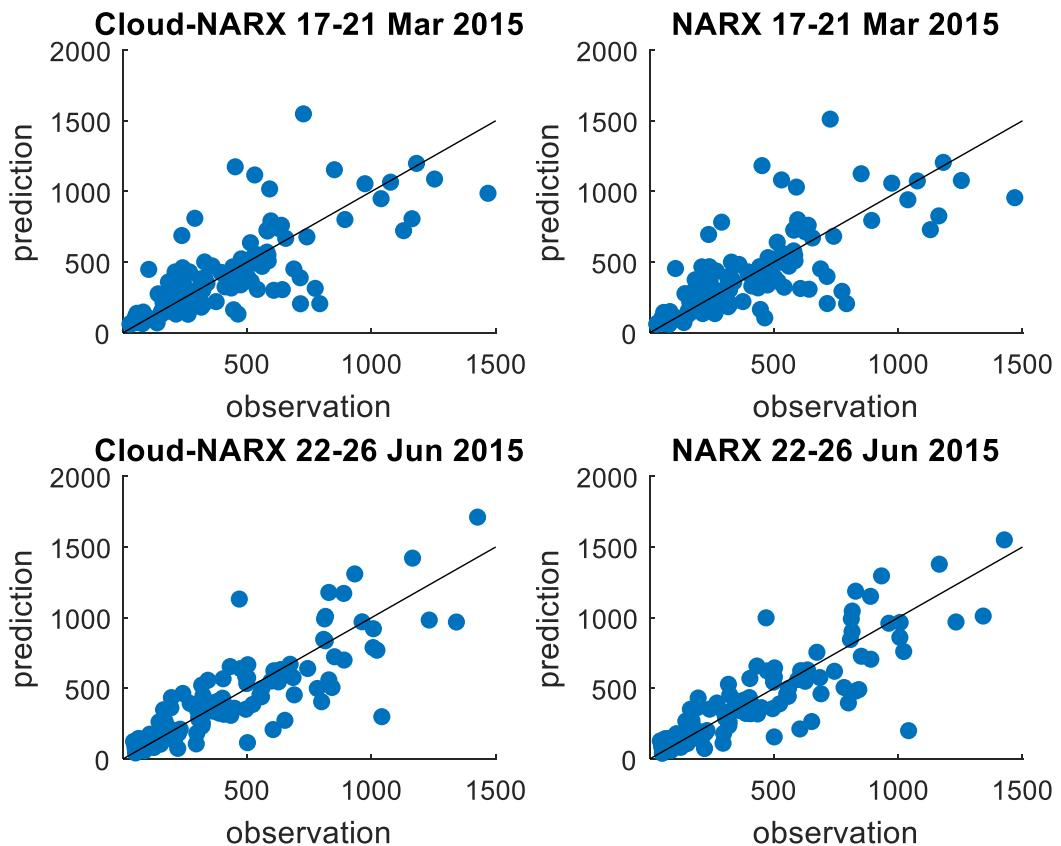
**Figure 4.12** Scatter plot of the averaged prediction and observation of the cloud-NARX model and the best NARX model on two test datasets
