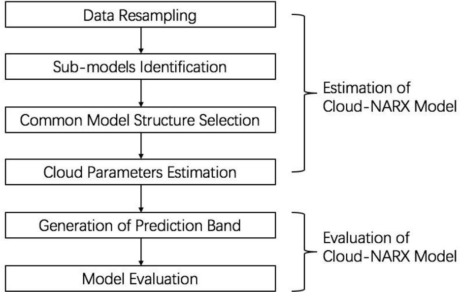
**Figure 4.2** The process of estimation and evaluation of the cloud-NARX model
