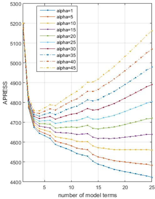
**Figure 5.10** Number of selected model terms versus APRESS value (alpha is a tuning parameter)
