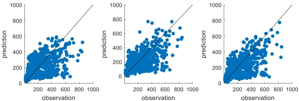
**Figure 5.11** Scatter plot of observed and predicted appliance energy use (left: First-stage NARX model, middle: Neural Network, right: MLE-NARMAX Model)
