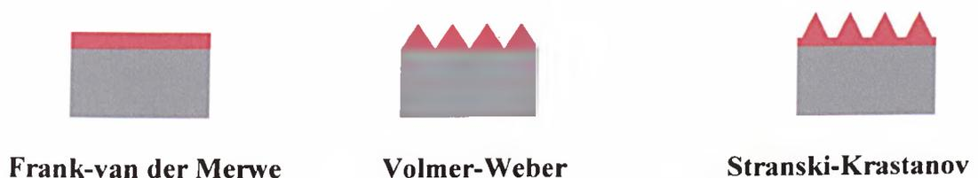
Figure 5-1 Schematic diagrams of the three possible growth modes.
